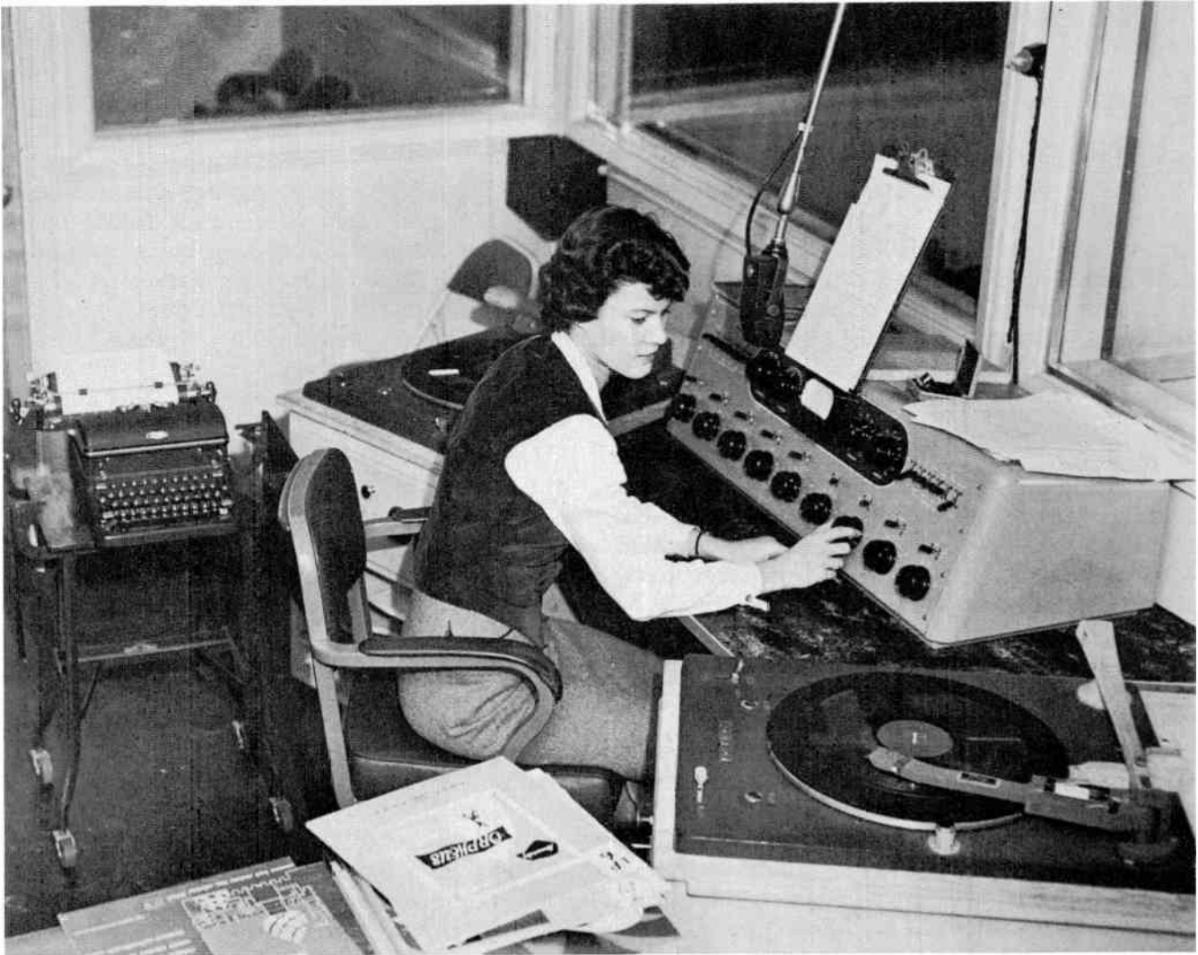
Figure 2. If you are fortunate enough to have studios and a control room, we suggest the above arrangement for the master control booth. It is practical and easy for one person to handle. Note the typewriter for keeping the log; the playback tables on both sides of the console; the overhang mike; the day's copy and schedule on the clip board. The table in the foreground is used for a tape recorder when one is necessary for production or playback. Playback tables are equipped for both 33 1/3 r.p.m. and 78 r.p.m. in addition to LP. Change on the playback head is made by a twist of the wrist. (Photo courtesy WBUR-FM, Boston University)
