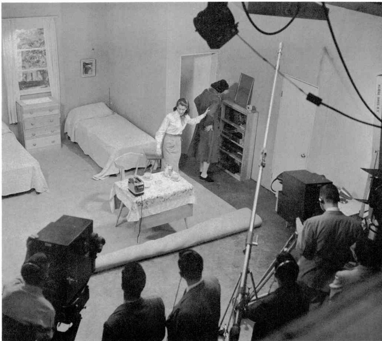
Figure 5. General view of a college television workshop in action. Note students manning cameras in foreground; boom mike to pick up dialogue; lighting system and set. After television play has been rehearsed, motion pictures are taken by mounting movie cameras on the cameras. (Photo courtesy Boston University Television)
