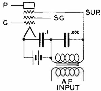
3—(38) Draw a simple schematic diagram showing a method of coupling a modulator tube to a radio frequency power amplifier tube to produce grid modulation of the amplified radio frequency energy.
