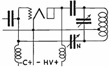
2—(102) Draw a simple schematic circuit diagram of a radio frequency amplifier, employing a triode vacuum tube and making use of grid neutralization.
