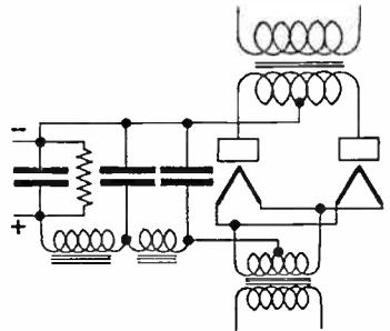
2—(247) Draw a diagram of a half wave rectifier system employing thermionic rectifier tubes and a two section, condenser input, filter system.
