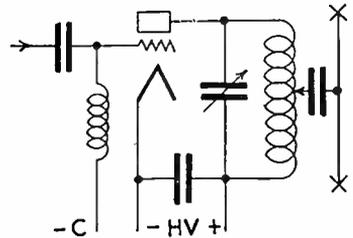
3—(78) Draw a simple schematic diagram indicating a capacitive coupling system between a tuned grid-tuned plate oscillator stage and a single electron tube, neutralized amplifier.
