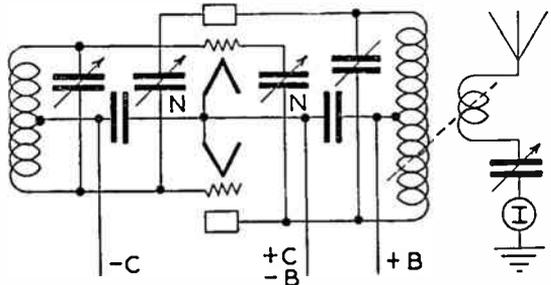
3—(80) Draw a simple schematic diagram of a system of neutralizing the grid-plate capacitance of a single electron tube employed as a radio-frequency amplifier.
