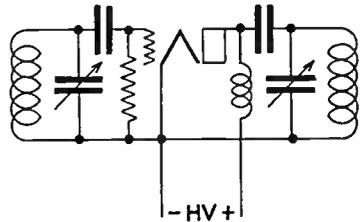
2—(90) Draw a simple schematic diagram of a crystal controlled vacuum tube oscillator. Indicate power supply polarity.
