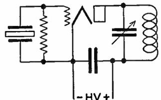
2—(91) Draw a simple schematic diagram showing a Colpitts type triode oscillator, with shunt-fed plate. Indicate power supply polarity.
