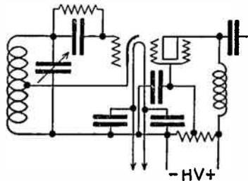
2—(94) Draw a simple schematic diagram of a pentode type tube used as a crystal controlled oscillator, indicating power supply polarities.
