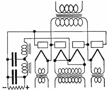
2—(246) Draw a diagram of a full wave, single phase, rectifier employing thermionic vacuum tubes, connected to a condenser input, two section filter system, and including a bleeder resistance.
