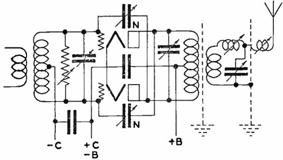
4-(109) Draw a complete class B modulation system, including the modulated radio frequency amplifier stage. Indicate points where the various voltages will be connected.
