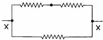
2—(112) Draw a simple schematic diagram showing the method of connecting three resistors of equal value so that the total resistance will be one and one-half times the resistance of one unit.
