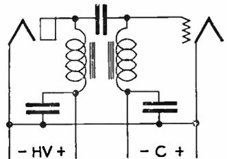
2—(100) Draw a diagram of a method of coupling a single radio frequency amplifier using a triode vacuum tube to a push pull radio frequency amplifier using triode vacuum tubes, showing proper neutralization of the push pull amplifier.
