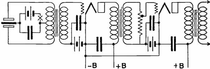
3—(36) Draw a simple schematic diagram showing a Heising modulation system capable of producing 100-percent modulation. Indicate power-supply polarity where necessary.
