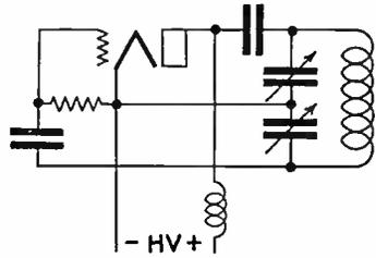
2—(92) Draw a simple schematic diagram showing a tuned-grid Armstrong type triode oscillator, with series-fed plate. Indicate power supply polarity.
