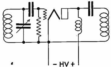
2—(89) Draw a simple schematic diagram showing a tuned-plate tuned-grid triode oscillator with shunt-fed plate. Indicate polarity of supply voltages.
