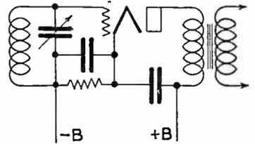
2—(108) Draw a simple schematic diagram of a triode vacuum tube connected for grid-leak condenser detection.
