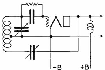
2—(110) Draw a simple schematic circuit of a radio frequency doubler stage, indicating any pertinent points which will distinguish this circuit as that of a frequency doubler.
