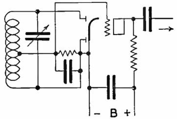
2—(107) Draw a simple schematic diagram of a triode vacuum tube connected for plate or "power" detection.
