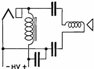
2—(96) Draw a simple schematic diagram of a triode vacuum tube audio frequency amplifier inductively coupled to a loudspeaker.
