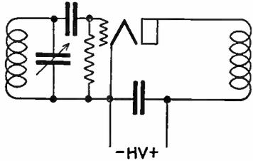
2—(93) Draw a simple schematic diagram of an electron coupled oscillator, indicating power supply polarities where necessary.
