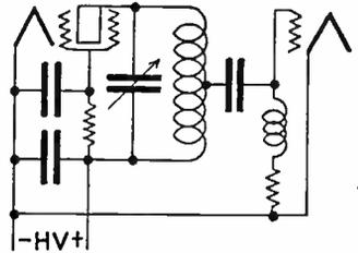
2—(105) Draw a simple schematic diagram showing a method of coupling between two triode vacuum tubes in a tuned radio frequency amplifier, and a method of neutralizing to prevent oscillation.
