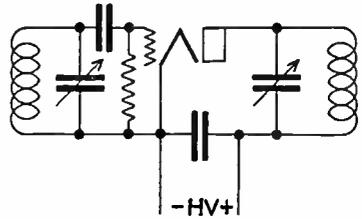
2—(87) Draw a simple schematic diagram showing a Hartley triode oscillator with shunt-fed plate. Indicate power supply polarity.
