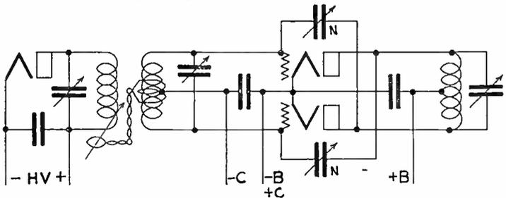
2—(101) Draw a simple schematic circuit diagram of a radio frequency amplifier, employing a triode vacuum tube and making use of plate neutralization.
