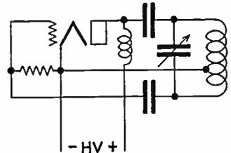
2—(88) Draw a simple schematic diagram showing a tuned-grid Armstrong type triode oscillator, with shunt-fed plate. Indicate power supply polarity.
