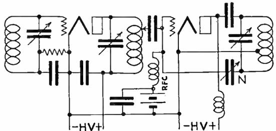
3—(79) Draw a simple schematic diagram of a push-pull, neutralized radio frequency amplifier stage, coupled to a Marconi type antenna system.
