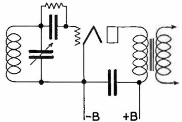
2—(109) Draw a simple schematic circuit of a regenerative detector.
