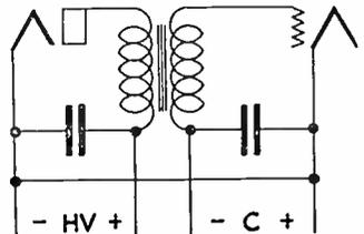
2—(99) Draw a simple schematic diagram of a method of impedance coupling between two vacuum tubes in an audio frequency amplifier.
