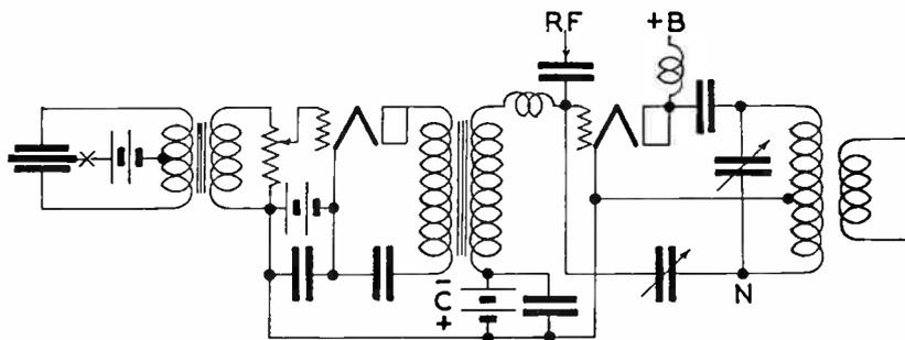
4—(55) Draw a simple schematic diagram of a class B audio high level modulation system, including the modulated radio frequency stage.
