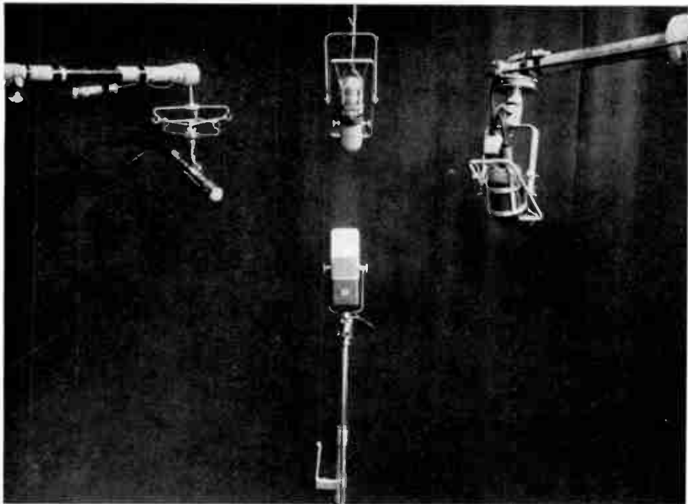
Broadcast microphones: Clockwise from left: Electro-Voice dynamic 666; RCA 77 D; Altec cardioid 639 B; RCA velocity 44 BX.
