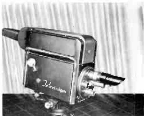
RCA TK-11 image orthicon camera with 3-inch tube and lens turret
