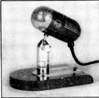
FIG. 30. RCA pressure microphone, type 88-A (MI-4048C). This microphone is ideal for general remote pickup use. It has good frequency response and is relatively free from effects of wind and moisture. Its rugged construction withstands the hard usage of remote work.
