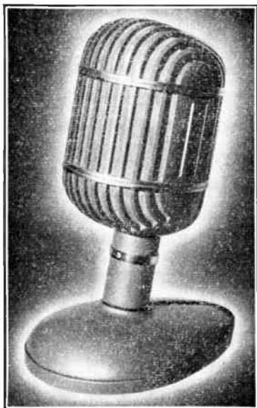
FIG. 24. Western Electric 639B cardioid microphone, on desk-type base. Combines a dynamic moving-coil pressure element with an improved ribbon-type velocity element.
