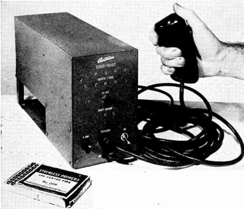
FIGURE 21. Aeronics's Sono-shot, an instrument that simulates live gunshots by electronically firing shotgun primers. (Courtesy of Aeronics, Inc., of New York.)
