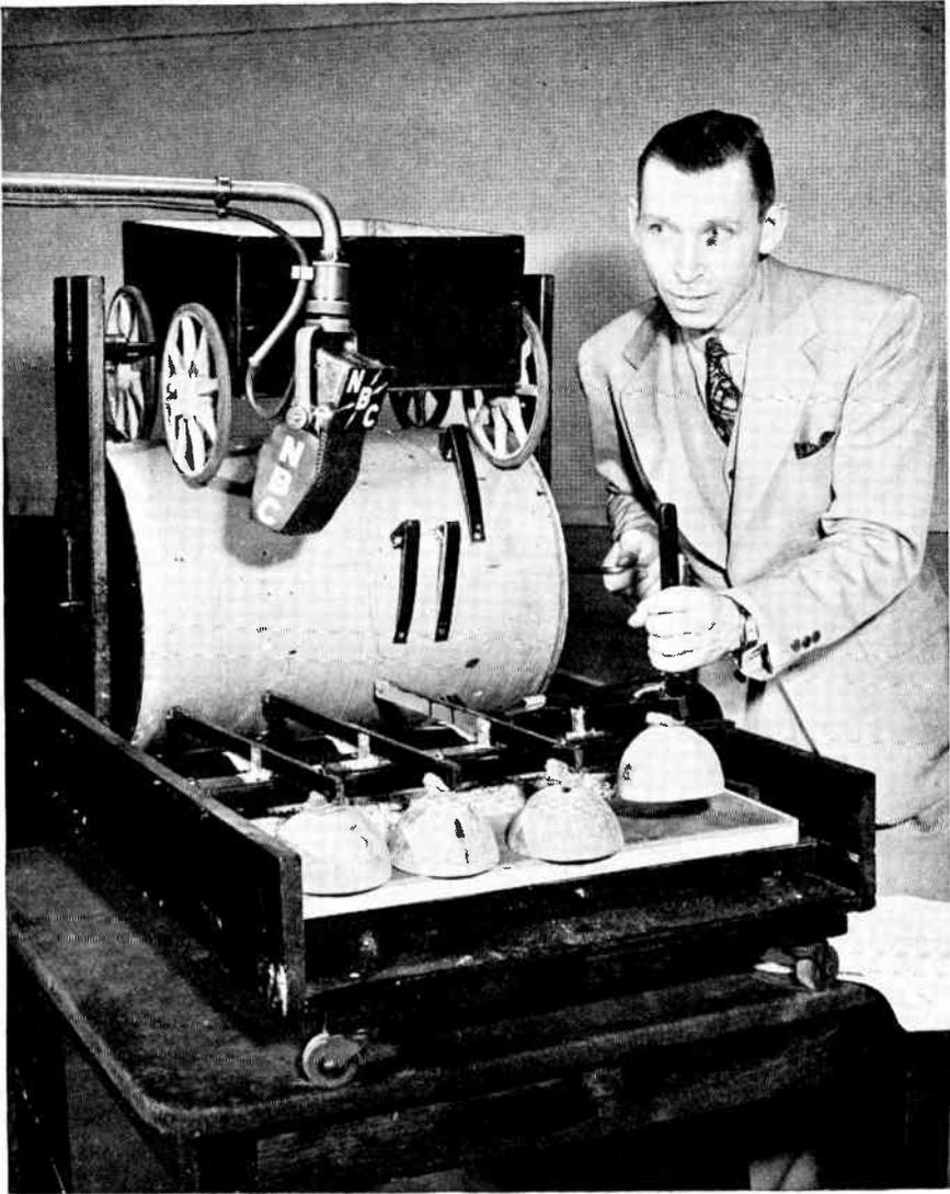
FIGURE 9. Soundman Tommy Evans operating NBC's horse and wagon apparatus. The eccentric offsets on the revolving drum activate the hooves in proper rhythm. Surfaces under the hooves are interchangeable to simulate different terrain. (Courtesy of National Broadcasting Company.)
