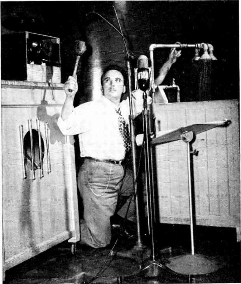
FIGURE 19. Soundman Edward Wojtal striking a thunder spring. The spring is attached to a contact mike and fed to a speaker. At the upper left is a wind machine and on the right a rain machine. (Courtesy of Columbia Broadcasting System.)
