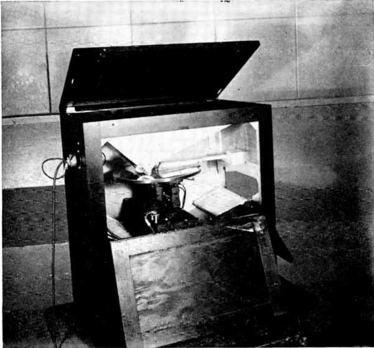
FIGURE 49. *Later refinement of rain machine as shown in Figure 47. Birdseed from hopper dropped on revolving turntable. Stationary arm swept off birdseed onto cellophane panels as the table revolved. (Courtesy of Columbia Broadcasting System.)*
