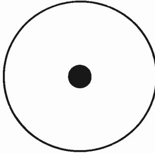
The small circle indicates the nondirectional mike. The large circle indicates the pickup pattern. Any sound given on the periphery of the large circle will have the same volume and frequency response, no matter from what direction it comes. In other words, the pickup is not limited to any specific direction; the beam is 360 degrees; there is no dead side. If used for sound, a nondirectional mike should be mounted so that the axis of the beam is parallel to the floor.
