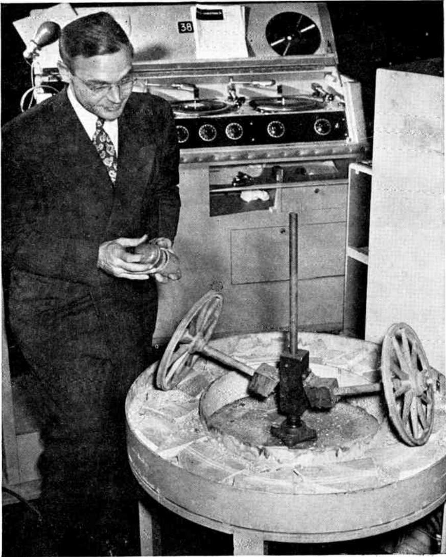
FIGURE 1. Carriage on cobblestone street used on *Sherlock Holmes*. The motor revolving the wheels is controlled by a foot-operated variac. Soundman Bill Hoffman uses hollowed wooden blocks for horse's hooves. (Courtesy of Mutual Broadcasting System.)
