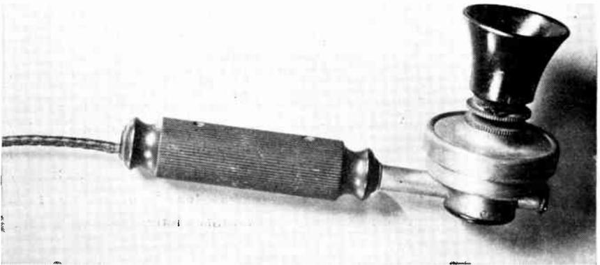
FIGURE 18. *One of the first devices used to get a realistic “filtered” telephone effect. The actor spoke into the hand-held phone instead of speaking into a filtered cast mike. (Courtesy of National Broadcasting Company.)*
