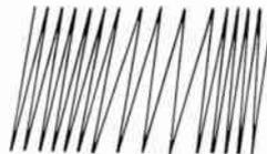
This would be the modulated carrier wave. The frequency is increased where the sound wave is highest (positive) and the frequency is decreased where the sound wave is lowest (negative). The amplitude does not change.
