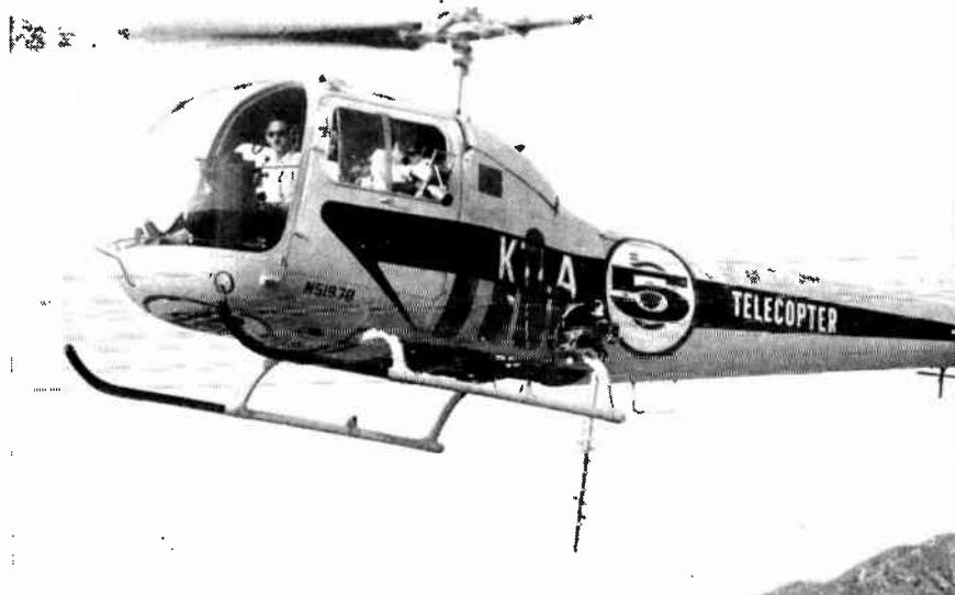
Fig. 20-20. KTLA Telecopter over Los Angeles. GE vidicon camera with Pan Cinor zoom lens and open frame view finder protrudes from cockpit window. Transmitter antenna, below, must be raised before landing.
