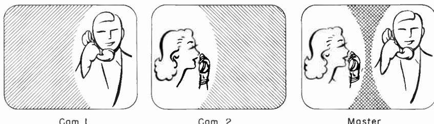
Fig. 12-9. Matting by off-setting the lens turret. The two cameras are superimposed for the composite effect shown at right as it is seen on the master monitor.
