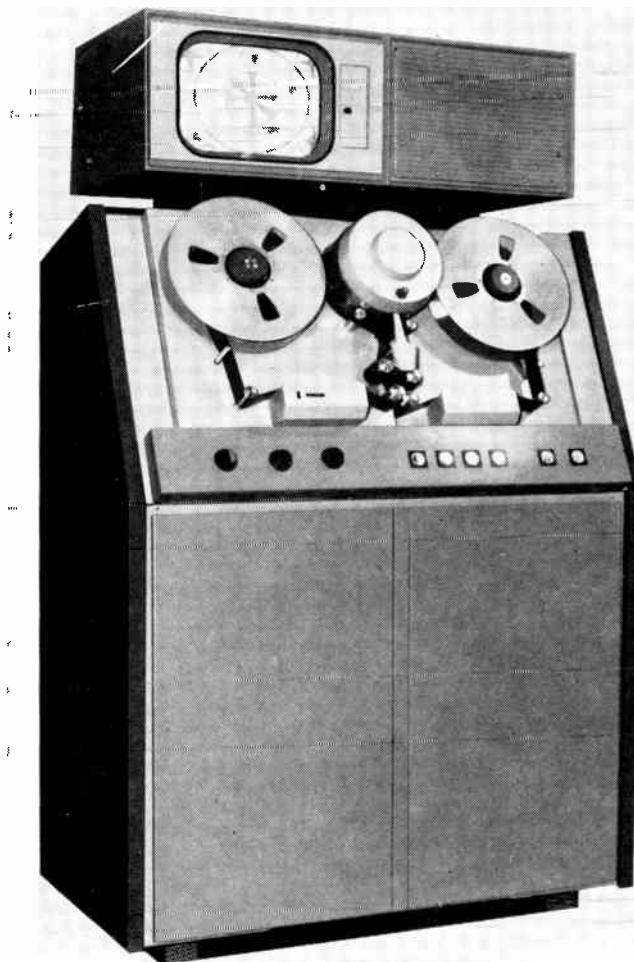
Fig. 23-9. The Ampex VR 8000. The single head rotates inside the drum at center as the tape moves around it in a helical wind.
