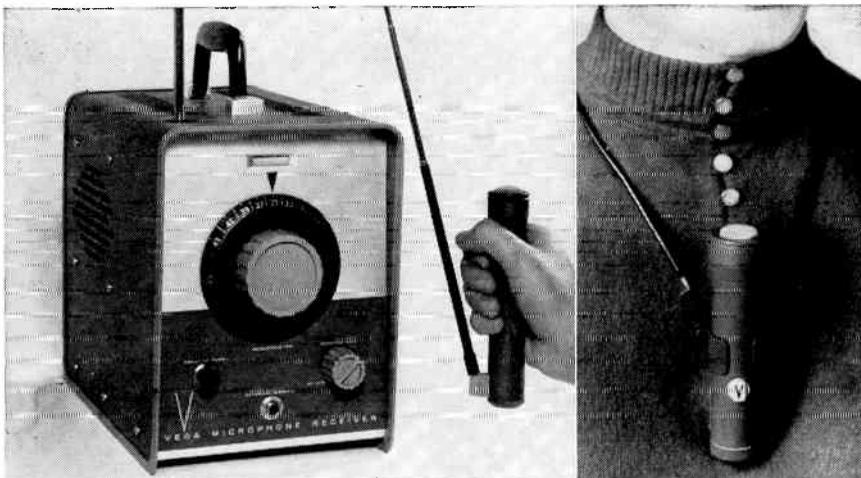
Fig. 19-15. Vega wireless microphone. Receiving unit on left. Mike may be used in the hand with telescoping antenna or may be worn as a lavaliere, in which case the neck strap acts as an antenna element. Several Vega microphones may be used with one receiving unit, either on the same frequency (in which case they all operate together without individual adjustment) or on different frequencies (in which case they can only be used separately, since the receiving unit must be retuned between them).
