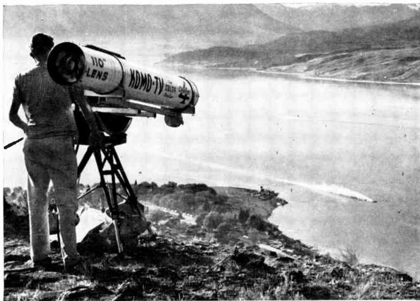
Fig. 5-7. A 110-inch lens at KOMO-TV, Seattle. Horizontal angle of view: 0.6 degrees. This is sufficient to fill the entire camera field with a close-up of the sun or moon. Here the lens is shown following hydroplane races on Lake Chelan.
