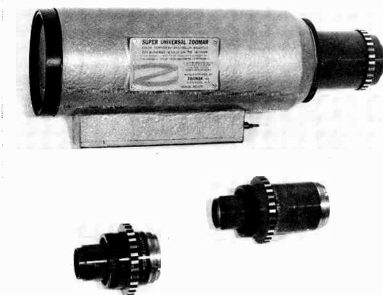
Fig. 5-12. Super Universal Zoomar with converters. Focal length of lens as shown above: 2 1/2 to 16 inches ( $f/3.9$ ). With converter at lower left: 4 to 25 inches ( $f/5.6$ ). With converter at lower right: 6 1/2 to 40 inches ( $f/8$ ).
