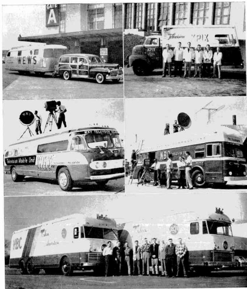
Fig. 20-15. Six representative mobile units. Top left, WEWS, Cleveland, adapted Sparton House trailer. Top right, KPIX, San Francisco, adapted Ford truck. Center left, WKY-TV, Oklahoma City, adapted Flexible bus. Center right, NBC "crash" unit includes audio and video transmitters and gas-driven generator. Bottom, NBC, Hollywood, color TV mobile vans.
