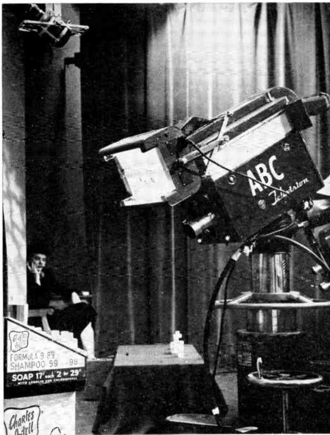
Fig. 22-5. TelePrompTer in action on a live commercial.
