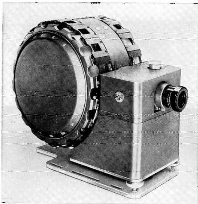
Fig. 10-8. RCA TP7 slide projector, a dual 2- by 2-inch slide projector utilizing one light source and one projection lens. Magazines hold total of 36 slides.
