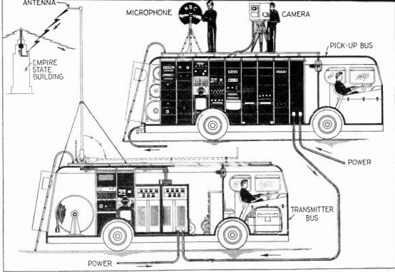
$F_{IG}$ . 44.—The television mobile unit. The upper unit is equivalent to a studio control room; the lower unit contains the radio transmitter used to relay the television signal to the Empire State Building for rebroadcast on the main transmitter.
