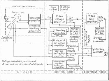
FIG. 67.—A typical one-channel television system.
