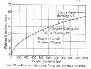
the service radius of the station) in terms of the height of the antenna. This has been done in the following table:
