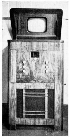
FIG. 9a.—A model of receiver used during the field-test period of the development of the RCA-NBC television system.
