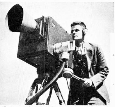
FIG. 48.—An outdoor-type television camera mounted on a motion-picturetype tripod. The funnel-shaped hood on the front is to shield the lens from stray light.
