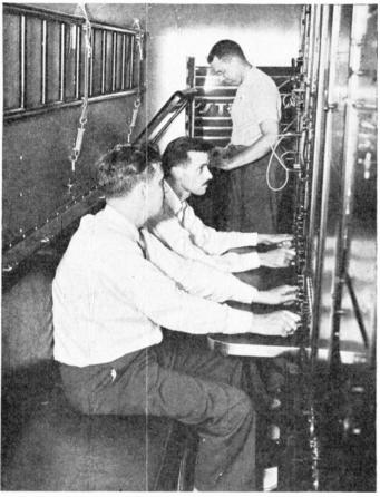
FIG. 50.—Another view of the control position, showing the audio and video engineers at work. In the rear, an engineer is monitoring the picture on a home-type receiver.
