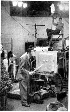
FIG. 26.—A "dolly" television camera. This camera is used for "moving shots"—such as moving in from a "long shot" of a person to a head-and-shoulders close-up. The camera operator can ride along with the camera, concentrating all his attention on the composition and focus of the picture, while being pushed by a second person.
