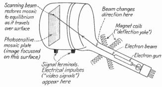
FIG. 5.-The essential parts of an Iconoscope.
