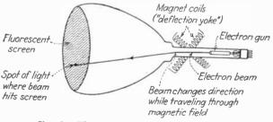
FIG. 8.-The principal parts of a Kinescope.
