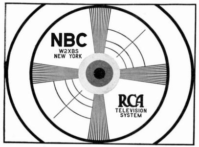
FIG. 68a.-The NBC-RCA standard test chart.
