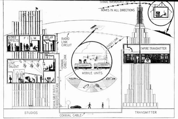
FIG. 20.—The three sources of program origination; live talent, film, and outside pickups; and the methods used to relay the television signal to the main transmitter at the Empire State tower for rebroadcast to viewers in the New York area.
