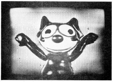
FIG. 3b.—In the modern picture the tiny dots visible are on the acoustic wall material, in the studio. They further indicate the definition possible with 441-line scanning.
