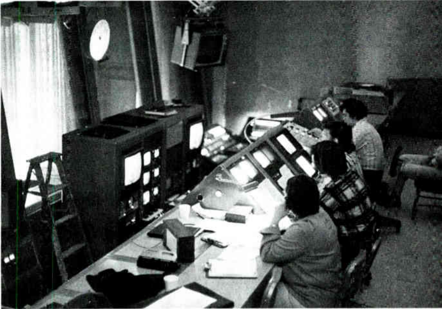
1-2 The actual coordination of production persons and equipment takes place in the control room. Here decisions are made about what kinds of pictures and sounds are to be stored on videotape or sent directly over the air.
