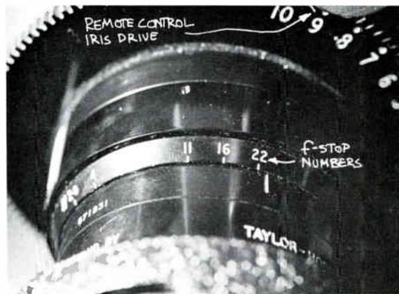
3-6 f -Stop: The f -stop is a calibration that indicates how large or small the iris, or lens opening, is.
