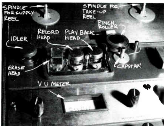
7-30 Head Assembly of the Reel-to-Reel Tape Recorder.
