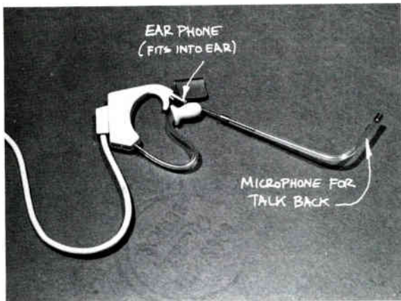
8-2 Intercom Headset: The most vital link in television production is the intercommunication system. All production and engineering personnel that need
