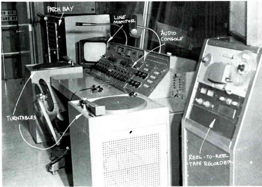
8-9 Audio Control: The audio control area contains the audio control board, through which the various sound inputs are selected, amplified, mixed, and distributed to the line-out, reel-to-reel tape machines, or at least the controls for them, tape cartridge machines, turntables, speakers and intercom controls, and patching facilities. In essence, the audio control area in the television control room represents a small radio station.
