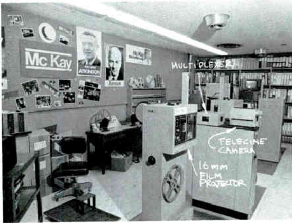
8-13 Telecine Room: Telecine contains the film islands, consisting of film projectors, slide projectors, multiplexers, and television film, or telecine, cameras
