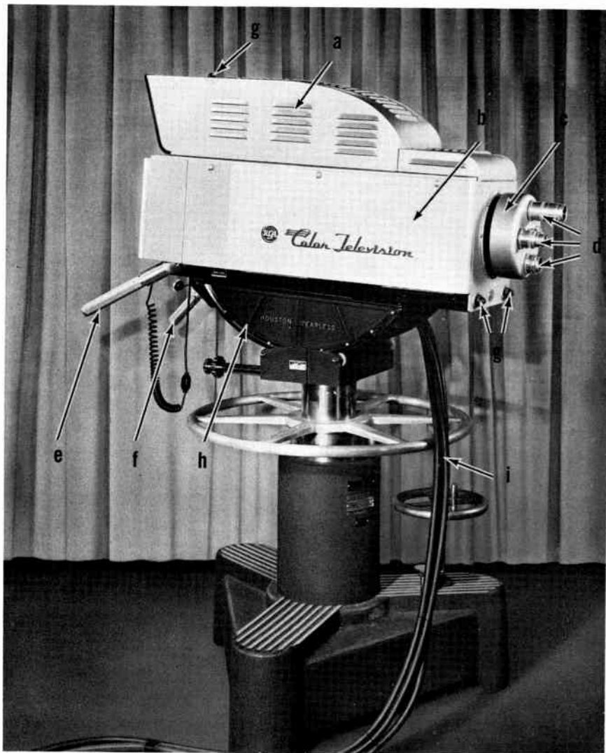
RCA TK-41 Color Camera: a) viewfinder; b) camera; c) lens turret; d) lenses; e) camera panning handle with focus grip; f) camera panning handle; g) tally lights; h) cradle head; i) three camera cables.
