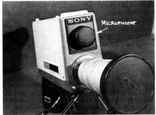
17-11 Most portapak cameras have an omnidirectional microphone attached or built in, pointing into the direction of the lens.
