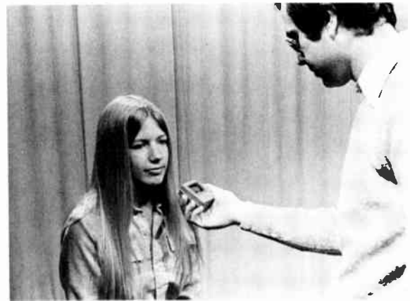
b Reflected Light Reading: Light meter is pointed close to the lighted object, thereby measuring the light reflected by the object.
