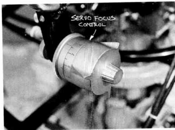
3-29 Servo Focus Control: The servo focus control does not transfer your movement of the focus wheel mechanically; instead, it activates a motor that drives the focus mechanism in the zoom lens extremely smoothly.
