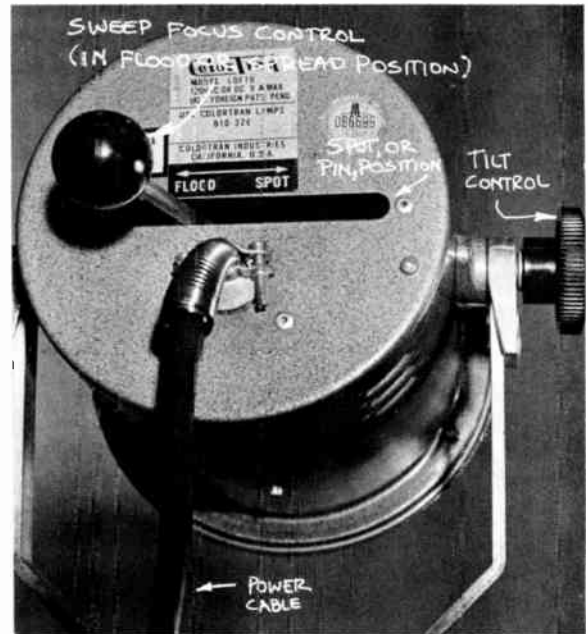
5-9 Sweep Focus: The beam can be spread or pinned by moving the sweep knob horizontally to flood (spreading) or spot (pinning) position.
