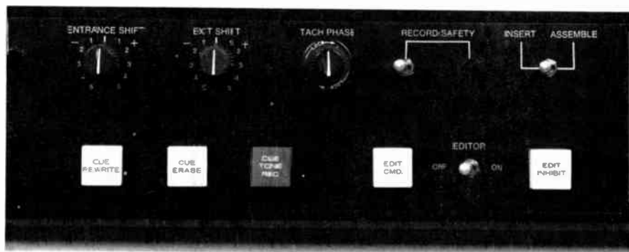
10-28 Ampex AVR-2 Editec Electronic Editor.
