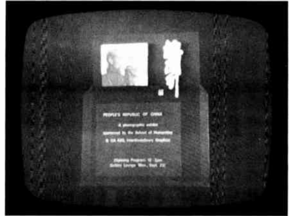
12-3 When showing an out-of-aspect-ratio studio card in its entirety, the information usually becomes so small that it is no longer readable.
