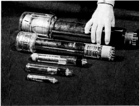
2-6 Television Pickup Tubes (from top to bottom): 4½-inch image orthicon; 3-inch image orthicon; 25mm Plumbicon; 1-inch vidicon; ⅔-inch vidicon.
