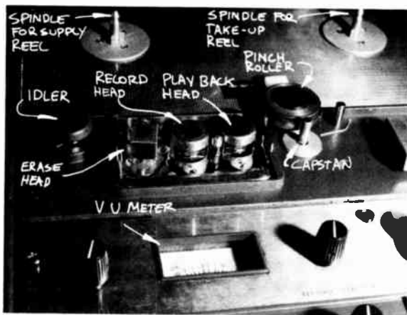
7-30 Head Assembly of the Reel-to-Reel Tape Recorder.
