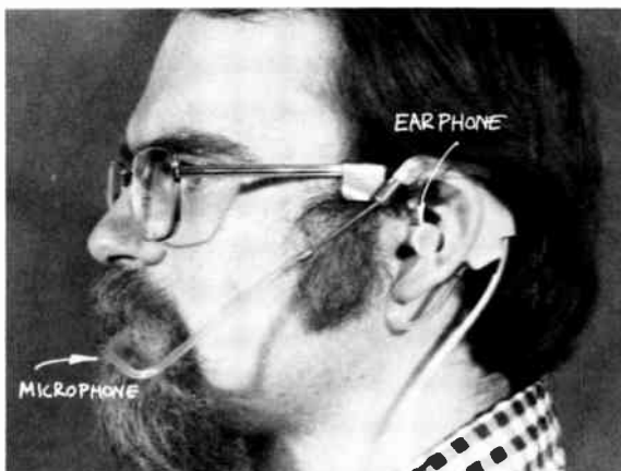
to be in voice contact wear telephone headsets with a small earphone and a microphone for talkback.
