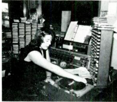
Figure 12.2 Janet Wooldridge cues-up a record on turntable 2, while turntable 1 plays the music being broadcast. (Courtesy KTOB-AM, Petaluma, California)
