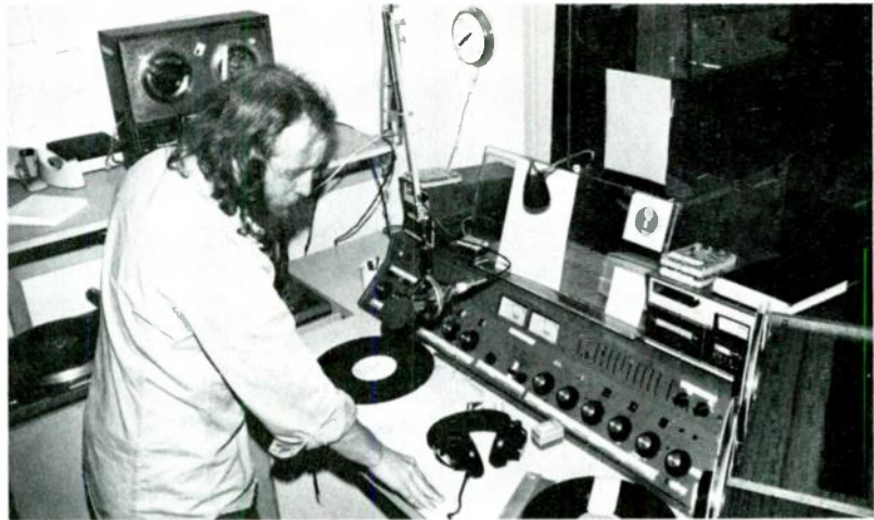
Figure 10.1 David T., production director for KTIM, San Rafael, California, produces a recorded commercial for a local account. He works with a Gates console and turntables, an E-V 635A microphone, Sony and Otari tape recorders, and Sparta cart machines. Having written a rough script, he lays down a “bed” of music and sound effects on the Sony recorder, and then mixes its output and his voice (through the mic) onto the Otari recorder. The last step sees him transfer the completed spot to a cart, which then is labeled for identification purposes. (Courtesy KTIM, San Rafael, California)
