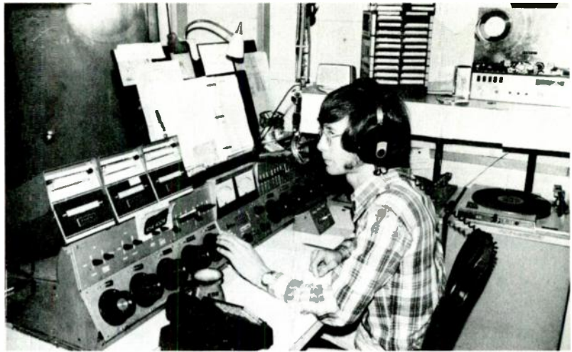
Figure 12.4 Clint Weyrauch, program director and air “personality” for KTIM, San Rafael, is shown during his regular air shift. He works a Gates stereo board, two Sparta turntables, and Sparta cart machines, and he speaks into an Electro-Voice 635A microphone. Before him are the running log (on counter top), and the copy or continuity book. (Courtesy KTIM, San Rafael, California)
