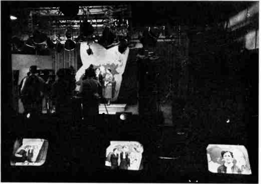
Control room monitors indicate area of pick-up by different lenses from studio cameras each 17 feet from scene: 50 mm., 90 mm., and 8½ inch.
