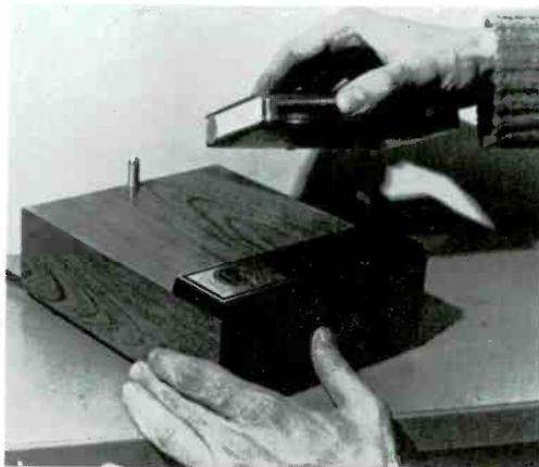
**FIGURE 9.14** Cartridge tape builder. Rather than do this themselves, the majority of stations simply purchase new carts or send existing ones out to be refilled. Courtesy Broadcast Electronics.
