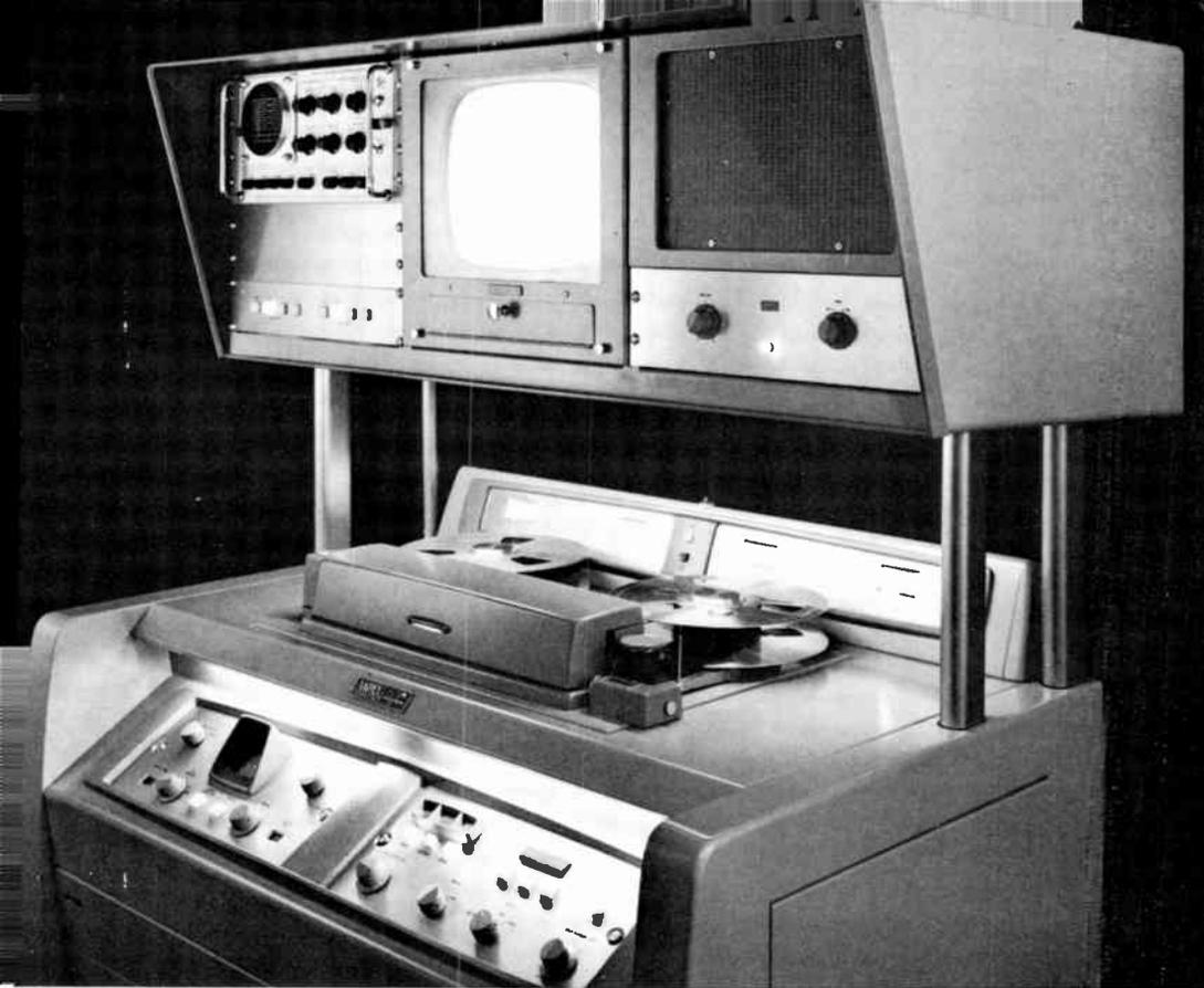
Figure 59. Videotape, Ampex VR-1000 Magnetic Recorder.
