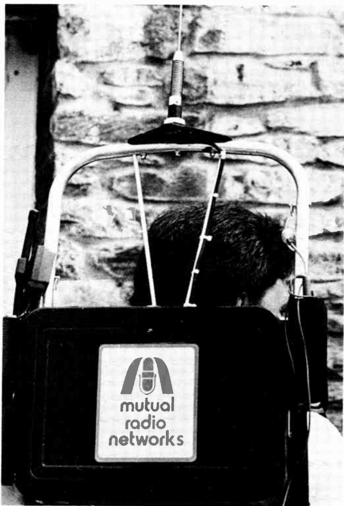
Fig. 1-4. An example of today's high-technology broadcasting equipment: Mutual Broadcasting System's exclusive long-distance wireless reporting back-pack for location and remote broadcasts. ( Courtesy Mutual Broadcasting System )
