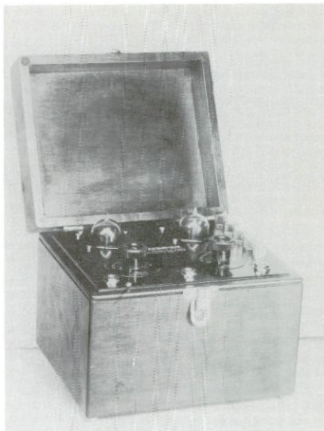
Radiola Senior Amplifier, a two tube amplifier made for RCA by Westinghouse, was designed to be used in conjunction with company's one tube receivers. Circa 1923 Courtesy RCA.
