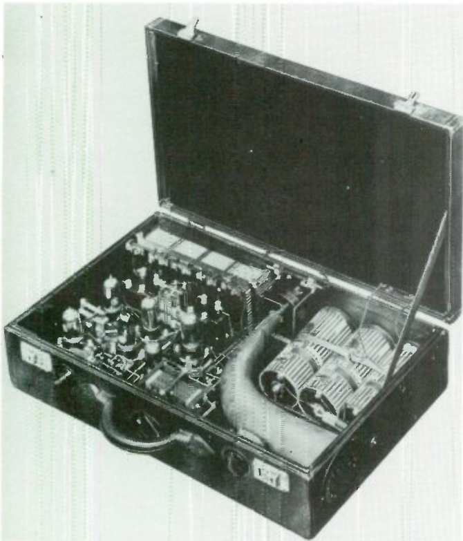
Inside the first Zenith portable receiver; six tubes and a single tuned stage. Everything else appears to be audio amplification. Courtesy Zenith
