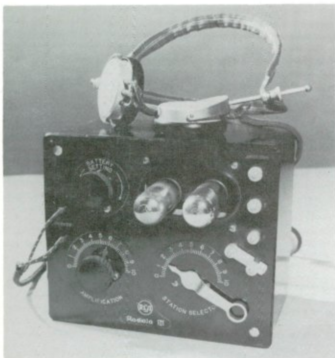
RCA Radiola III. Made in 1923, this two tube regenerative receiver has a bakelite panel that carries all the controls. The "Battery Setting" varies filament voltage. "Amplification" controls regeneration. Courtesy RCA.
