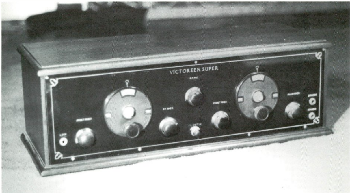
Victoreen Super receiver, using an advanced superhet circuit and sold in kit form, 1928 to 1929. It had eight tubes and a tunable second detector. Jacob collection.
