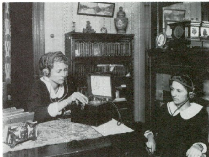
First mass-produced receiver. Made for RCA by Westinghouse, it is called Aeriola Jr. and uses a lead galena crystal and a single tunable circuit. Courtesy Westinghouse.
