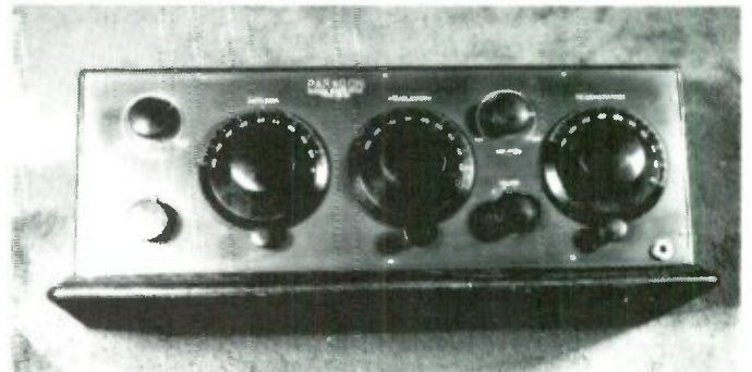
Paragon RB2A, three tube regenerative receiver of 1923. It sold for $135.00 at the time. It was made by the Adam Morgan Company of New Jersey. Typically, it had a detector followed by two stages of audio amplification. Jacob collection.
