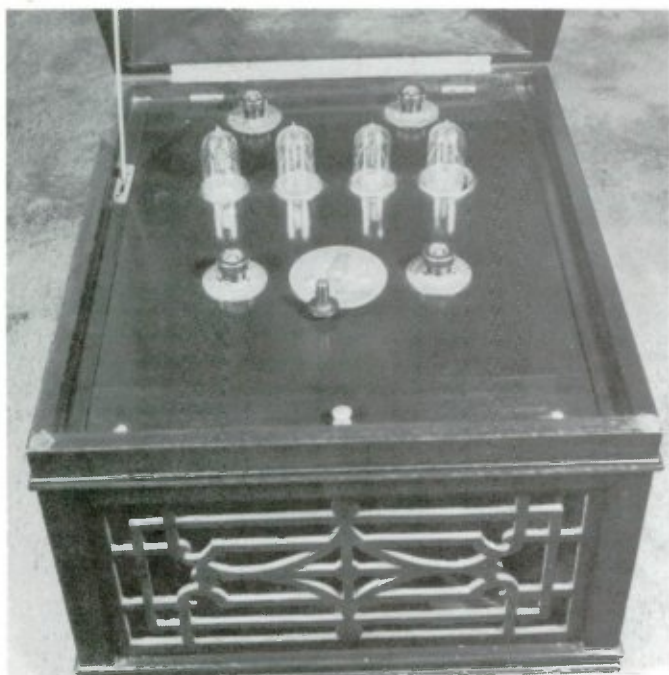
RCA Grand Radiola of 1922. Battery and horn were internal. Used four tubes in a regenerative circuit, with a single tuned stage. It sold for $350.00 in its day. Jacob collection.
