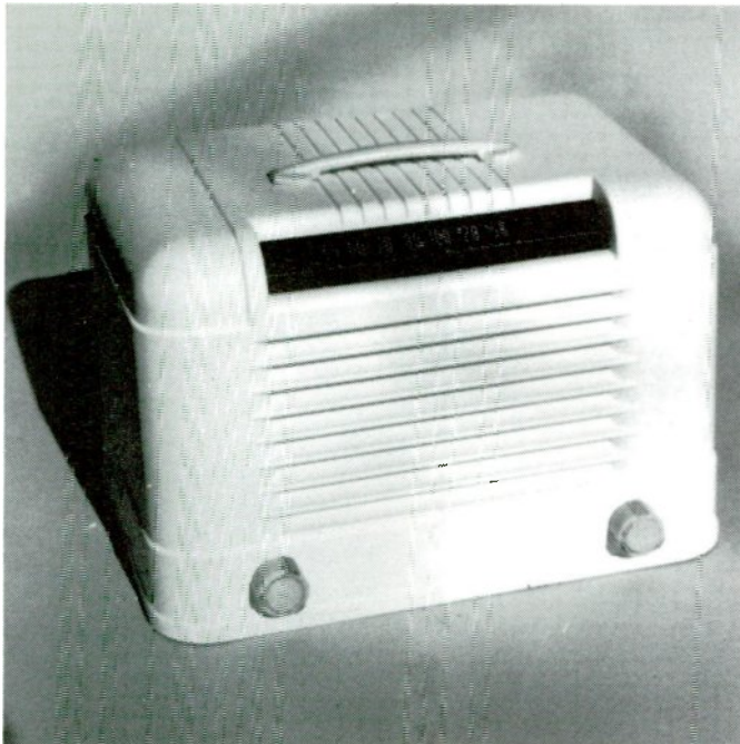
Exterior of RCA Model 12X2, a five tube, series filament, superheterodyne midget, circa 1938. Author's collection.
