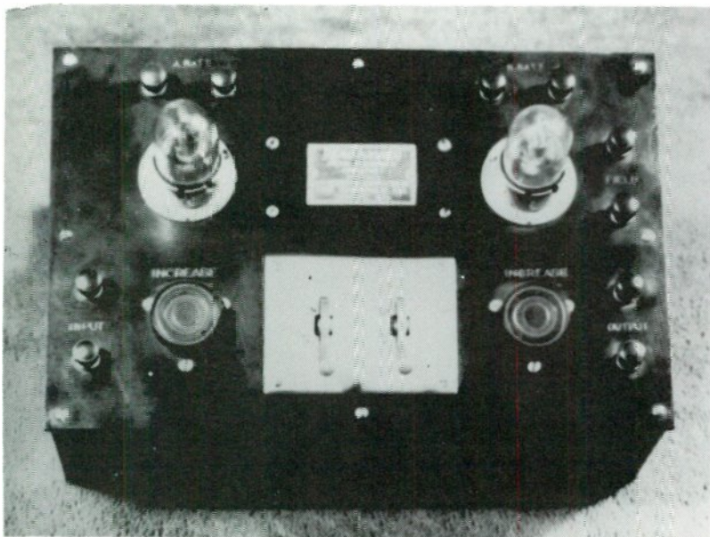
Magnavox, two-tube, battery-powered audio amplifier, circa 1920 (?). Jacob collection.
