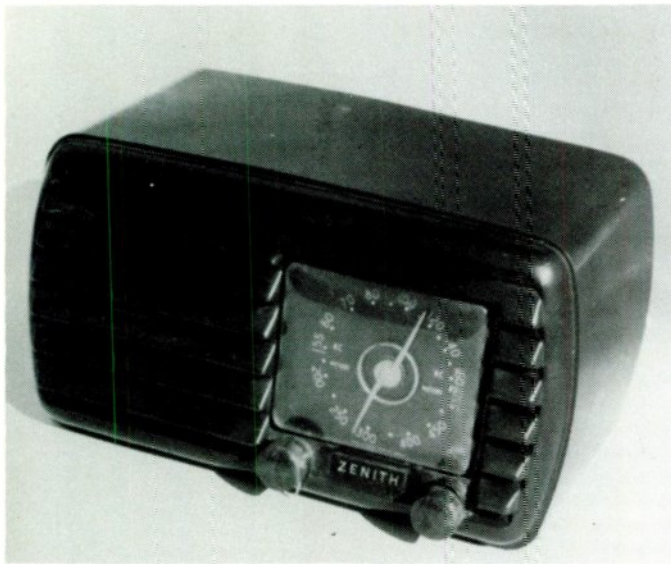
Zenith 5D-611, a five-tube, series-filament superhet. Manufactured about 1941.
