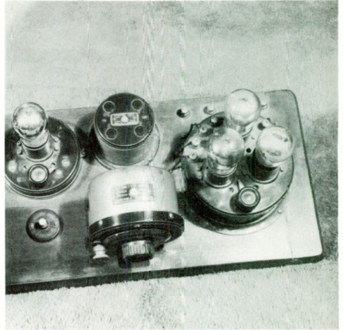
Close-up of the same receiver showing the audio section. Jacob collection.
