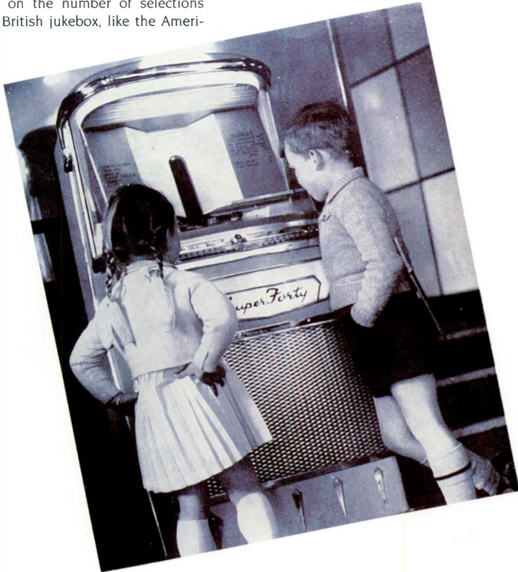
Above The scaled down British version of AMI's Model H was a coffee bar favourite. Holding only 20 records, the Super 40 was the luxury version of the Bal-AMI Junior which was a similarly scaled down G. Unlike other Bal-Amis the Super 40 featured a specially designed mechanism.
