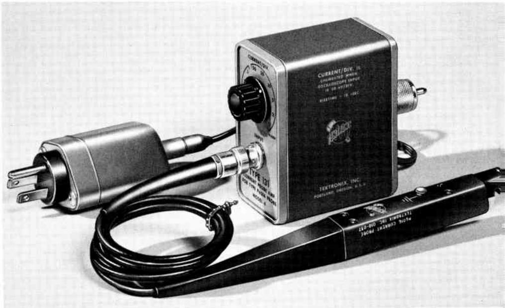
FIGURE 20.2 CURRENT PROBE AND AMPLIFIER
