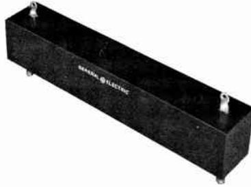
4JA220, 4JA420-421-422 Series: Mounted in standard eight pin tube base (4JA220-420 Series) or in rectangular design with solder lug connections (4JA221-421-422 Series). Available in a large number of circuit configurations. One to 20 cells may be potted in a single circuit. Individual cell specifications determine ratings. 4JA220 Series utilize germanium 1N91-93 cells. 4JA420-421-422 Series utilize silicon 1N536-540, 1N1095 cells. (See BASIC RECTIFIER CELL LISTING.)
