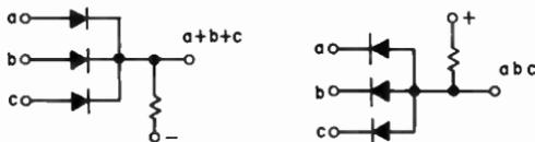
Logic is performed by diodes. The output is not inverted. Amplifiers are required to maintain the correct logic levels through several gates in series.
