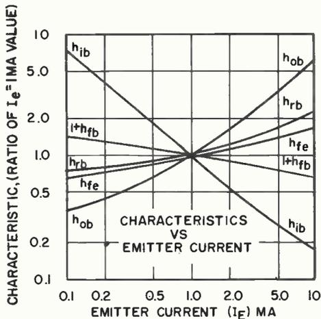
The a-c voltage gain  $\frac{e_{out}}{e_{in}}$  is approximately equal to  $\frac{R_L}{h_{ib}}$ . For the circuit shown this would be  $\frac{5000}{30}$  or approximately 167.
