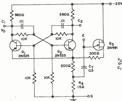
**BASIC HYBRID TIMING CIRCUITS USING PNP AND NPN TRANSISTORS**
