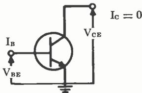
$$V_{CE} = I_B R_E + \frac{1}{\Lambda} \ln \frac{1}{\alpha_1} \quad (4j)$$
