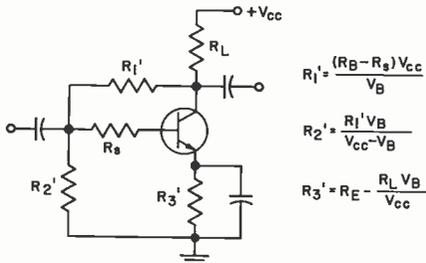
VOLTAGE DIVIDER TYPE BIAS CIRCUIT WITH FEEDBACK
