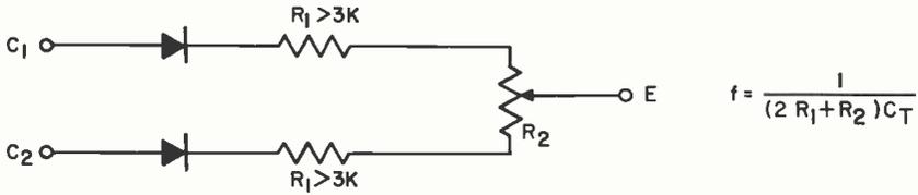
This configuration gives a multivibrator which has a constant frequency but a variable duty cycle.
