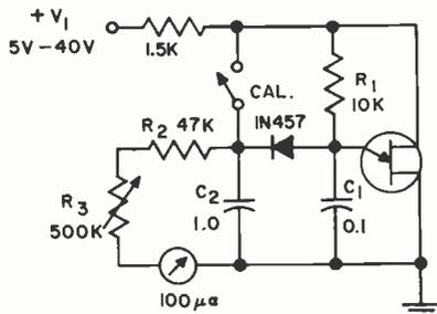
TEST CIRCUIT FOR INTRINSIC STANDOFF RATIO ( $\eta$ )
