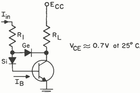
Collector current clamp using silicon and germanium diodes
