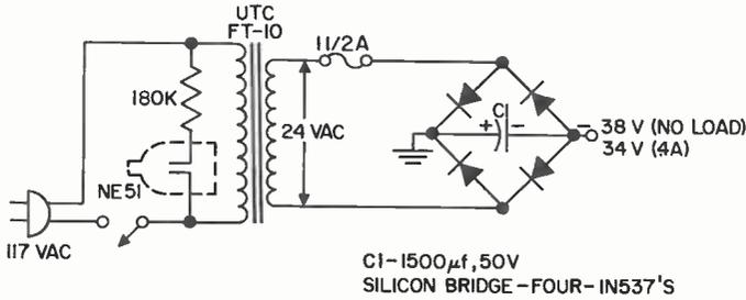
**POWER SUPPLY FOR DUAL SEVEN-WATT AMPLIFIERS**
