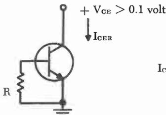
$$I_{CER} = \frac{(1 + \Delta I_{EO} R) I_{CO}}{1 - \alpha_N \alpha_1 + \Delta R I_{EO} (1 - \alpha_N)} \quad (4h)$$
