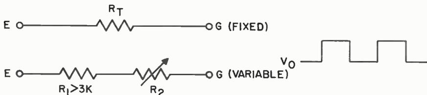
Connecting the resistor between points E and G in the basic circuits gives a square wave generator which has perfect symmetry. By the use of a 2 megohm potentiometer the frequency may be varied continuously from 1 cps to 500 cps. The frequency is  $f = 1/2 R_T C_T$ .
