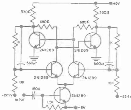
CIRCUIT OF FIGURE 11.13(B) WITH TRIGGER STEERING ADDED FOR COUNTER APPLICATION
