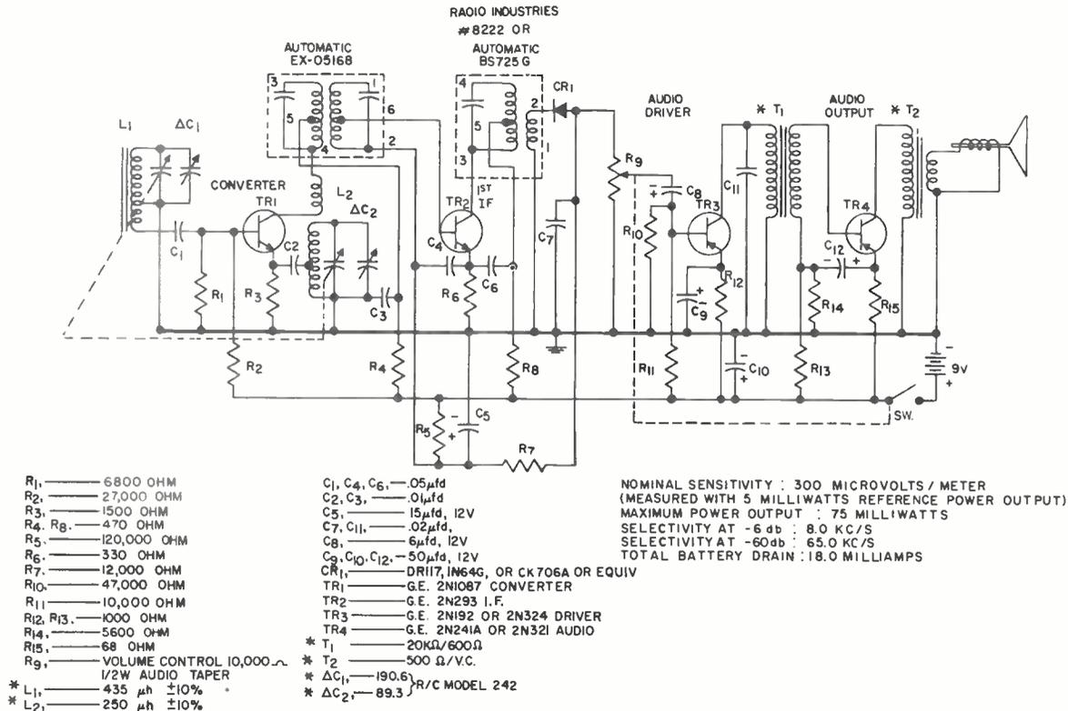
**FOUR TRANSISTOR SUPERHETERODYNE BROADCAST RECEIVER**
