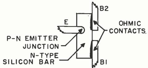
Construction of unijunction transistor—cross sectional view
