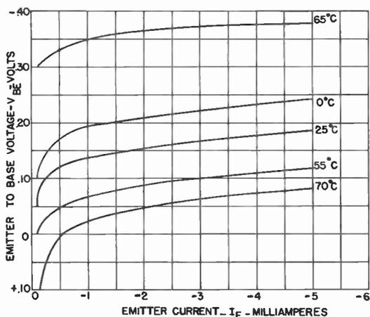
INPUT CHARACTERISTICS OF 2N525 ( $V_{CE} = 1V$ )
