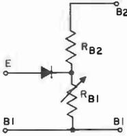
Unijunction transistor representative circuit
