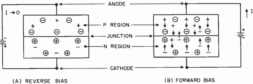
CONDUCTION IN A PN JUNCTION RECTIFIER
