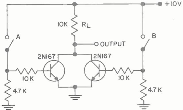
(A) GATE USING NPN TRANSISTORS
