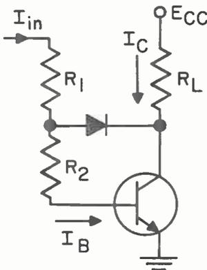
$$V_{CE} \approx \frac{R_2 E_{CC}}{R_L h_{FE} + R_2}$$
