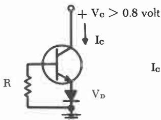
$$I_C = - \frac{(1 + \Delta I_{EO} R - \alpha_1 \Delta V_D) I_{CO}}{1 - \alpha_N \alpha_1 + \Delta R I_{EO} (1 - \alpha_N)} \quad (4i)$$
