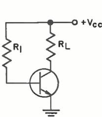
$$I_c = h_{FE} \left( \frac{V_{CC}}{R_1} + I_{CO} \right)$$
