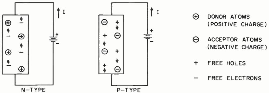
CONDUCTION IN N-TYPE AND P-TYPE SEMICONDUCTORS
