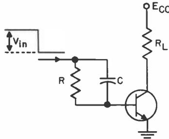
Stored charge neutralization by capacitor
