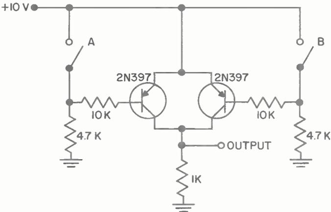
(B) GATE USING PNP TRANSISTORS
