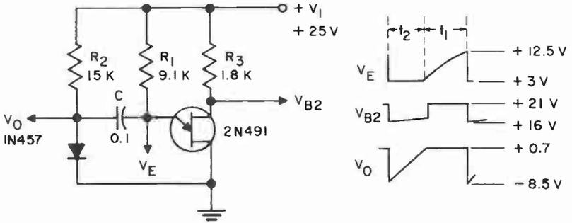
**UNIUNCTION TRANSISTOR MULTIVIBRATOR**
