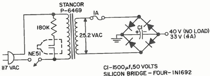
**POWER SUPPLY FOR SEVEN-WATT AMPLIFIER**
