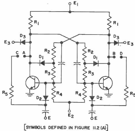
**CIRCUIT CONFIGURATIONS FOR NON-SATURATING FLIP-FLOP WITH CLAMPED OFF VOLTAGE**
