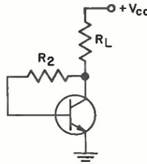
$$I_c = \frac{h_{FE} (V_{CC} + I_{CO} R_2)}{R_2 + h_{FE} R_L}$$
