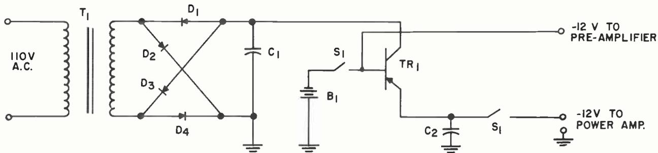
TR<sub>1</sub> - POWER TRANSISTOR (MOUNT ON HEAT SINK) C.B.S. 2N256, 2N156 OR EQUIVALENT.
