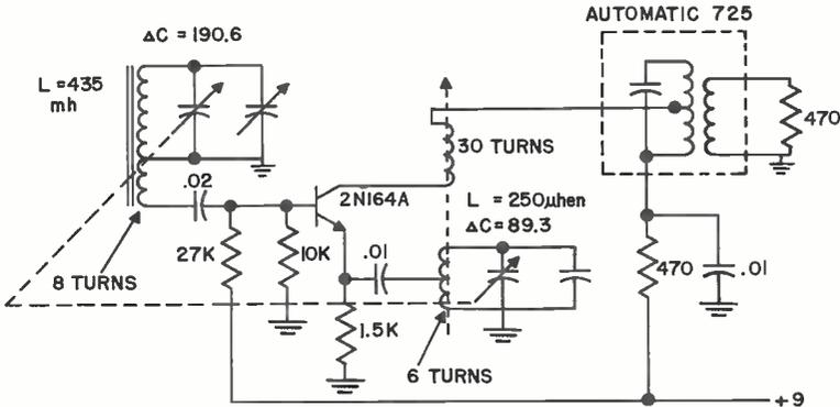
ANTENNA - DELTA COIL #1 - 105A OR EQUIVALENT
