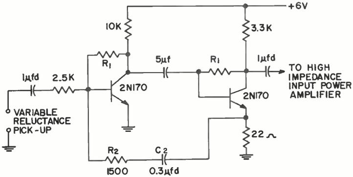
R<sub>1</sub> (100K - 500K) SHOULD BE CHOSEN TO MAKE COLLECTOR VOLTAGE 2.5 TO 3.5 VOLTS
