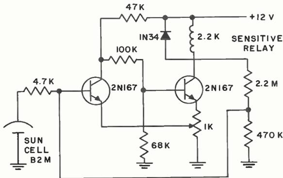
THE RELAY IS ENERGIZED WHEN A 100 WATT LAMP IS PLACED 5" FROM THE SUN CELL. THE VOLTAGE NEEDED AT THE SUN CELL TO OPERATE THE RELAY VARIES WITH TEMPERATURE AS FOLLOWS:
