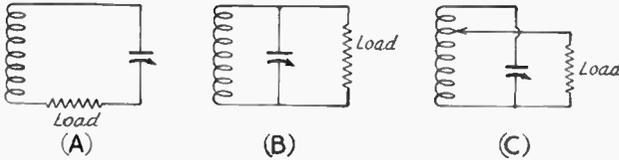
ance has the following values: 10, 20, 70, 150, 600, 2000, 5000 ohms. Find the value of capacity which should be used in each case, and also the value of inductance necessary to tune to resonance in each case.
