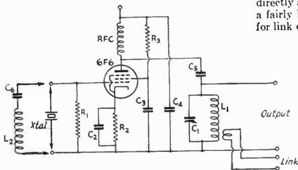
Fig. 2 — Oscillator circuit.
