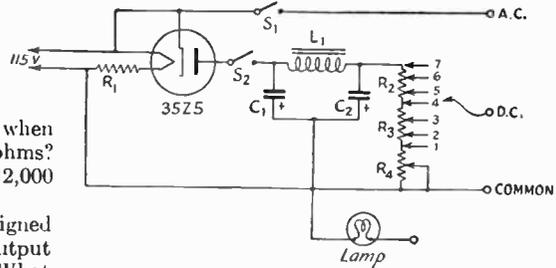
Fig. 2 — Circuit diagram of the transformerless power supply.
