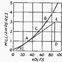
While there is bound to be some inaccuracy in drawing the tangent, in general the results will be nearer the truth than if two points on the curve itself are selected. Of course if the curve is straight the curve and its tangent coincide, so that in the special case of a straight-line curve points can be taken directly from the curve.
