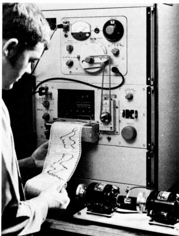
Figure 6-5. Typical application of a vibration pickup. It is mounted on the end bell of the left motor in the foreground and the vibration signal is being analyzed by a General Radio automatic-recording 1/3-octave-band analyzer.
