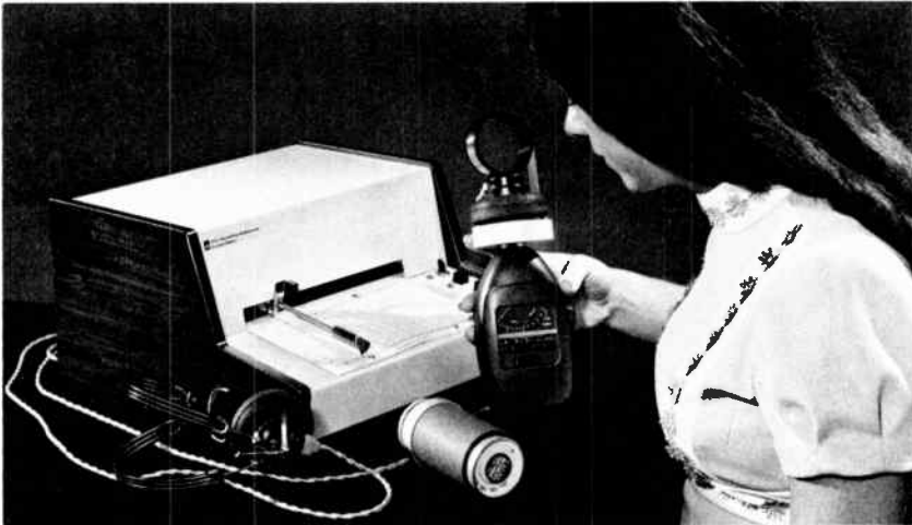
Figure 6-32. The GR 1562-Z Audiometer Calibrator shown measuring the output of a 1703 Audiometer earphone.
