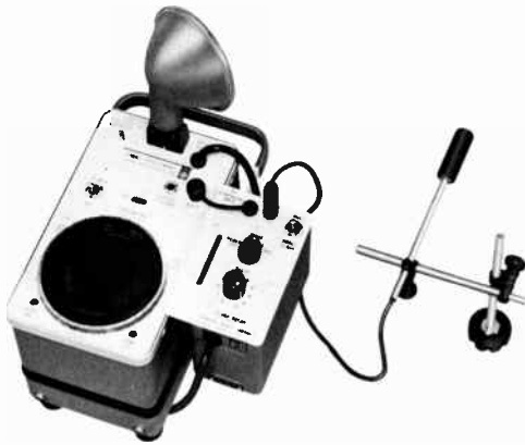
Figure 6-33. Type 1531 Strobotac ® electronic stroboscope (left), Type 1531-P2 Flash Delay (attached to stroboscope), and Type 1536-A Photoelectric Pickoff.
