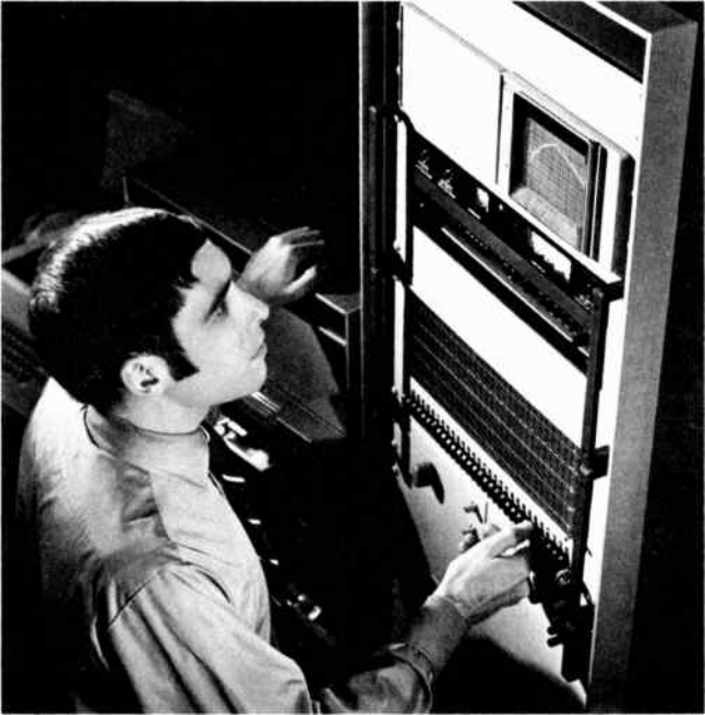
Figure 6-18. The Type 1921 Real-Time Analysis System operating under computer control. The computer and peripherals are shown at left.
