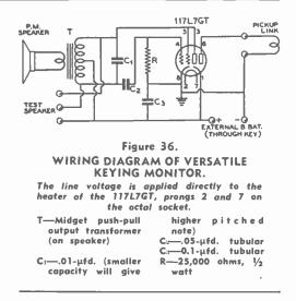
the signal generated by the keying monitor. Likewise, any keying lag will be apparent, because the strength of the monitor signal is determined by the strength of the carrier.
