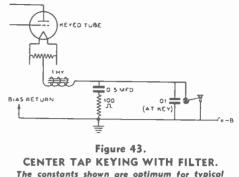
The constants shown are optimum for typical values of plate voltage and plate current, under average conditions. However, some alteration of these values may be required in some instances to give complete suppression of clicks. When high plate voltage is used, a relay should be substituted for the key.
