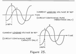
The above two illustrations show the manner in which a pure inductance or a pure capacitance (no resistance component in either) will cause the current in the circuit either to lead or to lag the voltage by 90 degrees. frequency increases. When the frequency is fixed, the reactance will be greater as the capacity is lowered.
