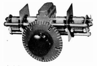
The Micrometer dial reads direct to one part in 500. Division lines are approximately 1/4" apart. The dial revolves ten times in covering the tuning range, and the numbers visible through the small windows change every revolution to give consecutive numbering by tens from 0 to 500. The condenser is of extremely rigid construction, with four bearings on the rotor shaft. The drive, at the mid-point of the rotor, is through an enclosed preloaded worm gear with 20 to 1 ratio. Each rotor is
