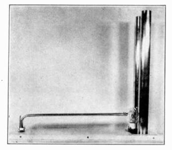
Figure 10. TYPICAL U.H.F. PUSH-PULL OSCILLATOR USING CLOSE-SPACED RESONANT PIPES FOR FREQUENCY CONTROL. A "Twin-30" special u.h.f. dual
