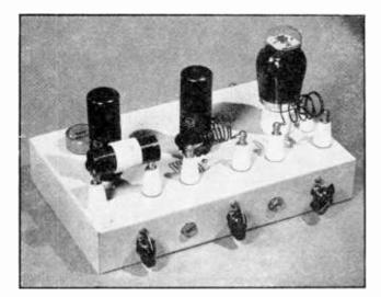
Figure 14. THREE-STAGE 20-WATT CRYSTAL-CONTROLLED 50-MC. EXCITER UNIT. A 6L6 oscillator on 6250 kc. drives a 6L6 quadrupler, which in turn drives a T21 doubler to 50 Mc.
