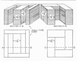
Figure 39. TYPES OF TRANSFORMER CORES.
