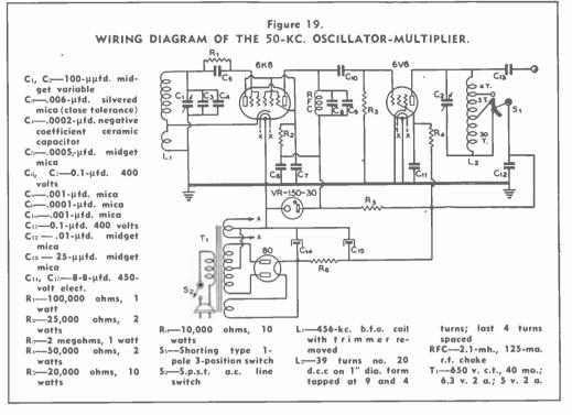
necessary to series these two coils as shown in the manufacturer's diagram as the connection for an electron-coupled oscillator. The cathode of the oscillator-mixer tube is then connected to the tap. The actual connections to the coil are as follows: blue wire, ground; green wire, grid; red and black connect together and go to cathode.
