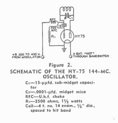
as to take up as little space as possible when placed alongside the modulator system for the mobile 10-meter transmitter. Normal operation of the oscillator will be with 300 volts at about 80 ma. on the plate. If desired, the power input may be raised to 425 volts at 80 ma. to give about 35 watts input. The circuit diagram of the oscillator is shown in Figure 2.
