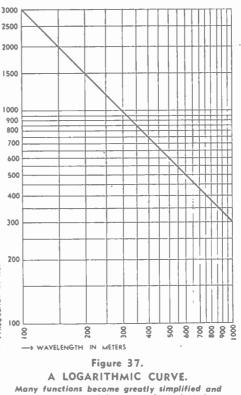
Many functions become greatly simplified and some become straight lines when plotted to logarithmic scales such as shown in this diagram. Here the frequency versus wavelength curve of Figure 31 has been replotted to conform with logarithmic axes. Note that it is only necessary to calculate two points in order to determine the "curve" since this type of function results in a straight line.
