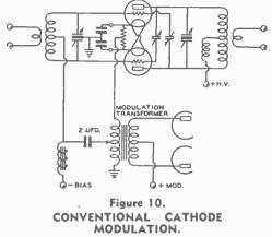
The modulation transformer in series with the cathode return of the modulated stage must match the cathode impedance of this stage. The choke in series with the grid return of the stage should have from 15 to 40 henrys inductance and should be capable of carrying the full grid current of the stage. The grid tap on the modulation transformer is varied, after the stage has been placed into operation, to give the best modulation pattern.
