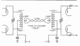
Figure 36. PUSH-PULL LINK COUPLING.
