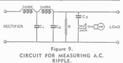
The meter should not be inserted in the circuit until after the voltage is turned on; otherwise the charging current surge may blow the meter. The jack must be of the closed-circuit type. C: must be rated at considerably more than the plate voltage to provide a safety factor.
