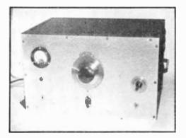
Figure 9. 20-25 WATT V.F.O. FOR 20, 40, AND 80 METERS.
