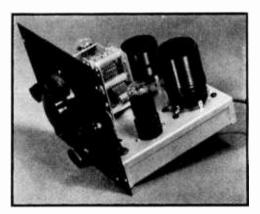
Figure 44. TEST SIGNAL GENERATOR. This signal generator covers the range from 440 to 1500 kc. in two jumps. A voltage regulator tube prevents change in plate voltage with line voltage fluctuations.
