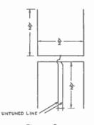
Figure 2. H TYPE ARRAY ARRANGED FOR VER-TICAL POLARIZATION.
