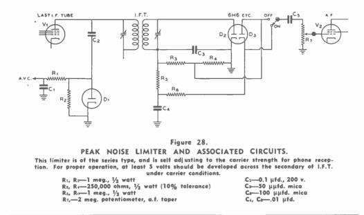
jection is not too high. Variable injection is to be preferred, adjustable from the front panel. If this feature is not provided, the b.f.o. injection should be reduced to the lowest value that will give a satisfactory beat. When this is done, effective limiting and a good beat can be obtained by proper adjustment of the r.f. and a.f. gain controls. It is assumed, of course, that the a.v.c. is cut out of the circuit for c.w. telegraphy reception.
