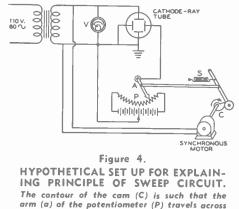
the winding at a uniform rate in one direction and then immediately flies back to repeat the action at regular intervals.
