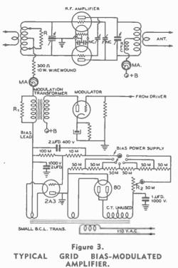
Note especially the r.f. and a.f. swamping resistors, R and R<sub>1</sub>, and the voltage regulated bias pack. The 300-ohm grid resistor is for the purpose of parasitic suppression, not bias.
