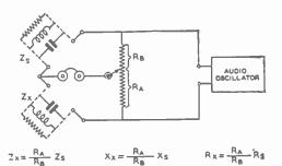
$$\begin{split} Z_X = & \text{impedance being measured, } R_S = \text{resistance component of } Z_S\\ Z_S = & \text{impedance op standard, } X_X = \text{reactance component of } Z_X\\ R_X = & \text{resistance component of } Z_X, \\ X_S = & \text{reactance component op } Z_S \end{split}$$
