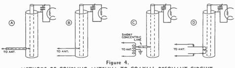
METHODS OF COUPLING ANTENNA TO COAXIAL RESONANT CIRCUIT. (A) Coupling a concentric line feeder to a concentric line resonant circuit. (B) Unbalanced method of coupling 2-wire line into a concentric line circuit. (C) Balanced-to-unbalanced method of coupling a 2-wire line to a concentric line resonant circuit. (D) Balanced loop method of obtaining good coupling from 2-wire line to a concentric line circuit.
