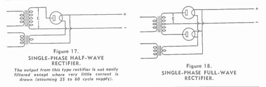
gle-phase a.c. line supply consist of a halfwave rectifier, as shown in Figure 17, a fullwave rectifier, as shown in Figure 18, and a bridge rectifier circuit as shown in Figure 19.
