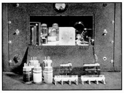
Figure 17. ILLUSTRATING METHOD OF CHANGING COILS. Coils are changed through a door in the front panel. A safety switch automatically disconnects the primary a.c. voltage when the door is opened.
