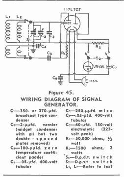
Coils The two coils are wound on 2-inch diameter bakelite tubing with No. 24 enamelled wire. The high frequency coil has a plate winding of 36 turns, close-wound, and a tickler winding of approximately 35 turns, closewound. The two windings are separated about 1/8 inch.
