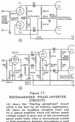
power audio tubes when a conventional crystal or high-impedance dynamic microphone is used on the input. The circuit shown at (A) is quite flexible and is capable of considerable change to suit different circuit conditions. That shown at (B) should be used as is without change if its excellent operating characteristics are to be retained. Both circuits are fully described in the accompanying text.
