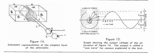
rotated. This current will flow out through the collector rings R and brushes B to the external circuit, X-Y.
