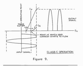
of a class C amplifier with twice cut-off bias and with the peak grid swing of such a value as just to approach the diode bend in the plate characteristic. When the excitation voltage is increased beyond this point, the plate current waveform will have a dip at the crest due to the taking of electrons from the plate current stream by the grid on its highly positive peaks.
