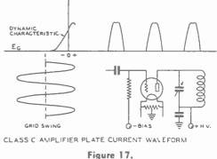
torted plate current wave form in the form of pulses as shown in Figure 17. The LC circuit is tuned to resonance, and its purpose is to smooth out these pulses, by its storage or "tank" action, into a sine wave of radio-frequency output. Any wave-form distortion of the carrier frequency results in harmonic interference in higher-frequency channels.
