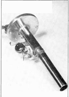
Figure 17. CONSTRUCTION DETAIL OF OSCILLATOR. The assembly shown below can be slid out intact after the plate conection to the 955 is disconnected.
