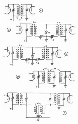
Figure 17. I.F. AMPLIFIER COUPLING ARRANGEMENTS. All of these arrangements give a better shape factor (more straight sided selectivity curve) than would the same number of resonant circuits coupled by means of tubes.
