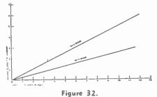
Only two points are needed to define functions which result in a straight line as shown in this diagram representing Ohm's Law.
