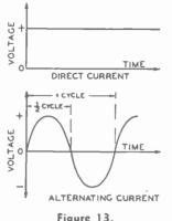
Figure 15. Graphical comparison of unidirectional (direct) current and alternating current.
