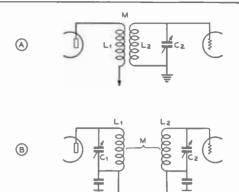
Figure 34. Two commonly used types of inductive coupling between radio frequency circuits. With the arrangement at "A," the coupling between L, and L: is made quite close.
