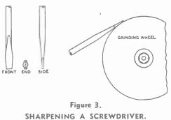
The way to hold the screwdriver blade on the grinding wheel while sharpening it, and the appearance of a properly sharpened blade.
