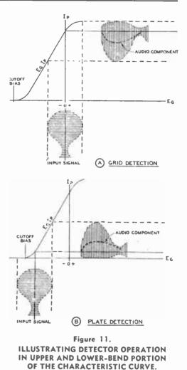
radio-frequency signal carrier at the receiver. Detection always involves either rectification or nonlinear amplification of an alternating current.
