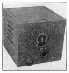
Figure 21. 5-BAND HIGH GAIN PRESELECTOR. This high gain preselector uses an 1851 tube, tuned output circuit, and moderate regeneration. It makes a worthwhile addition to any receiver having less than 2 r.f. stoges.
