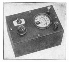
Figure 3. LOW RANGE OHMMETER. This ohmmeter is particularly useful for measuring resistances too low to be read accurately on an instrument of the type diagrammed in Figure 2.
