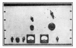
Figure 19. 100-WATT 10-160 METER BAND-SWITCHING EXCITER. This exciter delivers about 90 watts on 10 meters and well over 100 watts on lower frequency bands.
