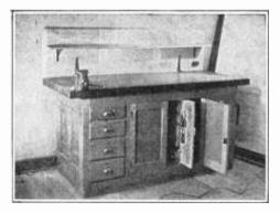
Figure 7. ENCLOSED-TYPE WORKBENCH. An enclosed-type workbench with three drawing boards along the rear making up the backboard. The shelf along the backboard serves to strengthen it, and furnishes additional storage space.
