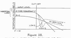
TYPICAL RESPONSE CURVES OF COM-MON LOW-PASS FILTER CIRCUITS.
