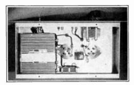
Figure 31. UNDER-CHASSIS VIEW OF SENSITIVE F.S. METER. The combined "A" and "C" battery is strapped under the chassis as shown here.
