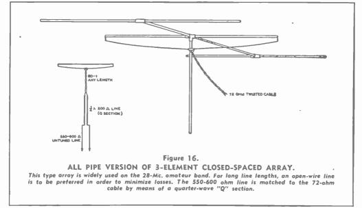
determined by cut and try. For a starter, the reflector may be made exactly  $\frac{1}{2}$  wavelength, the driven element 0.96 of a half wavelength, and the director 0.92 of a half wavelength. A half wavelength for a given frequency may be determined by dividing the frequency into 492, the answer being in feet if the frequency is in megacycles.
