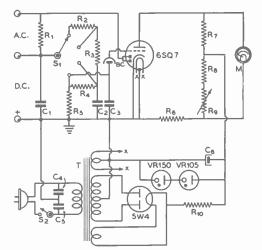
Figure 8. WIRING DIAGRAM OF THE A.C.-D.C. VACUUM-TUBE VOLTMETER
