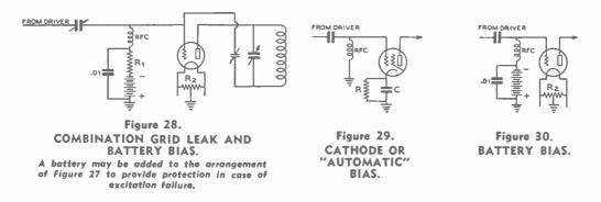
r.f. excitation. Grid-leak bias cannot be used for grid-modulated or linear amplifiers in which the average d.c. grid current is constantly varying with modulation.
