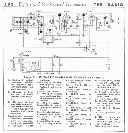
Coil L<sub>1</sub> consists of 30 turns of no. 24 enamelled, close-wound on a  $\frac{7}{8}$ -inch diameter ceramic form, with cathode tap 10 turns from the ground end, mounted in coil shield.
