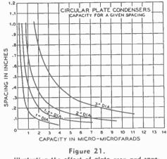
Illustrating the effect of plate area and spacing upon the capacity of a condenser having two flat, circular electrodes. The capacity given is for a dielectric of air.
