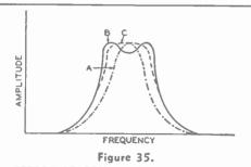
EFFECT OF COUPLING BETWEEN CIR-CUITS UPON THE RESONANCE CURVE. Curve A indicates the curve when the circuits are under coupled, B is the curve resulting from over coupling, and C is the curve resulting from a critical value of intermediate coupling, called "critical coupling."
