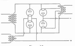
Figure 19. BRIDGE CIRCUIT.
