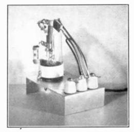
Figure 7. 8-WATT HY-75 220-MC. OSCILLATOR This small HY-75 transmitter is ideal for the amateur who wishes a medium-power 11/4meter oscillator for both fixed station and portable use.
