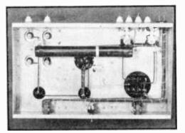
Figure 34. UNDER-CHASSIS VIEW OF THE 1500-VOLT SUPPLY.
