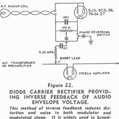
nodulated stage. It is widely used in broadcast practice, but cannot be employed to full advantage in a transmitter using class B plate modulation with an inexpensive modulation transformer. The leakage reactance of the latter encourages undesirable oscillations, unless the feedback factor is low.
