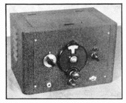
Figure 39. FREQUENCY METER, C.W. MONITOR, EMERGENCY C.W. RECEIVER. This unit is completely self-contained and self-powered. Bandswitching is used to eliminate the need for changing coils.
