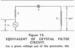
voltage developed across Z: depends upon the ratio of the impedance of X to the sum of the impedances Z and Z. Because of the high Q of X, its impedance changes rapidly with frequency.
