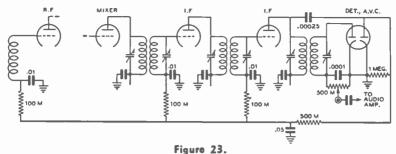
DOUBLE-DIODE DETECTOR-A. V. C. CIRCUIT. Any of the ordinary small dual-diode tubes may be used in this circuit. The left-hand diede serves as the detector, while the right-hand section operates as an a.v.c. rectifier. Using separate diodes for the detector and a.v.c. functions help to improve the audio fidelity.
