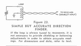
signal. Then check to see if the two minima that are observed as the loop is rotated are exactly 180 degrees apart. If not, the loop is not tuned to exact resonance, and the tuning should be altered slightly as necessary to cause the two minima or nulls to fall exactly 180 degrees apart. When this is done, either null may be taken as a bearing.
