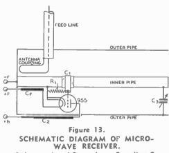
$R_1$  has a value of 2 megohms. Capacitors  $C_1$ ,  $C_1$ , and  $C_7$  are described in the text. Tuning capacitor  $C_1$  is shown in detail in Figure 15.
