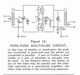
tion of the fundamental and all *odd* harmonics, an advantage when spurious emissions must be minimized. Another advantage is that when the available excitation is low and excitation pulses exceed 90 degrees, the output and efficiency will be greater than for the same tubes connected in parallel.
