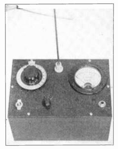
Figure 33. RADIOPHONE TEST SET. This versatile instrument can be used as a modulation monitor, absorption wavemeter, field strength meter, carrier-shift indicator, and neutralizing indicator.
