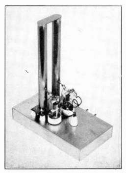
Figure 9. PUSH-PULL 220-MC. HY-75 OSCILLATOR.
