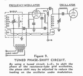
ing a resistor in series with the oscillator tank condenser. Since the current through the tank condenser leads the voltage across the tank circuit by 90 degrees, the r.f. voltage applied to the modulator grid will also lead this voltage by the same amount; the modulator plate current will lead the tank voltage, and the modulator tube will appear as a condenser.
