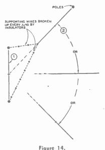
Illustrating how two dipoles or arrays with horizontal elements can be supported from three poles with a minimum of coupling between the two systems. This is an important consideration if maximum directivity is desired.
