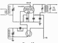
Figure 10. DUAL PURPOSE CONVERTER TUBE WITH SEPARATE OSCILLATOR.
