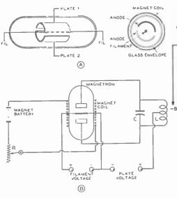
Figure 23. DETAILS OF SIMPLE MAGNETRON AND CIRCUIT.
