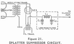
C1, C1, L1—Components of low-pass filter: characteristic impedance is the same as the class C load impedance; cutoff frequency is 3000 cycles.
