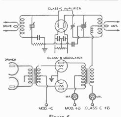
Figure 6. CLASS B PLATE MODULATION. This type modulation is the most practicable form of high level modulation for communications work.
