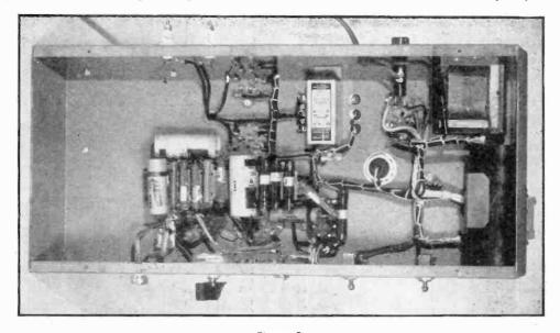
Figure 2. UNDER-CHASSIS VIEW OF THE 25-WATT MODULATOR. The filter choke and all resistors and condensers except C10 are mounted below the chassis. The use of a resistor strip adds to the appearance and facilitates checking and replacement of these units.
