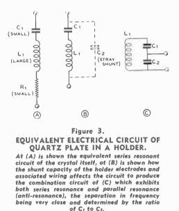
pressed or deformed in any way a potential difference will appear upon its opposite sides.
