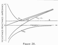
Variation in reactance and impedance of a series resonant circuit with changing frequency.
