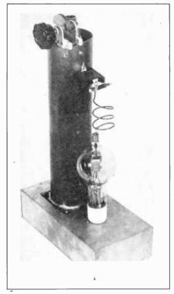
Figure 3. CONCENTRIC-LINE 75T OSCILLATOR This concentric-line oscillator with a 75T gives good stability and a quite reasonable power output on the 144-Mc. band.
