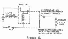
THE SIMPLEST CODE PRACTICE SET CONSISTS OF A KEY AND BUZZER.
