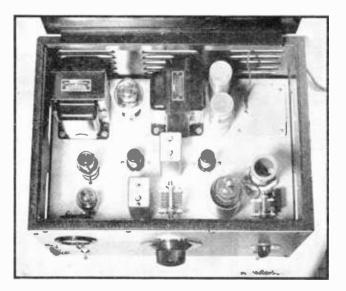
Figure 10. INTERIOR CONSTRUCTION OF V.F.O.-EXCITER.
