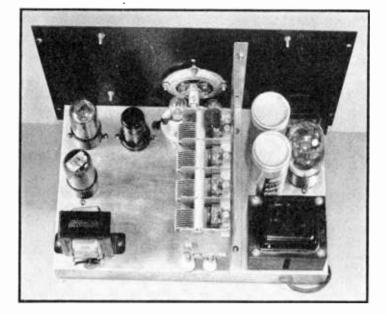
Figure 48. PLACEMENT OF COM-PONENTS ABOVE THE CHASSIS. Note especially the metal
