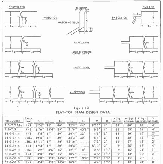
Dimension chart for flat-top beam antennas. The meanings of the symbols are as follows:
