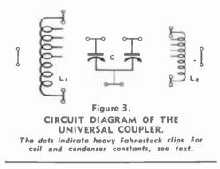
This coupling system operates by virtue of the fact that capacity coupling between the final tank and the antenna is eliminated by the grounded link and the grounded center tap of the antenna tank; also, due to the selectivity of the antenna tank against the harmonic frequencies, inductive coupling of them into the antenna system will also be attenuated.
