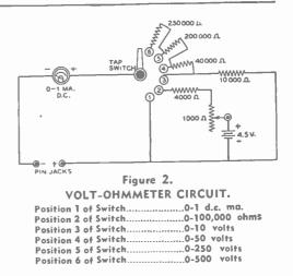
the full scale voltages being 10, 50, 250, and 500 volts respectively.
