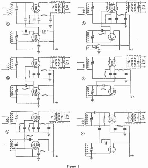
Figure o. MIXER-OSCILLATOR COMBINATIONS. The various oscillators do not have to be used with the mixers with which they happen to be shown. The triode oscillator shown at E could replace the pentode circuit shown at B, for instance.
