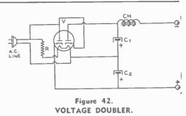
to 2.82 times the r.m.s. line voltage value. Because of its action, this circuit is known as a *voltage doubler*. At higher current levels, the output voltage is slightly under twice the line voltage.
