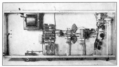
Figure 23. UNDER-CHASSIS VIEW OF THE 50-WATT F.M. TRANSMITTER. The filament transformer for the entire rig is shown in the left rear. The meter switch is mounted, with the resistors between its sections, directly in front of the resistor tie plate for the rig.
