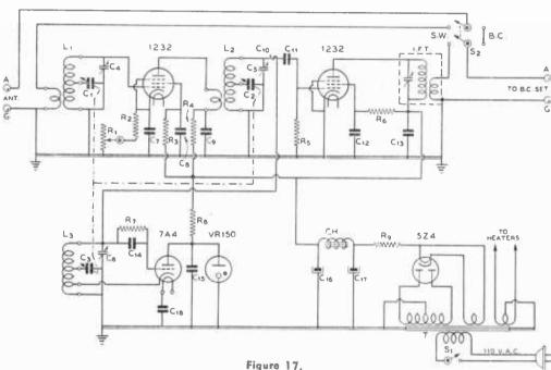
WIRING DIAGRAM OF THE CONVERTER.
