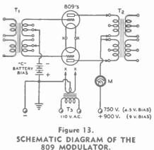
T1---Multiple-ratio input transformers; 4.S:1 step-down ratio usually used T2---Multiple-impedance output transformer T:---6.3-volt S-ampere filament transformer M---0-250 d.c. milliammeter
