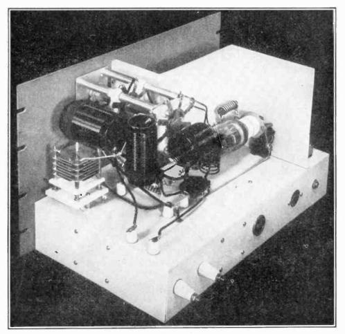
Figure 22. 814 OUTPUT AMPLIFIER OF 100-WATT BANDSWITCHING EXCITER. Four of the 5 coils are visible in this photo. The 10-meter coil is hidden by the bandswitch and tank condenser. The fixed air padding condenser, permanently connected across the 160-meter coil, may be seen in the left foreground.
