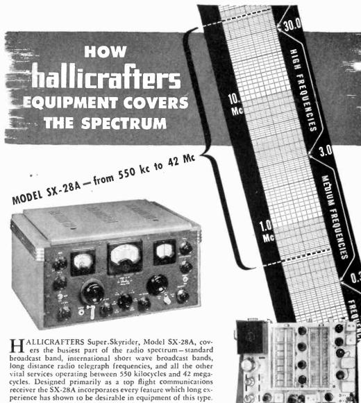
The traditional sensitivity and selectivity of the pre-war SX-28, ranking favorite with both amateur and professional operators, have been further improved in this new Super Skyrider by the use of "micro-set" permeability-tuned inductances in the RF section. The inductances, trimmer capacitors and associated components for each RF stage are mounted on small individual sub-chassis, easily removable for servicing.
