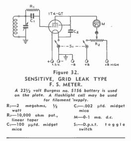
input; in fact, with sufficient input the plate current may begin to increase. This saturation or blocking point is easily determined simply by gradually increasing the r.f. input until the plate current no longer falls off. The meter then is calibrated just up *to* this point.
