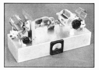
When the unit is tuned up initially, care should be taken to make sure the various doublers are working on their second harmonic and not their third harmonic.
