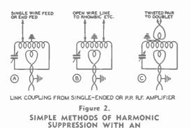
For a given number of turns in the coupling link, greatest coupling will occur when the link is placed around the center of the coil, regardless of the location of the node on the coil. For this reason, it is sometimes difficult to get sufficient coupling with an unsplit tank, as the link must be placed at the cold end of the coil in such a system to prevent detuning of the tank circuit, possible arcing between tank coil and link, and capacity coupling of harmonics.
