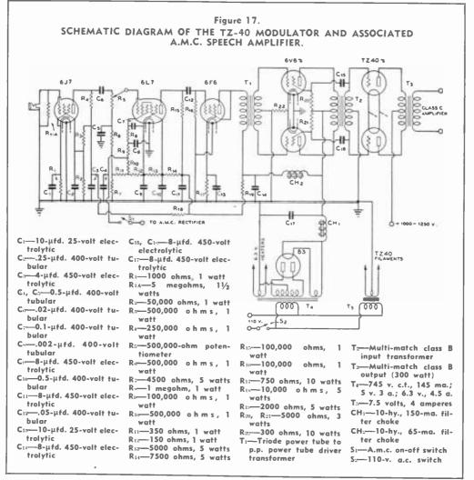
ble of fully modulating 600-watts input, and the plate current would kick up to 175 to 225 ma. under full modulation.
