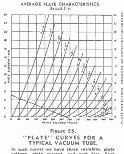
voltage, plate current, and grid bias. Each point on a grid bias line corresponds to the plate voltage and plate current represented by its position with respect to the X and Y axes. Those for other values of grid bias may be found by interpolation. The loadline shown in the lower left portion of the chart is explained in the text.
