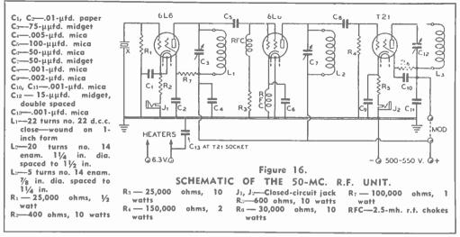
cially designed for u.h.f. service, it is possible to construct a medium power 50-Mc. amplifier that will exhibit good efficiency without resorting to the use of parallel rods in the plate circuit.
