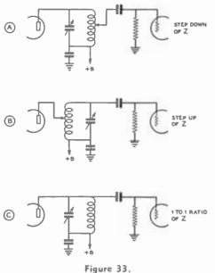
rigure 33. Impedance step up and step down may be obtained by utilizing the plate tank circuit of a vacuum tube as an auto-transformer. In this manner the dynamic plate load on the tube can be made any desired value.
