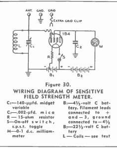
trimmer used as a pickup. If the trimmer is not used, a long pickup antenna will detune the meter.
