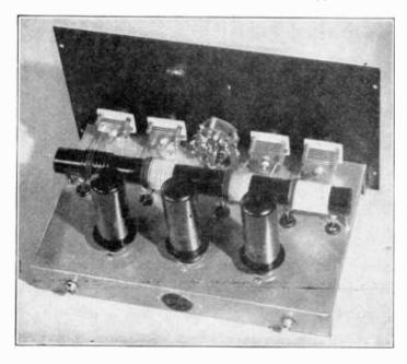
Figure 13. SHOWING CONSTRUC-TION OF MULTI-BAND FREQUENCY MULTI-PLIER.
