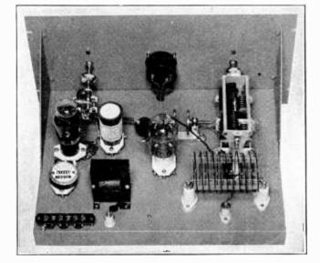
Figure 31. EXCITER CHASSIS. The 6L6-G harmonic oscillator and the HK-54 buffer-doubler stages are located on this deck.
