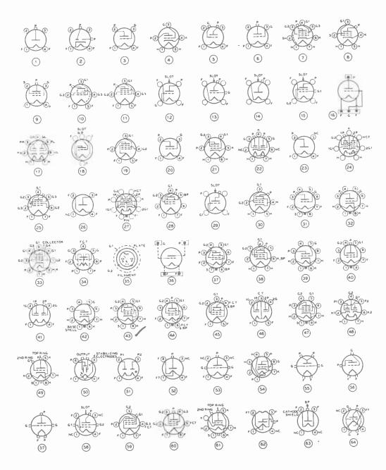
TRANSMITTING TUBE SOCKET CONNECTIONS—BOTTOM VIEWS
