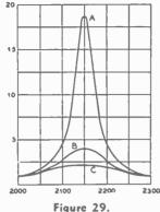
Resonance curve showing the effect of resistance upon the selectivity of a tuned circuit. The curves apply to voltage in a parallel resonant circuit or to current in a series resonant circuit.
