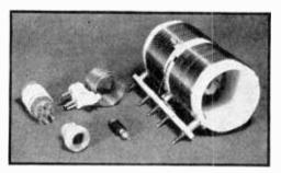
Figure 19. Common types of inductors employed in radio equipment. The smallest is a radio frequency choke coil; the largest is a power amplifier tank coil.
