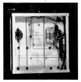
Figure 46. UNDER-CHASSIS VIEW OF SIGNAL GENERATOR.
