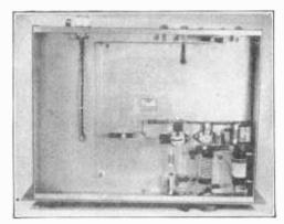
Figure 4. BOTTOM VIEW OF R.F. CHASSIS. The location of the plate coils for the two 6L6 stages is clearly shown in this photograph. It is important that the twisted leads connecting to the r.f. output terminals at the rear of the chassis be kept well separated from the HY 69 grid circuit.
