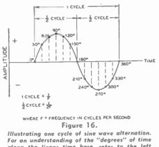
For an understanding of the "degrees" of time along the linear time base, refer to the left hand (rotating) representation of figure 15. As one cycle represents one revolution of the alternator, one cycle is said to constitute 360 electrical degrees.
