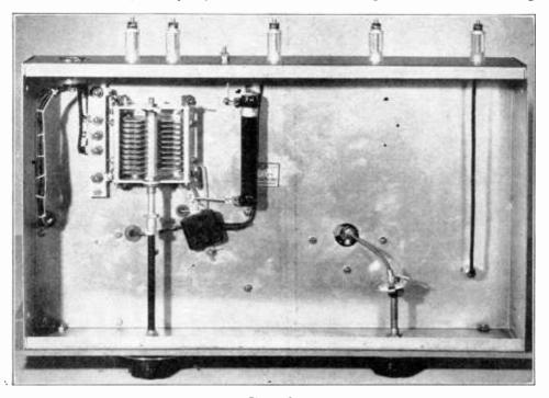
Figure 9. UNDER-CHASSIS VIEW OF THE SINGLE-ENDED AMPLIFIER. The grid condenser and bias resistor are located under the amplifier chassis. Note the flexible shaft which allows the vertically mounted plate condenser to be controlled from the panel.
