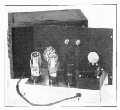
Figure 9. V.T.V.M. REMOVED FROM ITS CABINET. The power transformer, metal rectifier tube, and the two voltage regulator tubes are in a line, from right to left across the rear of the chassis. Rubber grommets insulate the meter terminals where they pass through the panel.
