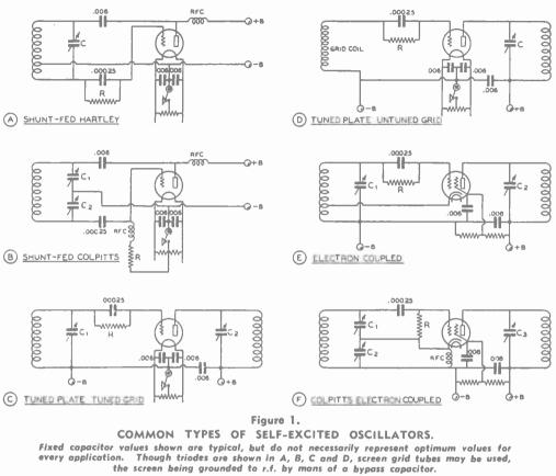
turn along the coil. Due to the inductive coupling between the portion of the coil in which the plate current is flowing and the grid portion, a potential will be induced in the grid portion.
