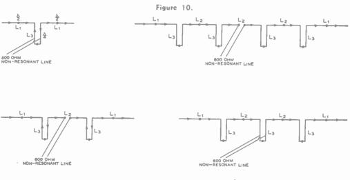
FRANKLIN OR CO-LINEAR ANTENNAS HORIZONTAL POLARIZATION BROADSIDE RADIATION
