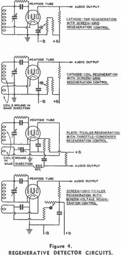
These circuits illustrate some of the more popular regenerative detectors. Values of I to 3 megohms for grid leaks are common. The grid condenser usually has a capacity of .0001 µfd., while the screen by-pass is 0.1 µfd. Pentode detectors operate best when the feedback is adjusted so that they start to oscillate with from 30 to 50 volts on the screen grid.
