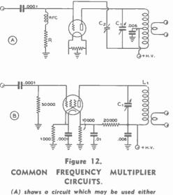
(A) shows a circuit which may be used either as a neutrolized straight amplifier or o regenerative frequency multiplier. (B) shows a pentade multiplier with cathode regeneration, a result of the undersized cathode byposs capacitar and large cathode resistar.
