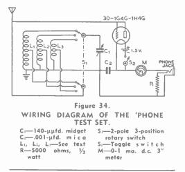
each coil covers two bands, there are gaps in the coverage of the entire range. However, if it is desired to cover the 10 to 20 and the 40 to 80 meter range, these two additional coils may be wound and a five-position range switch can be used.
