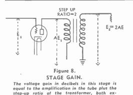
When one amplifier is to be followed by another amplifier, power gains are multiplied but the decibel gains are added. If a main amplifier having a gain of 1,000,000 (power ratio is 1,000,000) is preceded by a pre-amplifier with a gain of 1000, the total gain is 1,000, 000,000. But in decibels, the first amplifier has a gain of 60 decibels, the second a gain of 30
