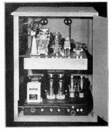
Figure 14. REAR VIEW OF R.F. AMPLIFIER AND MODULATOR.
