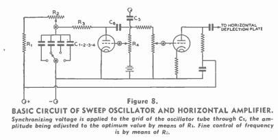
voltage varies badly, then it is possible that the oscillator will be sufficiently unstable that synchronization is difficult except at a 1-1 ratio.
