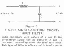
This type of filter is often used to feed a pushpull modulator stage (in which much of the plate voltage ripple cancels out) and telegraphy amplifiers in which slight modulation of the carrier can be tolerated.
