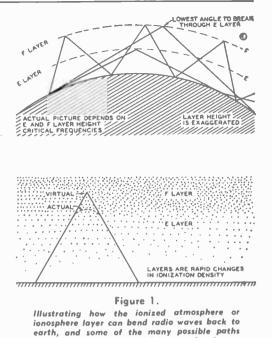
angle consistent with good signal strength for the frequency used. This cuts down the number of hops the signal has to make to reach the receiver, and consequently reduces the chance for arrival via different paths.
