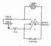
Figure 4. Diagram of the low-range ohmmeter illustrated in Figure 3.
