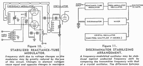
of this circuit. Changes in element voltages cause equal and opposite changes in reactance in the two modulators, thus minimizing the frequency shift. The reactance-tubes' grids receive excitation from a balanced tuned circuit so that one tube receives voltage lagging the oscillator tank voltage by 90°, while the other tube is excited with a voltage that leads the tank voltage by 90°.
