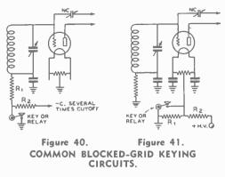
potential of several hundred volts above ground, with the attendant danger of shock to the operator. Blocked grid keying is not particularly effective for eliminating key clicks, though lag circuits can be incorporated which will reduce the clicks to an acceptable value.
