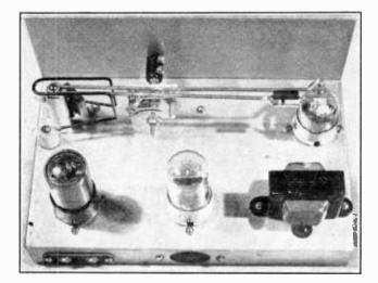
Figure 21. ILLUSTRATING MECHANICAL CONSTRUCTION OF 224-MC. RECEIVER.
