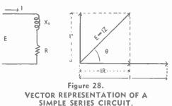
The righthand portion of the illustration shows the vectors representing the voltage drops in the coil and resistance illustrated at the left. Note that the voltage drop across the coil XL leads that across the resistance by  $90^\circ$ .
