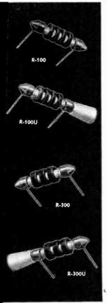
R-100 List S Without standoff insulator R-100U List S With standoff insulator R.F. chokes R-100 and R-100U are identical electrically, but the latter is provided with a removable standoff insulator screwed on one end. Both have Isolantite insulation and both have a continuous universal winding in four sections. Inductance 21/2 m.h.; distributed capacity 1 mmf.; DC re-sistance 50 ohms; current rating 125 ma.
