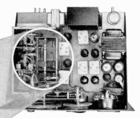
The RF section is built as a unit on a separate chassis which may easily be removed for servicing and incorporates a three position ceramic band switch. The positive action mechanical bandspread dial turns through more than 2200 divisions for each of the three ranges, 27.8 to 47, 46 to 82, and 82 to 143 megacycles.
