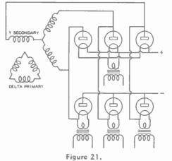
FULL-WAVE 3-PHASE RECTIFIER. Even with no filter the output of this rectifier will have a high percentage of d.c. A simple filter will suppress the small amount of ripple, because of the high ripple frequency (6 times supply frequency).
