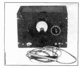
Figure 7. A.C.-D.C. V.T. VOLTMETER. The ranges for both a.c. and d.c. are 1, 10, 100, and 500 volts. The left knob operates the bridge-balancing control, and the one on the right operates the range switch.
