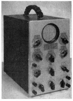
Figure 9. EXTERIOR VIEW OF TYPICAL MANU-FACTURED 3-INCH OSCILLOSCOPE.
