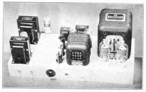
Figure 15. FRONT VIEW OF THE TZ-40 SPEECH AMPLIFIER-MODULATOR. This combined speech amplifier and modulator will fully modulate up to 600 watts on voice. It incorporates inverse feedback, a.m.c., and other features.
