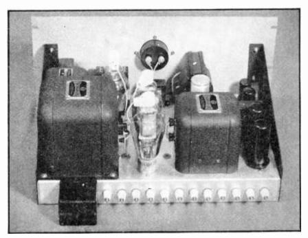
Figure 14. REAR VIEW OF THE CLASS B 811 MODULATOR INCORPORATING SPLATTER SUPPRESSOR.
