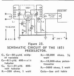
For maximum gain on the higher frequency range, tuning capacitors, sockets, and coil forms should have ceramic insulation.
