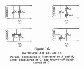
In both the above formulas  $C_B$  represents the amount of capacity variation supplied by the bandspread condenser. In well-designed midget condensers, the variation will approach the rated maximum capacity, and the maximum capacity may be used for  $C_B$  without serious error. In the first formula, the result  $C_F$ , will include all fixed capacities across the circuit, including the input capacity of the tube, stray capacity to ground, and the minimum capacity of the bandspread condenser.
