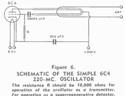
operation of the oscillator as a transmitter. For operation as a superregenerative detector, R should be removed and a 500,000-ohm resistor placed acrass the grid capacitor. The plate circuit of the 6C4 may then be fed into a conventional audio amplifier.
