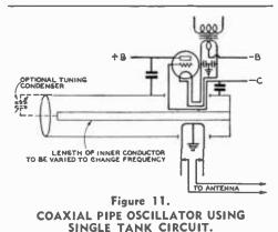
The frequency can be varied either by the optional tuning capacitor shown or by varying the length of the inner conductor of the concentric line.
