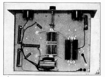
Figure 33. BOTTOM VIEW OF THE FINAL AMPLIFIER. The grid coil is shielded from the plate circuit by the metal supporting shelf.
