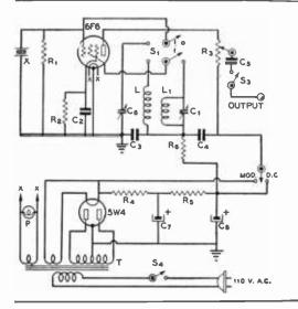
It should be borne in mind that the accuracy of the crystal when oscillating on 1000 kc. is not supposed to be sufficient for precision measurements; it is simply for convenience in identifying the highly accurate 100 kc. points.
