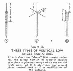
line, are shown in Figure 3. Antenna A is known as the "Sleeve" antenna, the lower half of the radiator being a large piece of pipe up through which the concentric feed line is run. At B is shown the Brown ground plane vertical, and at C a modification of this same array.
