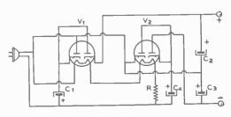
Figure 43. VOLTAGE QUADRUPLER.
