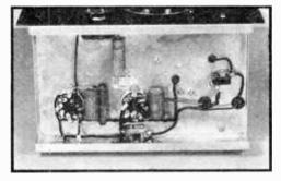
Figure 6. UNDER-CHASSIS VIEW OF U.H.F. SUPERREGENERATOR. Placement and wiring of the a.f. and d.c. components is not particularly critical.
