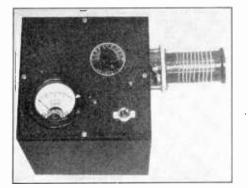
Figure 26. DIODE-TYPE FIELD STRENGTH METER. This field strength meter uses a type 30 connected as a diode; a 0-100 or 0-200 microammeter provides good sensitivity. The unit can be used as an absorption wavemeter if calibrated. It also can be used as a neutralizing indicator.
