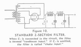
average electrolytic filter condenser is between 450 and 600 volts; the working voltage is usually rated at 450. When electrolytic condensers are used in filter circuits of high-voltage supplies, the condensers should be connected in series. The positive terminal of one condenser must connect to the negative terminal of the other, in the same manner as dry batteries are connected in series.
