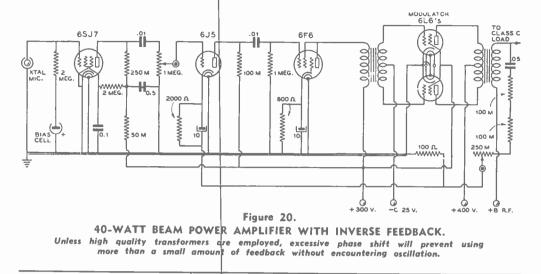
feedback to about 6.5 watts with the feedback circuit shown. The circuit consists simply of a high-gain audio stage, using a tube with high plate impedance, coupled to a beamtube or pentode output stage. Degenerative feedback is accomplished by the inclusion of the 500,000 ohm resistor from the plate of the output tube to the plate of the 6SJ7.
