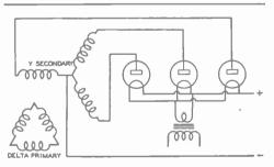
Figure 20. HALF-WAVE 3-PHASE RECTIFIER.
