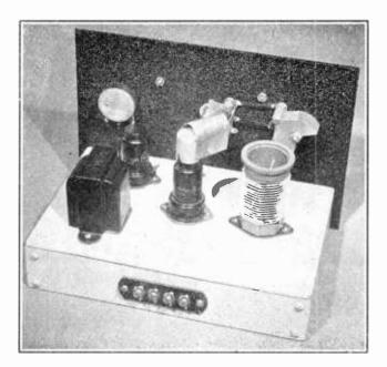
Figure 2. BACK VIEW OF THE 2-TUBE AUTODYNE. The chassis is made of wood and Masonite wall board. The "shield hat" for the grid leak and capacitor hides most of the main tuning capacitor.
