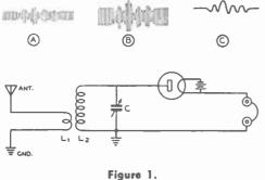
ELEMENTARY FORM OF RECEIVER. This diode detector with a single tuned circuit would make a very poor receiver, and is shown merely for purposes of illustration. (See text.)
