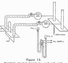
Practical physical layout for push-pull oscillator using resonant lines in filament, grid, and plate circuits.
