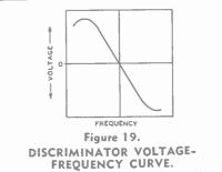
At its "center" frequency the discriminator produces zero output voltage. On either side of this frequency it gives a voltage of a polarity and magnitude which depend on the direction and amount of frequency shift.
