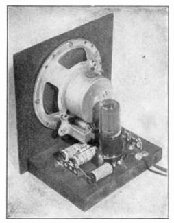
Figure 35. KEYING MONITOR AND CODE PRACTICE OSCILLATOR. This versatile unit may be used as a c.w. monitor, an audio "howler" for code practice, or as a test speaker requiring no field supply.
