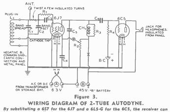
by substituting a 657 for the 615 and a 615-6 for the 605, the receiver can be run economically from dry cells for heater power. Only  $4\frac{1}{2}$  volts is required, and three no. 6 dry cells will give over 150 hours life.
