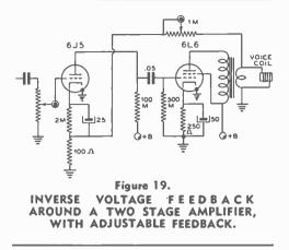
what different manner, as shown in Figure 19, for a two-stage amplifier. This method is particularly desirable, in that the tube driving the output stage does not have to deliver a high output voltage to offset the "bucking" effect of the feedback, as is the case where the feedback voltage is merely fed back from the plate to the grid circuit of the same stage.
