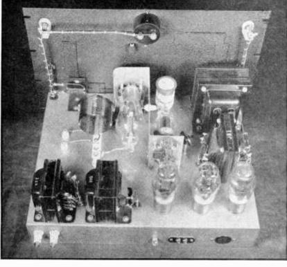
Figure 20. INTERIOR CONSTRUCTION OF 150-WATT TRANSMITTER. The location and function of the various parts are covered in the text.
