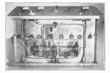
Figure 15. UNDER-CHASSIS VIEW OF MULTI-BAND FRE-QUENCY MULTIPLIER. Auto radio antenna couplers are used for making link connections in and out of the unit. Either shielded solid conductor or twisted hookup wire may be used for the link coupling line.
