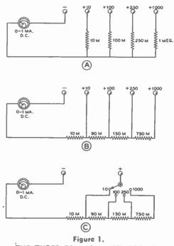
THE THREE COMMON METHODS FOR WIRING A MULTI-VOLTMETER.
