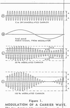
The top drawing (A) represents a continuous carrier wave; (B) shows the audio signal output from the modulator. (C) shows the audio signal impressed upon the carrier to the extent of 50 per cent modulation, and (D) shows the carrier with 100 per cent modulation. These drawings illustrate the mechanics of amplitude modulation.
