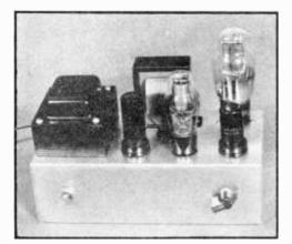
Figure 13. VOLTAGE REGULATED POWER SUPPLY.
