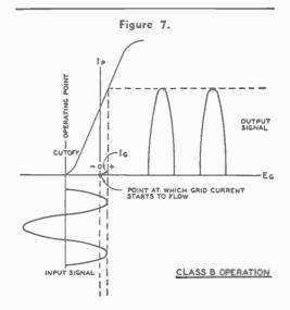
Because the plate current rises from a very low to a very high peak value on input swings in a class B audio amplifier, the demands upon the power supply are quite severe; a power supply for class B amplifier service must have good *regulation*. A high-capacitance output capacitor must be used in the filter circuit to give sufficient storage to supply power for the stronger audio peaks, and a choke-input filter system is required for good regulation.
