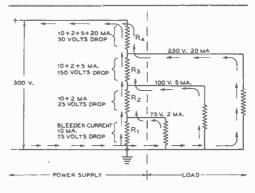
Figure 8. COMBINED BLEEDER RESISTOR AND VOLTAGE DIVIDER.
