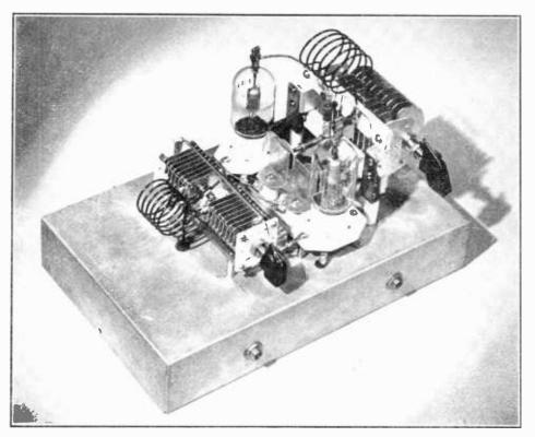
Figure 18. 125-WATT 50-MC. AMPLIFIER. Extreme simplicity characterizes this 50-Mc, amplifier stage. The neutralizing capacitors may be seen between the tubes. All components with the exception of the grid resistor are above the chassis.
