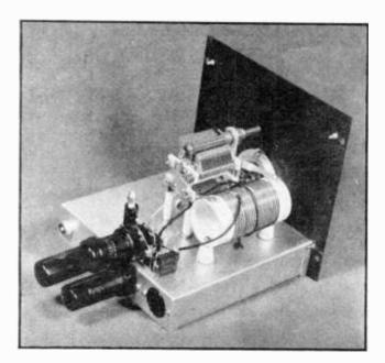
Figure 6. INTERIOR CONSTRUCTION OF 160 METER V.F.O. All parts of the oscillator circuit are made very riaid. The con-
