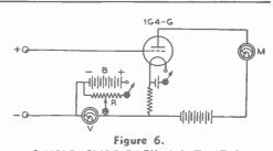
SIMPLE SLIDE-BACK VOLTMETER. By connecting a variable source of voltage in series with the input to the simple meter shown in Figure 5, a slide-back a.c. voltmeter for peak voltage measurements is made. The resistor R should be about 1000 ohms per volt at battery B.
