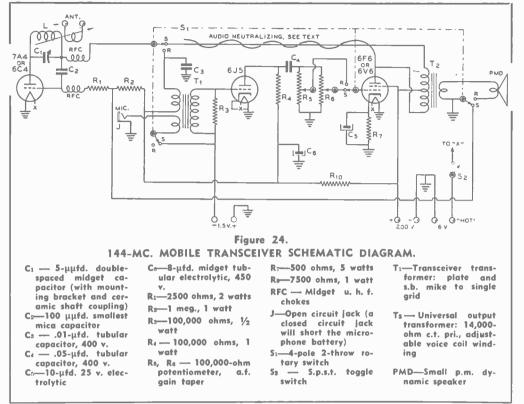
The layout is substantially the same as that for the receiver, illustrated in Figure 18, and therefore is not shown here. Also, the remarks pertaining to the r.f. portion of the circuit, including tank coil, tuning capacitor, and adjustable antenna coil, apply to the transceiver. This unit may be made in midget size.
