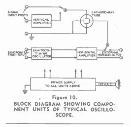
the accelerating anode potentials used with the larger tubes are high enough to be very dangerous, and also that the fluorescent screen can be damaged permanently by allowing the beam to rest for long on a single spot unless the intensity control is reduced sufficiently to prevent excessive brilliance.
