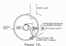
TUNING ARRANGEMENT. The tuning shaft is turned by means of a small knob, and a cable around the shaft drives an indicator which is provided with a large pulley as described in the text.
