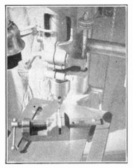
Figure 5. DRILL PRESS VISE. Small abjects are best handled on a drill press by means of a drill press vise.
