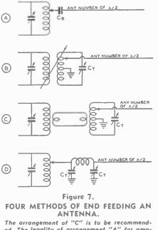
The arrangement of "C" is to be recommended. The legality of arrangement "A" for amateur work is debatable if the blocking condenser is large. It is really a form of direct coupling, permitted by the regulations only when an untuned feed line is used.
