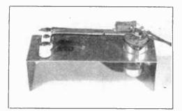
Figure 5. 2-WATT 220-MC. OSCILLATOR This simple and inexpensive oscillator may be used either as a low-power transmitter on the 220-Mc band or, by a slight circuit alteration, as a 220-Mc. band superregenerative receiver.
