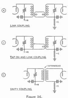
Figure 36. Twa types of link (inductive) coupling and (C) unity coupling.
