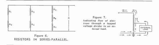
Shunts When a voltage is applied to a circuit consisting of two or more resistances in parallel the resulting current divides itself among the paths in inverse proportion to the resistance of each path. With respect to one of the elements those connected in parallel with it are said to *shunt* it.
