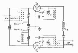
Figure 11-B. SIMPLIFIED SCHEMATICS OF "HIGH EFFICIENCY" LOW LEVEL MODULAT-ED STAGE.
