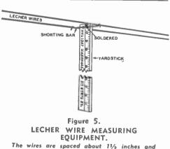
The wires are spaced about 11/2 inches and pulled taut. "Bumps" will appear exactly 1/2 wavelength apart on the wires as the jumper is slid along. The wires may be coupled to the oscillator under measurement by means of twisted line.
