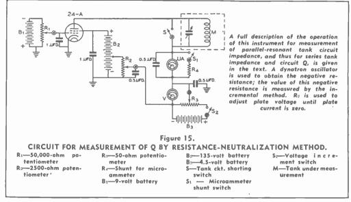
measurement of impedances of the values usually used in audio and low radio frequency work.
