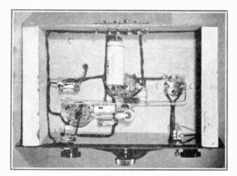
Figure 4. UNDER - CHASSIS VIEW OF 2-TUBE AUTODYNE. The construction of the chassis and placement of components is clearly illustrated. If desired the phone lack may be mounted on the back of the chassis. heaters are turned off by turning off the 110volt supply to the filament transformer.
