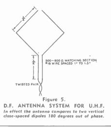
more sensitive than a conventional loop antenna at u.h.f., and is, therefore, to be preferred. The whole array can be supported from a pole having a single cross arm, which can be made removable to make the array collapsible.
