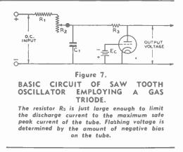
tive plate voltage is 7 or 8 times the negative grid bias voltage, assuming that the plate voltage is higher than the de-ionization voltage of approximately 16 volts. The basic gas-triode oscillator circuit is shown in Figure 7.
