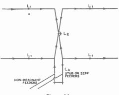
Figure 11. THE POPULAR "LAZY H" BI-DIREC-TIONAL ARRAY. Stacking the colinear elements results in both vertical and horizontal directivity.
