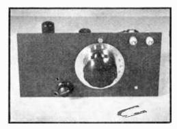
Figure 3. SIMPLE RECEIVER FOR USE BETWEEN 112 and 350 MC. The set is a superregenerator with a 9002 oscillator and plug-in inductances. The "coil" in the foreground is for 224 Mc.
