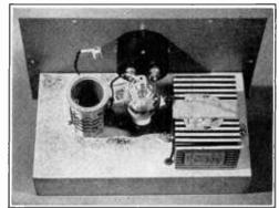
Figure 29. REAR VIEW OF SENSITIVE FIELD STRENGTH METER.
