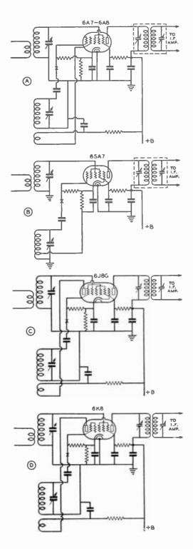
The different oscillator circuits shown in Figure 8 are not necessarily limited to use with the mixers with which they happen to be shown. Almost any oscillator arrangement may be used with a particular mixer circuit. Examples of some of the possible combinations will be found in Chapter 6.
