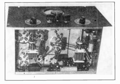
Figure 10. SHOWING FRONT PANEL AND UNDER-SIDE OF CHASSIS. Most of the "works" are under the chassis. The two ganged r.f. and mixer tuning capacitors are visible in this photograph, as is the oscillator band-setting capacitor.
