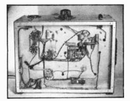
Figure 8. UNDER-CHASSIS VIEW OF 25-Watt V.F.O.
