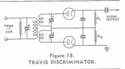
termediate (and discriminator) frequency is increased, the peaks must be separated farther to secure good linearity and output. Within limits, as the diode load resistors or the Q are reduced, the linearity improves, and the separation between the peaks must be greater.
