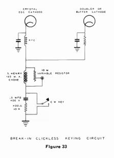
Two 6L6 or 6L6G tubes can be keyed very effectively with this type of circuit. The choke coil, shunted with a semi-variable resistor, provides a series inductance for slowing down the application of cathode current to the two tubes. The inductance of the choke coil can be effectively lowered to one or two henrys by shunting it with a
