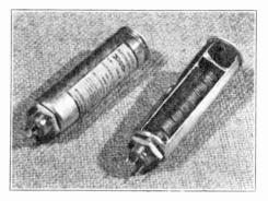
Figure 12—Newer Form of Electrolytic Condenser with a Bank of Electrodes, Rather Than a Foll-Coated Layer.
