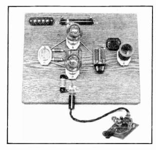
Figure 2—The Transmitter, Ready for Connection to Power Supply and Antenna.
