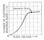
Figure 1- Curve showing emission from a cathode
