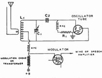
Figure 1-Self-Excited Modulated Oscillator.
