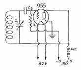
Figure 11—RCA 955-Circuit Diagram and Suggested Layout.
