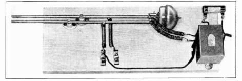
Figure 14-W.E.-316A ¼-Meter Oscillator.
