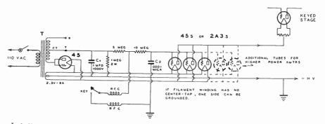
T- PLATE AND FILAMENT TRANSFORMER "Y" IS THE NORMAL TAP FOR REYING MEDIUM POWER TRANSWITTERS AND USE J25V EACH SIDE CENTER TAP "A" (ENTIRE SECONDARY) FOR HIGH POWER TRANSWITTERS
