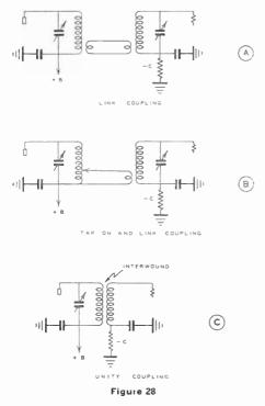
In .1 of figure 28, there is an impedance step-down from the primary coil to the link circuit. This means that the line which connects the two links or loops will have a low impedance and can, therefore, be carried over a considerable distance without introduction of appreciable loss. A similar link or loop is at the output end of the line; this loop is coupled to the grid tank of the driven stage.
