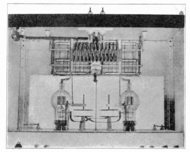
Figure 29—The high power modulated amplifier uses 250-TH's in push-pull.
