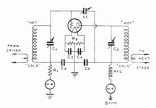
Figure 20—Link coupling between single-ended stages
