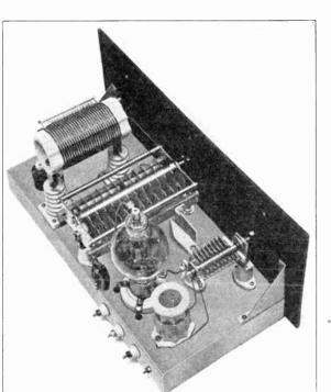
Figure 30 - Medium High-Power, Controlled Regeneration R.F. Amplifier with 100TH Triode. The Same Amplifier Design is Suitable for a Single RK-38, and, by Changing the **Tube Socket and Neutralizing** Condenser, for Such Tubes as the More Modern Versions of the "211," etc. The Neutralizing Condenser is Mounted with One of its Plates Attached to the Stator of the Plate Condenser, the Other Neutralizing Plate "Floats" on a Plug and Jack, Secured to a Standoff Insulator.
