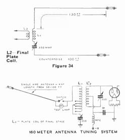
Figure 35—The circuit shows a tuning lamp in series with the antenna and a shorting switch for bridging the lamp after the antenna is tuned. Another method is to wrap a turn or two of the lead-in wire around a 2-turn loop connected to the lamp. The former system is best adapted for low power, the latter for medium or high power.
