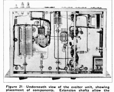
placement of components. Extension shafts allow the various condensers to be placed closer to their associated circuits.
