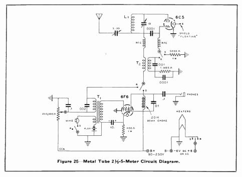
latter condition is sufficient to drive a small magnetic loudspeaker to moderate volume. The detector regeneration control can be set to a point of very low hiss level and high sensitivity.
