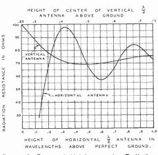
Figure 3—Effect of Height on the Radiation Resistance of a Dipole
