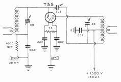
Figure 21—Single-Ended T-55 Amplifier as Pictured in Figure 20.
