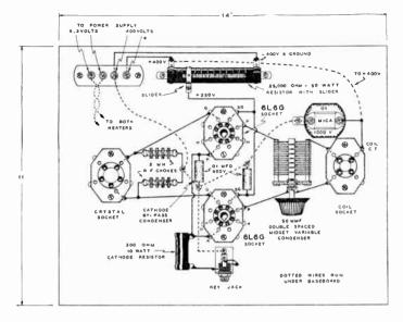
Figure 4—Pictorial Wiring Diagram, Showing Placement of Parts on the Baseboard.
