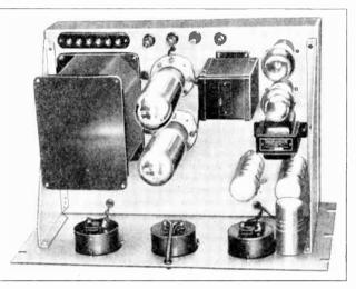
Figure 1— Relay Rack and Chassis for Mounting Heavy Modulator Components.
