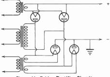
Figure 11-Bridge Rectifier Circuit
