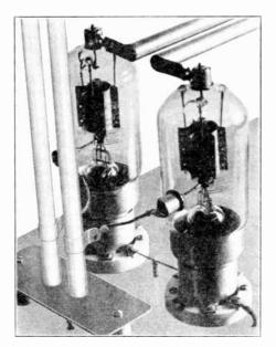
Figure 36—Parallel Rod U.H.F. Oscillator with HK-354C Gammatrons in Push-Pull. The circuit diagram\_is shown in figure 37.
