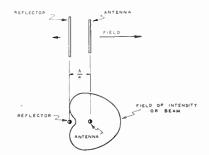
Figure 99—Directivity Pattern of Antenna Shown in Figure 98.
