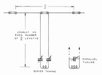
Figure 16-Center-Fed Zepp. Antenna.
