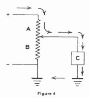
The device which secures current from the voltage divider is indicated as C. The current drawn by C flows through section Aof the bleeder resistor, then through C, and back to ground. The bleeder current, however, flows through the entire divider, i.e., through both A and B. Therefore, it becomes apparent that when a tap-on point is chosen to give the voltage desired, it is necessary to consider not only the current drawn by the device C, but also the bleeder current.
