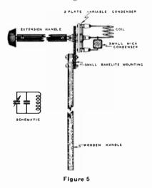
The turns can be squeezed in and out to "spot" the 5-meter band on the center of the condenser dial and the device then calibrated from known frequencies or Lecher wires. The coil can be wound with no. 10 wire in a winding length of 1-inch and with a diameter of about  $\frac{1}{2}$ -inch.
