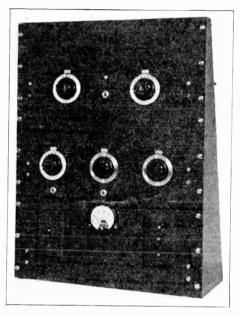
Figure 2—Front view of the inexpensive gridmodulated radiotelephone transmitter. It uses wall type on-off switches to control the power supplies. The Masonite panels are mounted on a wood rack. The two end pleces are ripped from one board by means of a single diagonal cut. Crackle paint gives both rack and panels the appearance of metal.
