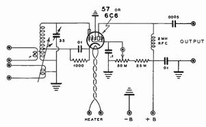
Figure 22—Wiring Diagram of the Regenerative Preselector.
