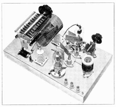
Figure 16—A Pair of 35T's, 800's, RK-35's or Other Tubes of Similar Type are Correctly Arranged in an R. F. Amplifier When the Placement is as Shown in This Illustration.
