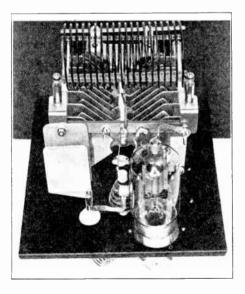
Figure 35—1-Kw. R. F. Amplifier with HK-364D Gammatron and New Atkins-Brown "Propeller-Type," Split-Stator Tuning Condenser. Note Extremely Short Connecting Leads.
