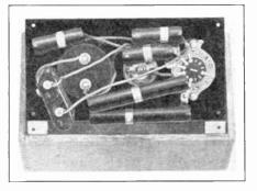
Figure 16—Interior View of Ohmmeter, Showing Battery, Rotary Switch and Ohmite Resistors.
