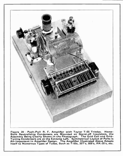
high output at low plate voltage when used as a neutralized amplifier.
