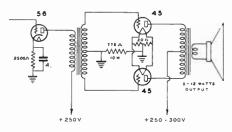
Low Distortion Audio Amplifier for Radio Receivers
