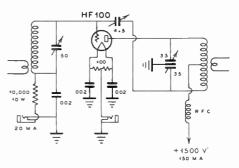
Figure 25—HF-100 Triode Amplifier. Figure 24 Shows its Mechanical Construction.
