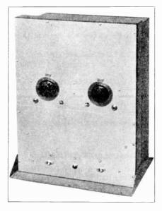
Figure 6—Front View of Housing for a Small Transmitter or High-Power Exciter. The Two Dial Lights for Tuning are Clearly Seen Between the Tuning Dials. These Dial Lights Obviate the Need of a Milliammeter.
