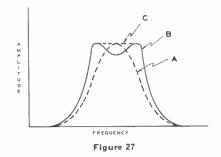
coupling is adjusted to such a value as to reduce the peak of the curve to a virtual flat-top, with no dip in the center as in B.
