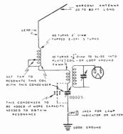
Figure 31—Loading System for Short Marcon i Antenna for Boats, Aeropianes, Etc.
