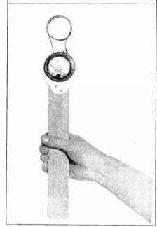
Figure 13—"Standing Wave Detector" and Field Strength Meter. The Device is Moved Along the Feeder or Antenna, Held Close to the Wire in the Same Relative Position. A Variation of Current Denotes Standing Waves.
