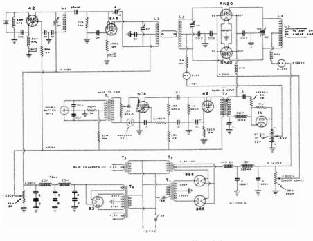
SUPPRESSOR MODULATED - CONTROLLED CARRIER PHONE
