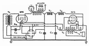
S. SCHEMATIC DIAGRAM OF POWER AMPLIFIER e AND POWER-SUPPLY UNIT
