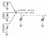
Figure 27-Tuned Circuits for Coil Switching
