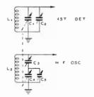
Figure 25-Front-End of Superheterodyne.
