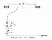
Figure 29-40-Meter Single-Wire-Fed Hertz for 160-Meter Operation. If "L" has sufficient turns, C1 is not required. "L" is coupled to the plate tank circuit.
