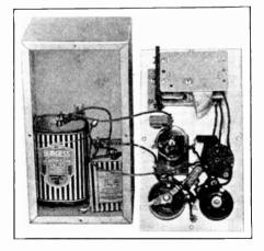
Figure 18—Interior View of All-Wave Test Signal Generator, Showing Type 30 Tube, Dry Cells, Condensers and Resistors.
