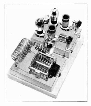
Figure 32-Oscillator, Oscillator-Doubler, Buffer and R. F. Amplifier Combination with 6A6 Twin - Triode, a 6L6G Doubler or Buffer Amplifier and a T-55 Triode in the Buffer-Driver Amplifier. An Ideal Medium Power Amateur Transmitter in Itself. It Can be Used as a Driver for the High-Powe Amplifier Shown in Figure 33. The T-55 Amplifier is Mounted on a Separate Small Metal Chassis. The Design of the Oscillator and Doubler is Given in the Chapter on Transmitter Frequency Control.
