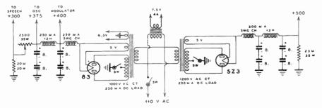
Figure 5—Two Power Supplies Provide All Necessary Power for the Transmitter.
