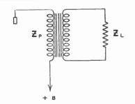
Figure 29—The reflected impedance ZP varies directly in proportion to ZL and the square of the turns ratio
