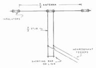
Figure 19—Center-Fed Half-Wave Antenna with Half-Wave Matching Stub.
