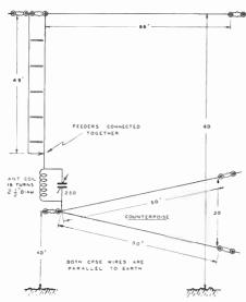
Figure 28—160 Meter Operation From a 40-Meter Zepp. Antenna. Where space is limited, the 40meter zepp.-fed Hertz antenna illustrated above will give satisfactory operation on 160 meters. The zepp. feeders are connected together at the station end and attached to one side of the tuning condenser and coil, as shown in the diagram. The remaining ends of the coil and condenser connect to the counterpoise.
