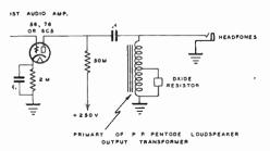
Figure 21-Automatic Noise Limiter Circuit.
