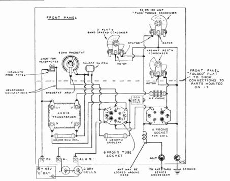
Figure 4—Pictorial Wiring Plan for Type-19 Twin-Triode Regenerative Receiver.
