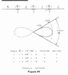
Two half waves *in-phase* will give a gain of approximately 2.5 db with respect to a single half-wave antenna; three sections will give a gain of approximately 4 db. Additional half-wave sections increase this power gain approximately one db. per section.
