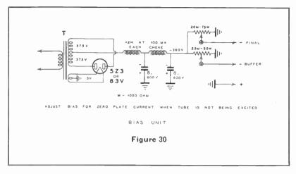
The value of C-bias depends upon the secondary voltage of the transformer and whether condenser or choke input to the filter is used.
