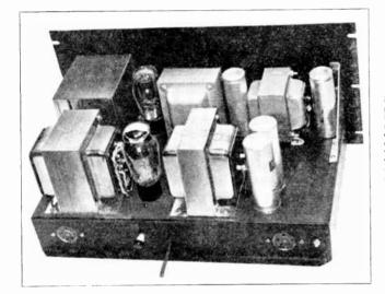
Figure 33—Dual-power supply for crystal oscillator, buffer-doubler and speech amplifier service. The unit closest to the front panel delivers from 350 to 400 volts, the other is a 600-volt supply for a huffer stage. Bleeder resistors are under the chassls. Wafer sockets are for plug-in terminals and cords.
