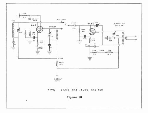
can be made to operate, and also because it will work with 80 and 40 meter crystals that do not show high activity.
