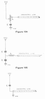
Figure 106 Concentric Feeder Systems for Broadcast Antennas with Various Terminations
