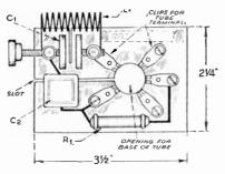
Figure 12-Plan view of transmitter.
