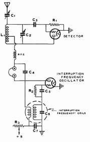
Figure 3—U. H. F. Receiver Circuit with Separate Oscillator.
