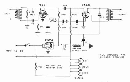
A.c.-d.c. amplifier circuit suitable for any intercommunicating system, either the simple "talk-back" type or the more elaborate, multi-station selective type system.
