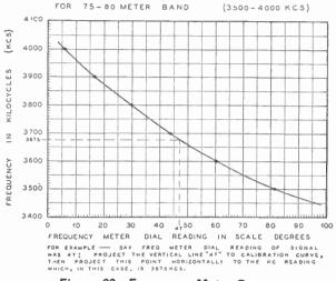
Figure 22-Frequency Meter Curve.
