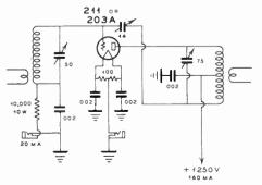
Figure 15-Circuit for 211 Amplifier Pictured in Figure 14.
