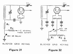
In figure 31,  $R_1$  is the usual grid-leak. Additional fixed bias is applied through a 100,000 ohm resistor  $R_2$  to block the grid current and reduce the output to zero. As a general rule, a small 300 to 400 volt power supply with the positive side connected to ground can be used for the additional C-bias supply.
