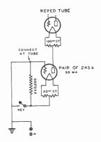
Figure 36—Vacuum Tube Keying. The circuit shows one of the more simple vacuum tube keying circuits. Some current flows through the key and this system sometimes produces clicks when the key is opened. Both filament transformers must be insulated from each other and also from ground. This circuit will not completely cut off the plate current to the keyed stage, but will reduce it to a very small value.
