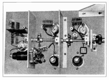
Figure 32—The Ganged High Frequency Circuits.
