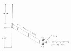
Figure 17–20- and 40-Meter Vertical Antenna with Zepp. Feeders. C1-C2 Are .00025  $\mu fd.$  Condensers.
