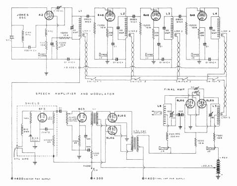
Figure 10—Typical Speech Amplifier Modulating a 50-Watt Class C Stage.
