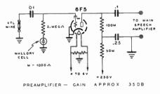
Figure 7—This pre-amplifier can be used with an inductive microphone by changing the resistance network in the input to a transformer of the correct design. If the pre-amplifier is far removed from the main speech amplifier, a plate-to-500ohm-line transformer should be connected in the output, with a corresponding 500 ohm-to-grid transformer at the speech amplifier.
