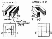
Figure 41—Types of Transformer Cores.
