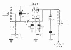
Figure 23—Single 35T Amplifier; Figure 22 Shows Its Construction.
