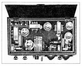
Figure 35-Looking into the High-Output Transmitter-Receiver.
