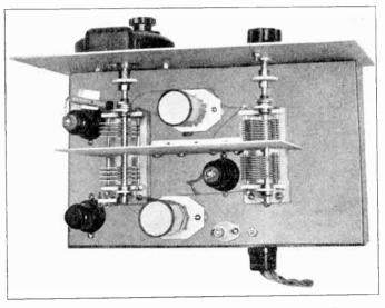
Figure 14—Interior view of the t.r.f. amateur type receiver. The receiver should preferably be housed in a metal container in order to reduce hum pickup.
