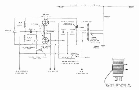
Figure 3—Schematic Circuit of Push-Pull 6L6G CW Transmitter and Pictorial Drafting of Plate Coil With Antenna Coupler.
