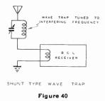
the Marconi type. If a Marconi antenna is to be used, a counterpoise, rather than a ground connection, will often minimize the interference in b.c. receivers.
