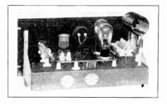
Figure 10—Final Amplifier with Two 210 Tubes in Push-Pull. The Tubes, Grid Coll and Neutralizing Condensers are Mounted on a Separate Masonite "Deck," Supported on Small Insulators.
