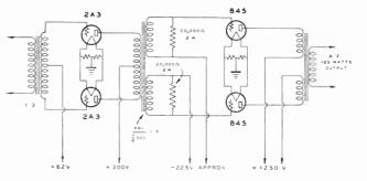
125-Watt Output Modulator with 845's in Push-Pull with Provision for Balancing Plate Current
