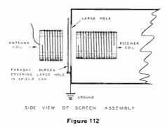
varnish. The wire is wound on, then a coating of insulating varnish is applied to the winding. After it has dried, one edge is trimmed with tin snips or heavy shears and the wires soldered together along the opposite edge as shown in the illustration.
