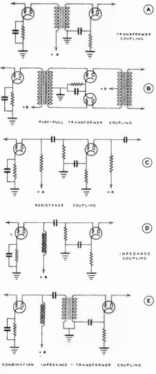
Figure 4 — Five Common Methods of A.F. Interstage Coupling.
