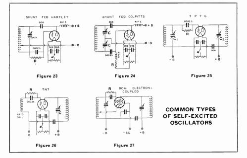
ating. R.f. chokes for operation on several harmonically-related bands must be designed carefully so that the impedance of the choke will be extremely high (several hundred thousand ohms) in each of the bands.
