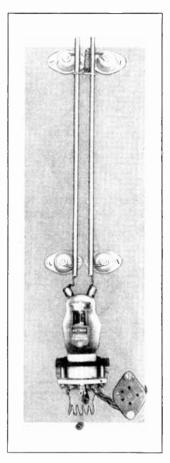
Figure 19—Raytheon RK-34 2½-Meter Oscillator.
