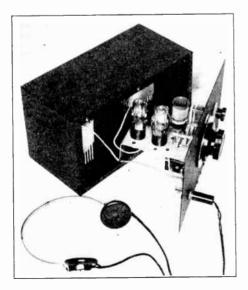
Figure 26—Illustrating Construction of the C. W. Monitor.
