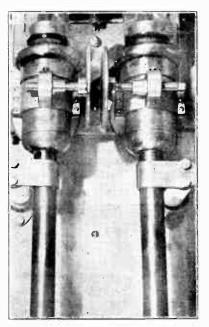
A 50-megacycle amplifier. Tank circuit is of the parallel-line type using a small disc condenser for fine tuning adjustment.
