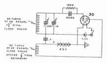
Figure 23—Calibration Oscillator for Battery Operation.
