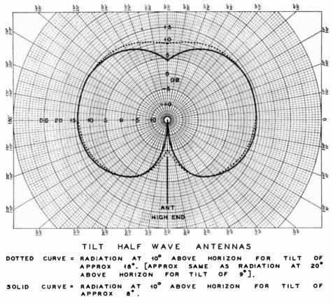
frequency is not always *exactly* the same, though for all practical purposes it may be considered the same, and a great reduction of signal is possible by having the proper amount of tilt for the particular frequency in use. The reason why a signal cannot be attenuated more than a few R points is that the incoming wave does not come in toward the antenna at just one angle, such as exactly 30°.
