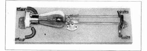
Figure 17-21/2-Meter Transmitter with RCA 834 U.H.F. Triode.
