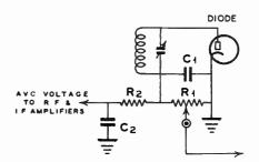
Figure 9--- Typical A.V.C. Circuit Using Diode
