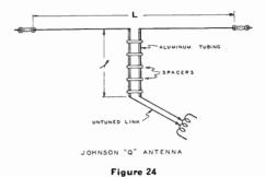
eter, spaced 1.6 inches apart, in order to obtain an impedance of about 200 ohms. This value is the geometric mean between the antenna center impedance of 73 ohms and the 600-ohm impedance of the two-wire nonresonant line. The matching "transformer" introduces a negligible loss and eliminates the fanned-out section of a two-wire matched impedance feed system, such as the one described in figure 12.
