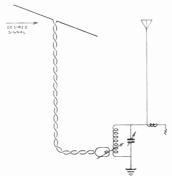
Figure 91-Tilt Bucking Antenna System.
