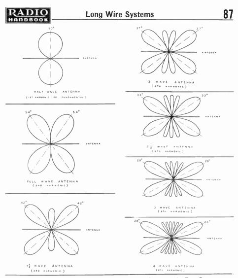
Figure 48—Radiation Patterns of Horizontal Antennas in Free Space. The presence of the earth makes the antenna less directional than indicated in the above patterns, particularly in the direction of the antenna wire.
