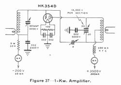
This new type condenser is incorporated in a high power amplifier illustrated in figure 35. A circuit diagram of the amplifier is shown in figure 37.
