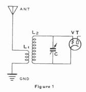
It will be recalled that the voltage induced across the coil is equal to the product of this current and the impedance of the coil. The *impedance* of the coil to the flow of current is made-up principally of its *reactance*. This is a function of the number
