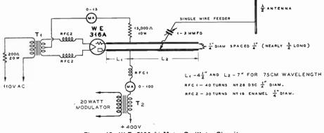
Figure 15-W.E.-316A ¾-Meter Oscillator Circuit.
