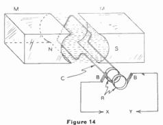
and if the opposite ends of conductor C are brought to collector rings, R, which are contacted by brushes, there will be a flow of alternating current when conductor C is rotated. This is the basic method of producing alternating current.
