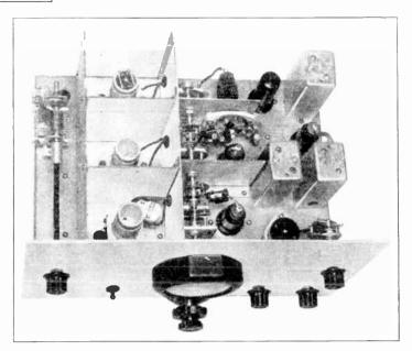
Figure 16—Illustrating assembly of the new "Ultra Gainer," showing antenna noise suppressor, shielded coll compartment (cover removed to show coils) and ganged condenser arrangement.
