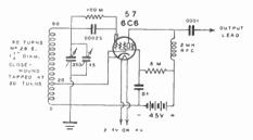
Figure 24—With Heater Type Tubes, Battery Plate Supply is Still Used for Stability.
