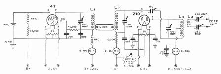
Figure 22—Complete Circuit Diagram of 47 Oscillator link coupled to 210 amplifier stage. One or two turns of wire are wound around coils L1 and L2 to form the coupling loop. The two loops are connected through a twisted-pair feed line, made with hook-up wire.
