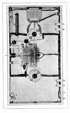
Figure 30—Under chassis view of the 250-TH amplifier, showing filament transformer, grid tank, etc.
