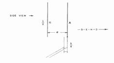
PARASITIC REFLECTOR  $\frac{\lambda}{4}$  in back of  $\frac{\lambda}{2}$  antenna gain approx 3 db. **Figure 66**
