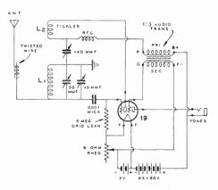
Figure 3—Schematic circuit diagram of the onetube receiver. L1 is the secondary, or grid coil. L2 is the "tickler," or regeneration coil.
