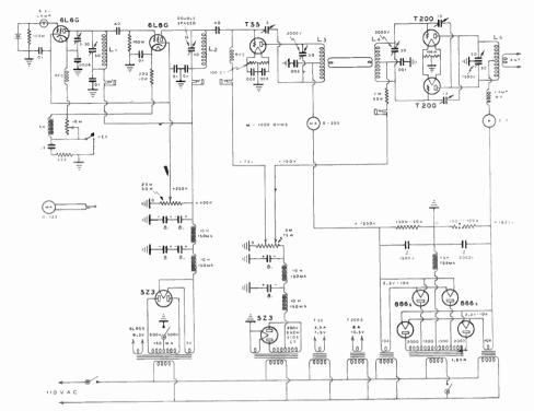
Figure 34—General Diagram of the Complete High Power Transmitter.
