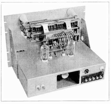
Figure 22—The 250-Watt 35-T Amplifier. This stage is either plate modulated or used to drive the high-power modulated amplifier. The plate tuning condenser is mounted parallel with the front panel to allow shorter leads, and is driven by cord and pulleys. 2
