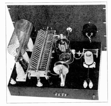
Figure 13 — The modulated final amplifier uses an HK-354C running class C. The grid tuning condenser is mounted parallel to the front panel; a flexible cable connects it to the dial on the front panel.
