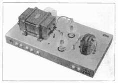
Figure 28-The 500 watt class B modulator unit.
