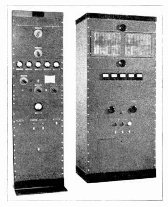
Figure 16—The 250 watt complete radiophone transmitter (left) and high power amplifier and modulator (right).
