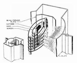
Figure 8-Internal Structure of Beam Power Tube
