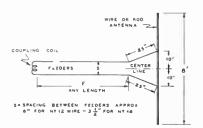
Figure 96—5-Meter Matched Impedance Antenna
