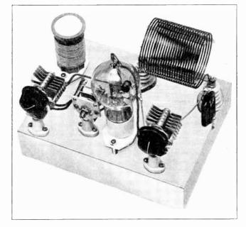
Figure 18-Standard Low-Cost Parts are Used in This Amplifier. The Tube is an RK - 35 Triode. Double-Spaced 50 µµfd. Midget Variable Condensers Tune Both the Grid and Plate Circuits. Neutralizing Condenser is a Standard 4-µµfd+ Wide-Spaced Midget. When Mounted Behind a Metal Relay-Rack Panel, Condenser Shafts Should be Fitted with Insulated Couplings.
