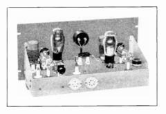
Figure 9-6L6G Exciter and 210 Buffer-Doubler.
