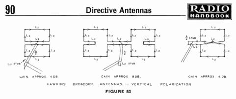
wave portion of an "H" section are bent over toward each other and connected together. This reduces the required vertical dimensions one-half. The reduction in gain due to cancellation of radiation in the bentover portion of the half-wave sections is not very great. The calculations of the designer give the approximate gains as shown in figure 53.
