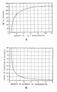
Figure 78-Diamond Antenna Design Chart.
