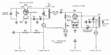
CRYSTAL OSCILLATOR - BUFFER - AMPLIFIER CIRCUIT
