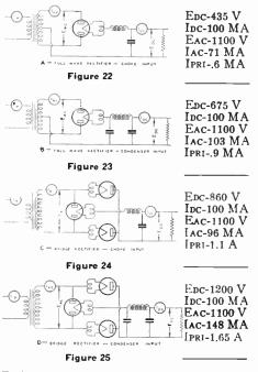
Typical voltage and current readings in various types of power supplies.
