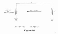
A very long wire of several wavelengths when terminated in a resistance equal to its characteristic impedance, becomes a "*Wave*" or "*Beverage*" antenna. This form of antenna is satisfactory for long-wave reception and is non-resonant.
