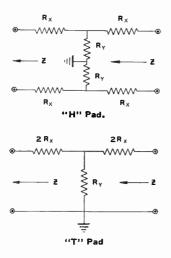
amount of input voltage available to excite amplifiers, thus precluding the possibilities of overloading certain components in the amplifying system. A resistive network which functions as an absorption device loses its identity as a "pad" and is most often referred to as an "insertion loss," because the section has been inserted to attenuate a known and definite quantity.
