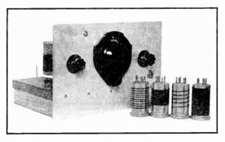
Figure 6—Front View of Receiver. Colls for All-Band Operation are to the Right.
