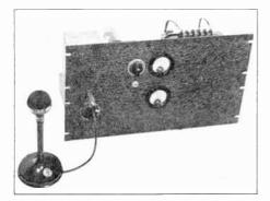
Figure 15—Front panel view of the speech amplifier and modulator unit.
