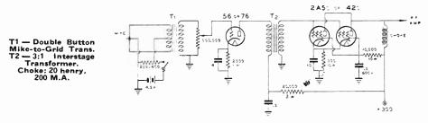
Figure 4—10-Watt Amplifier for Double-Button Microphone.
