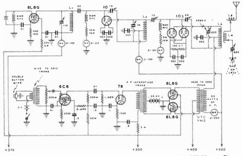
Figure 4—Radio Frequency Portion and Modulator of the 160-Meter Phone Transmitter.
