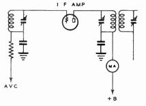
Figure 12—Circuit for Using Meter as Tuning Indicator.
