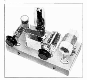
Figure 14 - The "Old Reliable" Type 211 or 203A Triode is Still Widely Used by Amateurs. The Amplifier Design is Ideal for Such Tubes. The Larger-Than-Usual Neutralizing Condenser is Easily Made from Aluminum, Bent as Shown in the Photograph, with One of the Sections Attached Directly to the Stator of the Plate - Tuning Condenser. Note How Well the Parts Lend Themselves to Symmetry in This Design.
