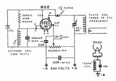
Figure 12-Reinartz 802 Oscillator Circuit
