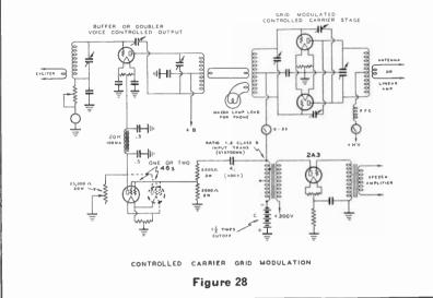
bias in the buffer r.f. tube. This change of bias varies the r.f. excitation to the gridmodulated r.f. amplifier. The latter operates in a manner similar to that of any other grid-modulated stage, except that the carrier output varies in accordance with the amplitude of the speech input.
