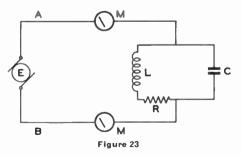
In this circuit, as contrasted with a circuit for series resonance, L (inductance) and C (capacitance) are connected in *parallel*, yet the *combination* can be considered to be in series with the remainder of the circuit. This combination of L and C, in
