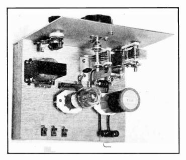
Figure 2—Rear View of the Dual Triode Receiver, Showing Layout of Parts.
