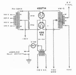
Figure 32—Wiring diagram for the high power modulator.
