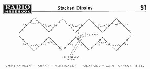
a half-wave matching stub or zepp. feeder of some multiple of half waves in length. If two bent wires are used as shown in the other Chireix-Mesny array, a quarter-wave matching stub can be connected across two points of high voltage.
