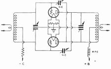
Figure 10-Push-pull r.f. amplifier stage
