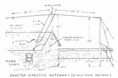
Figure 22—Pictorial of Figure 21, Showing Simplicity of 20-Meter Antenna Installation.
