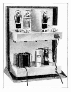
Figure 7—The Complete 6L6G Transmitter or High-Power Exciter, with Power Supply on the Lower Chassis. Five-Band Operation is Secured, with High Output for Either Direct Connection to an Antenna or Feeder System or as a Driver for a Medium Power R. F. Amplifier.
