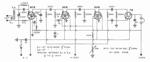
Figure 29-The Extremely Simple Circuit Diagram of the 5-Meter Resistance Coupled Super.
