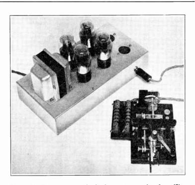
Figure 38—The vacuum tube keying system, using four 45's. Sockets for two additional (optional for higher power) tubes are provided. It is advantageous to mount the b. c. chokes directly at the key terminals, as shown.
