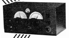
RME-69 SSS Receiver with built-in noise suppressor
