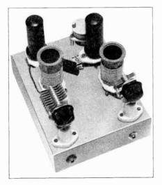
Figure 19—The Two Tube, 10 to 160 Meter 15-Watt Exciter
