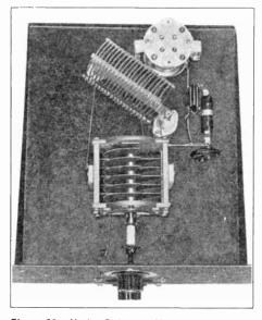
Figure 36—Under-Subpanel View of 1-Kw. R. F. Amplifier, Showing Grid Coll and Tuning Condenser, Method of Socket Mounting and Arrangement of Resistor and Bypass Condensers.
