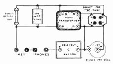
Figure 4—Pictorial Wiring Diagram of Code Practice Oscillator Shown Schematically in Figure 3.
