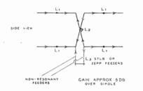
BROADSIDE ARRAY WITH HORIZONTAL POLARIZATION
