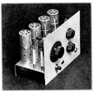
Figure 28—The Complete 5-Meter R-C Coupled Superheterodyne.
