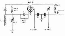
Figure 6 Tritet Crystal Oscillator
