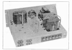
Figure 25-The 35-T class B modulator unit.
