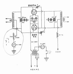
Figure 31—Schematic wiring diagram of the 1 kilowatt amplifier.
