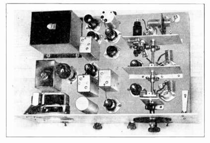
Figure 31-Top View, Showing Layout of Parts.
