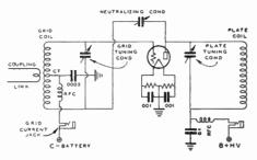
Figure 7-Grid neutralizing with series feed
