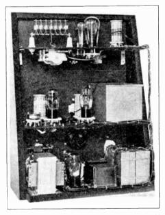
Figure 3—The continued popularity of the type 10 tube prompted the design of this grid-modulated transmitter. It will deliver a 30-35 watt carrier on phone, more on c.w. on the lower frequency bands.
