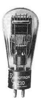
Grid bias for the type '10 may be obtained from a C-supply or by means of the voltage drop in a resistor connected in the negative plate return lead. The latter method is known as the self-biasing method, since the plate current determines the drop. It is not, however, generally applicable to battery-operated receivers.
