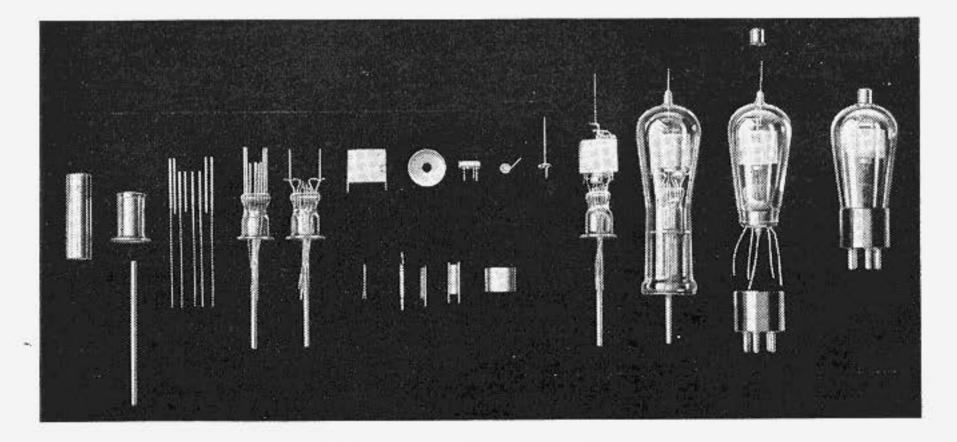
Parts Assembly of the '24-A
