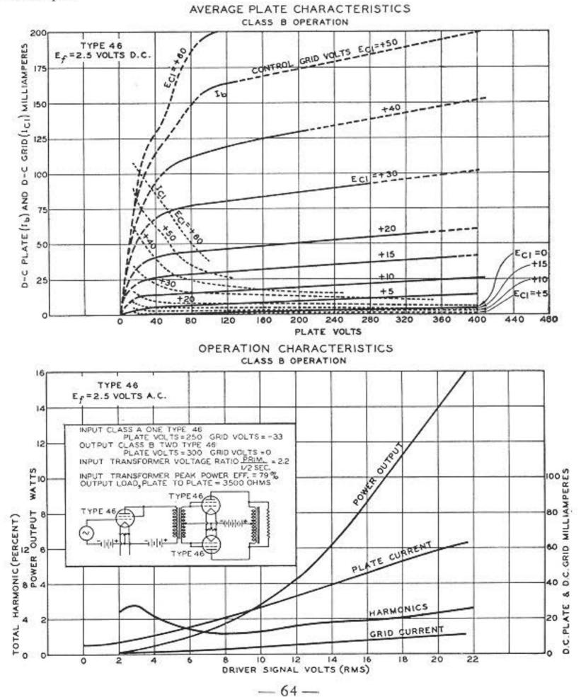
For Class A operation of the '46, the grid adjacent to the plate is connected to the plate. The grid next to the filament serves as the control grid. Operation of the tube is then similar to any Class A power amplifier triode. The operation of this tube connected as a Class A amplifier is not indicative of its performance in Class B circuits and should not be confused with the latter.
