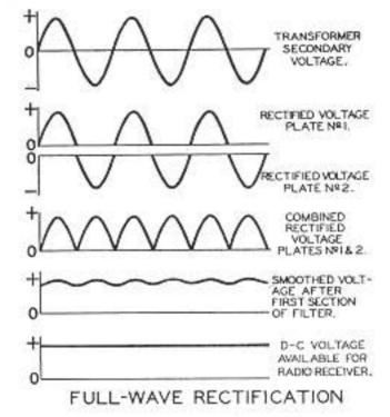
tube, current may be obtained on both halves of the a-c cycle. The '80 is an example of this type and is called a full-wave rectifier.
