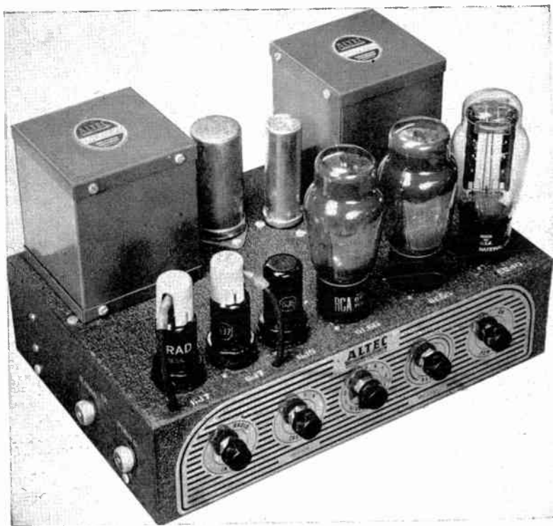
88. Assembly view of Altec Lansing 15-watt general-purpose amplifier. (Altec Lansing Corporation.)
