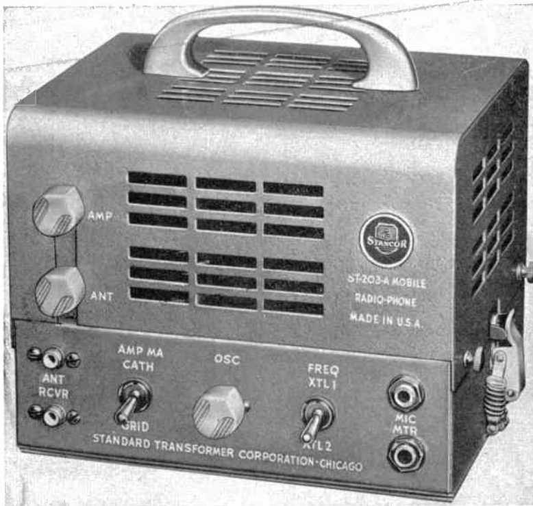
104. Assembly view of the Stancor ST-203-A radio transmitter with cover in place. (Standard Transformer Corporation.)
