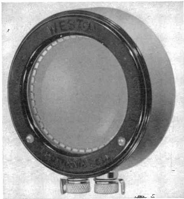
122. Weston Photronic Cell. ( Western Electrical Instrument Corporation. )
