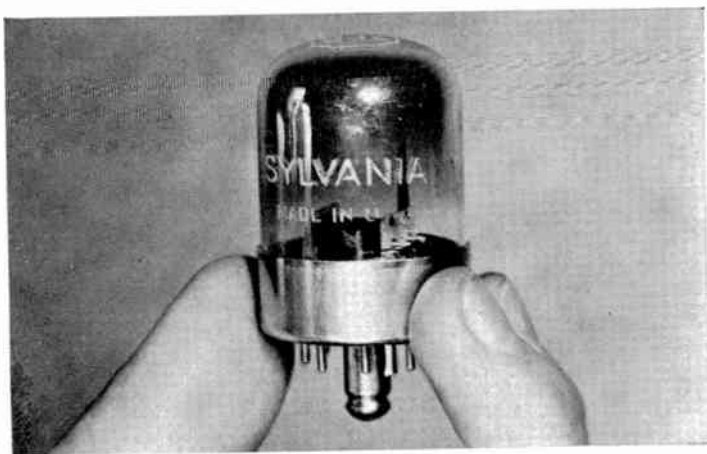
37. Type 7F8 multi-purpose high-frequency medium-mu twin-triode amplifier-oscillator with lock-in base. ( Sylvania Electric Products, Inc. )
