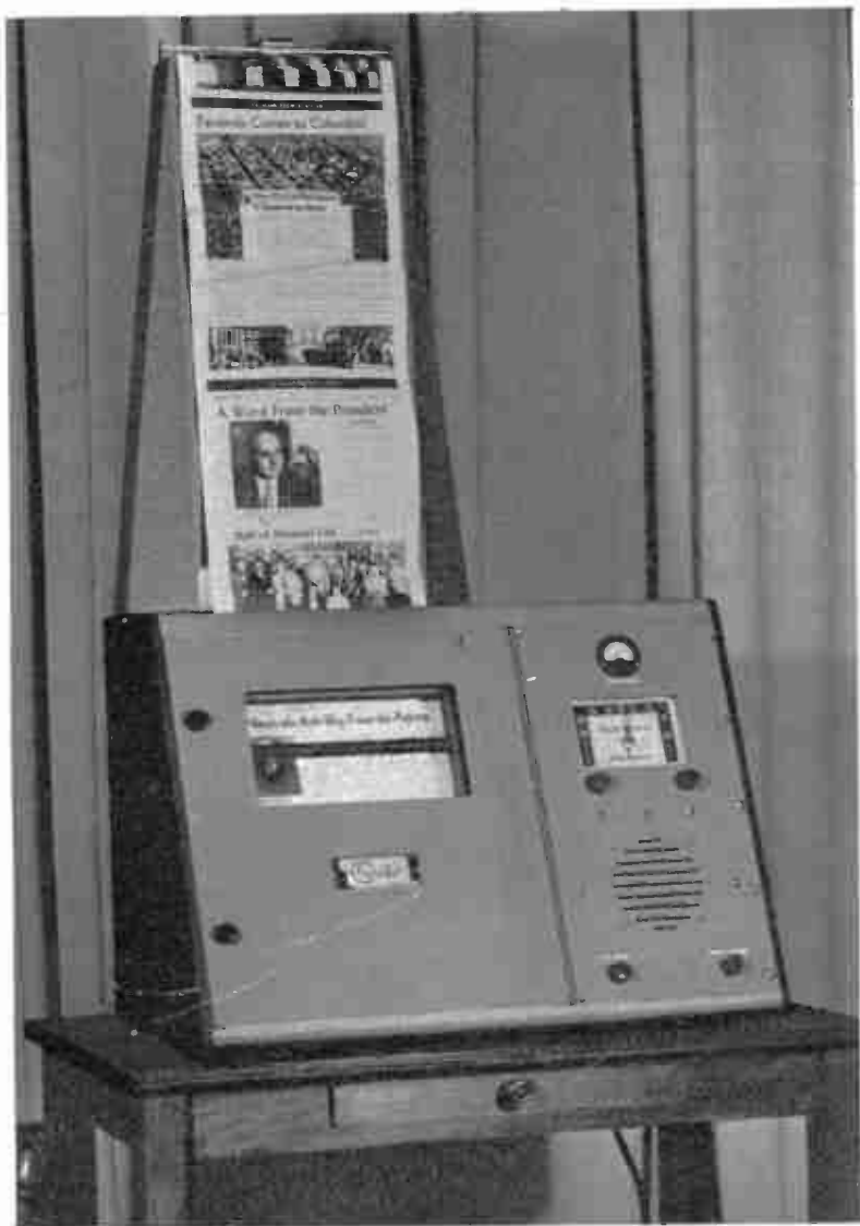
152. Table model of Hogan Faximile receiver manufactured by J. H. Bunnell Co. ( Radio Inventions, Inc. )
