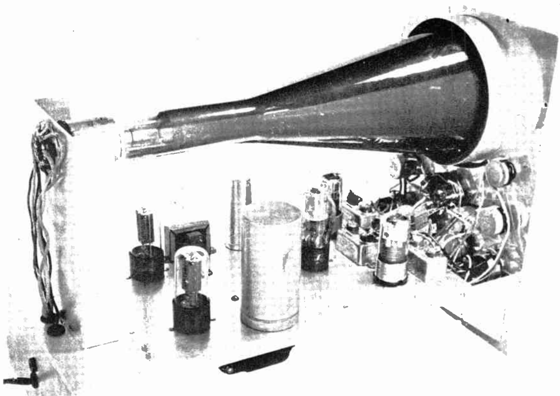
97. Assembly view of Eico oscilloscope, with cabinet removed. ( Electronic Instrument Co., Inc. )
