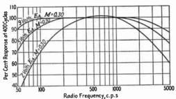
Fig. 6.—Fidelity as function of input voltage.
