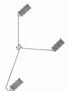
Fig. 53.—Antennas arranged for diversity reception.
