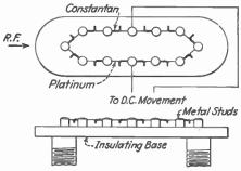
Fig. 6.—Galvanometer or bridge-type couple.
