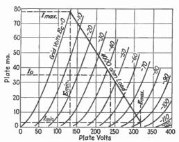
Fig. 4.—Load characteristics of a triode.
