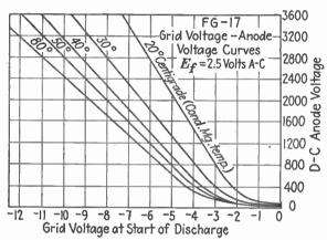
Fig. 19.—Typical mercury-vapor grid-controlled rectifier characteristics.
