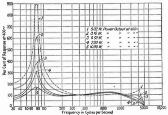
Fig. 14.—Variation of low-frequency response with volume.
