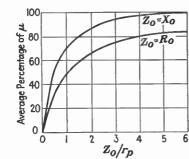
Fig. 2.—Voltage amplification of a triode.
