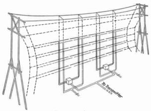
Fig. 42.—Telefunken directional antenna.
