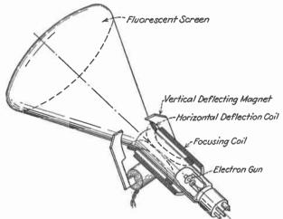
Fig. 6.—Oscillite tube and coil system.
