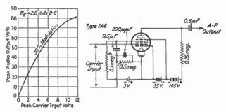
Fig. 19a.—Typical detection characteristics diode-tetrode.
