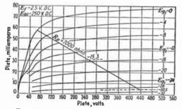
Fig. 23.—Load characteristic of 47 pentode.
