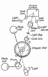
Fig. 8.—Balanced photocell optical system with chopper mirror and biasing C light.
