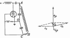
Fig. 45.—Colpitts circuit.
