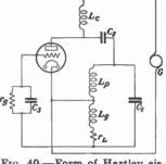
the voltage wave, but the average current thus passed is discharged at a uniform rate through the resistance, thereby providing a steady bias voltage.
