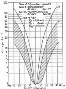
Fig. 22.—Iron-core coil characteristics.
