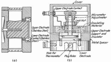
Fig. 17.—Types of crystal holders; (a) for ring plates, (b) holder with adjustable air gap.2
