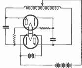
Fig. 36.—Symmetrical shortwave oscillator.
