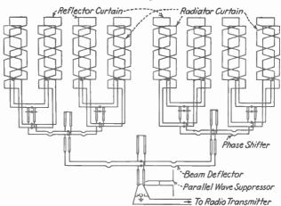
Fig. 46.—Barrage antenna of vertical radiators.
