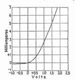
Fig. 2.—"Perikon" Crystal detector characteristic.
