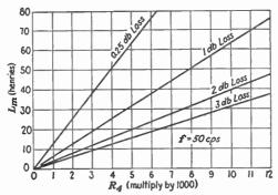
Fig. 19.—Loss at low frequency due to magnetising inductance.
