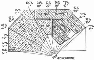
Fig. 38.—Velocity-microphone set-up for large orchestra group.
