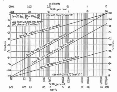
Fig. 6.—Relation of db to watts or volts.
