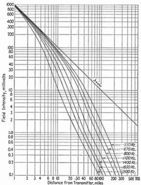
Fig. 74.—Field intensity at various distances from an antenna radiating an equivalent power of 1,000 millivolts at one mile over soil having conductivity of  $\sigma=60\times10^{-15}$  e.m.u. and an inductivity of  $\epsilon=15$  e.s.u.
