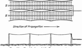
Fig. 52.—Double broadside Beverage antenna.
