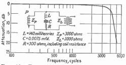
Fig. 12.—Transmission characteristic of scratch filter used with magnetic phonograph pick-up.
