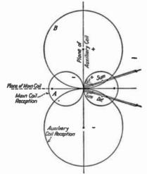
Fig. 16.—Crossed-coil direction-finding system.
