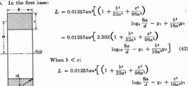
Fig. 24.—Multilayer coil.
