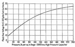
Fig. 12.—Flash-over voltage (60 cycles) of 2000 kva. capacitor.
