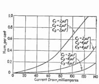
Fig. 13.—Percentage hum as a function of current drain.
