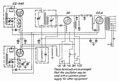
Fig. 29.—Beat frequency oscillator circuit. (RCA Manufacturing Company.)
