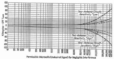
Fig. 7.—Two-carrier selectivity of 2,700- to 6,500-kc. receiver.
