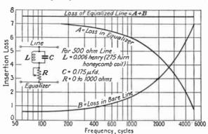
Fig. 30.—Attenuation equalizer for short cable circuits.
