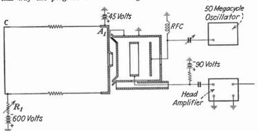
Fig. 4.—Circuit of image dissector—electron multiplier.
