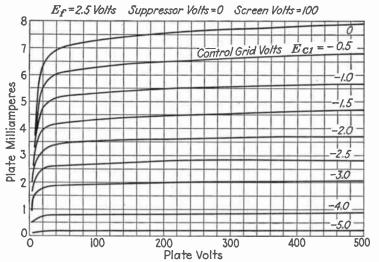
Fig. 28.—Average plate characteristics, type 57.
