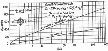
Fig. 68.—Impedance of parallel and concentric-tube lines.
