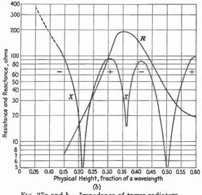
Fig. 27a and b.—Impedance of tower radiators.
