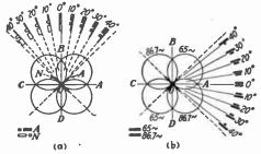
Fig. 20.—Transmitting characteristics of radio range-beacon antenna system.
