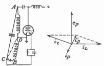
Fig. 44.—Effect of load resistance in Hartley circuit.
