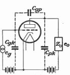
Fig. 3.—Triode amplifier showing interelectrode capacitances.
