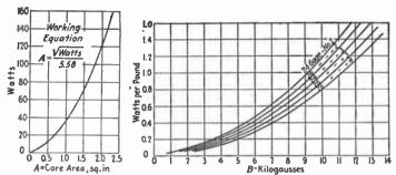
Fig. 31.—S m all power transformer core area as a function of watts.
