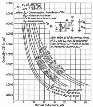
Fig. 73.—Values of M required for proper termination.
