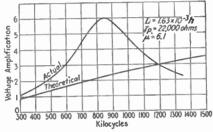
Fig. 4.—Amplification of a choke-coupled amplifier tube.
