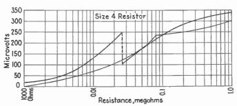
Fig. 7b.—Noise characteristics of smaller sized unit than in Fig. 7a.
