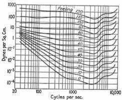
Fig. 4.—Relation between pressure in free wave and loudness for 10 db steps above threshold, observer facing sound source as given by Fletcher and Munson. (Jour. Acoustical Soc. America, 5, 91, 1933.)
