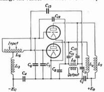
Fig. 61.—Equivalent parasitic circuit of Fig. 59.
