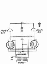
Fig. 7.—Balanced push-pull photocell amplifier.
