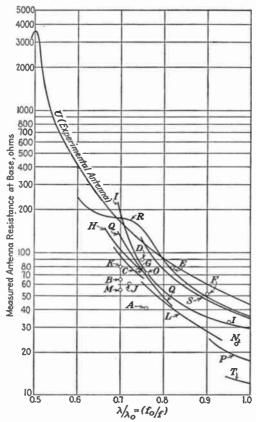
Fig. 26.—Base resistance of typical antennas.
