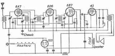
Fig. 43.-A-c-d-c receiver circuit.
