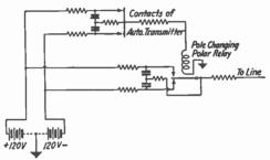
Fig. 11.—Double-current control circuits.
