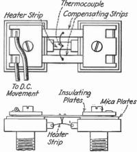
Fig. 7.—Compensated thermocouple.
