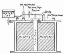
Fig. 13.—Ink recorder. Paper tape and tape guide not shown.
