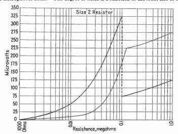
Fig. 7a.—Noise characteristics of carbon resistor.
