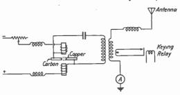
Fig. 3.—Arc transmitter.
