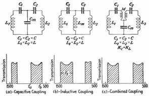
Fig. 24.—Coupled circuits as band-pass filters.
