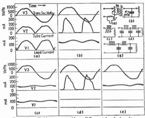
Fig. 20.—Half-wave rectifier, different load circuits.
