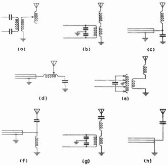
Fig. 28.—Antenna-tuning and transmission-line terminating systems.
