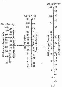
Fig. 34.—Transformer design chart based on  $E = \frac{BANf \times 4.44}{10^3}$ .
