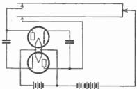
Fig. 37.—"Back-to-back" Lecher wire circuit.
