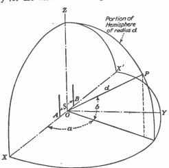
Fig. 20.—Geometry for calculating space characteristic of two-element array. acteristic in the upper half-space, for grounded antennas and perfectly conducting ground, is given in Fig. 20.
