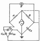
Fig. 48.—Measurement of direct capacitance.
