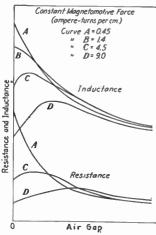
Fig. 18.—Effect of air gap on coil characteristics.
