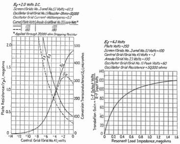
Fig. 33.—Characteristics of pentagrid converters 1C6, left; 6A7, right.
