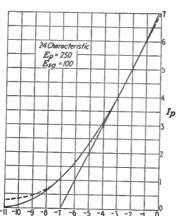
Fig. 7.—Hyperbolic detector characteristic.
