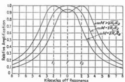
Fig. 17.—Response curves of doubly-tuned r-f stage.
