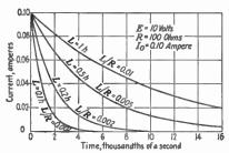
Fig. 2.—Fall of current in inductive circuit.
