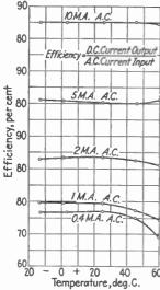
Fig. 13.—Ambient temperature-efficiency relation.
