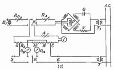
Fig. 33(c).—Drysdale potentiometer.
