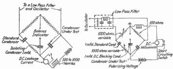
Fig. 10a.—Circuit for measuring Fig. 10b.—Capacity and power factor electrolytic condenser capacity.
