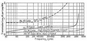
Fig. 28.—Transmission-loss characteristics of various audio-frequency circuits.
