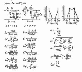
Examples of Filter Design: a. Single-section Filter. Required: High-pass single-section filter to be connected between resistance terminations of R=1,000 ohms, with a cut-off frequency of 1,000 cycles and maximum attenuation occurring at 800 cycles.
