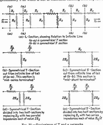
Fig. 35.—Equivalence of T and  $\pi$  networks.
