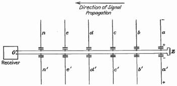
Fig. 51.-High-frequency Beverage antenna.
