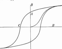
Fig. 6.—Typical B-H curve.
