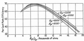
Fig. 55B.—Load curves for class B linear amplifier from which suitable adjustments may be selected.
