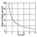
11.—Effect of  $C_1$  on ripple in output.
