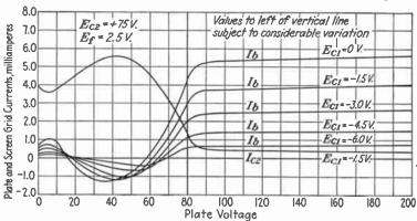
Fig. 27.—Type-24 screen-grid characteristics.
