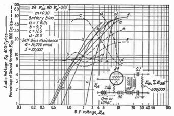
Fig. 17.—Screen-grid detector characteristics.
