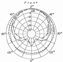
Fig. 20.—Directional characteristics of inductor microphone.
