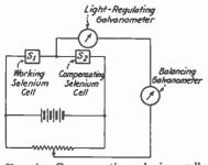
Fig. 4.—Compensating selenium cell lag. (Korn.)
