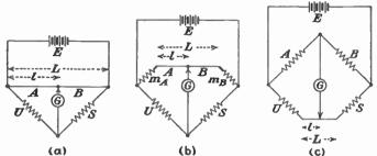
Fig. 37.—(a) Slide-wire bridge; (b) bridge with extension arms; (c) Carey Foster bridge.
