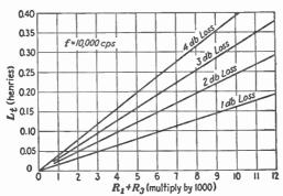
Fig. 20.—Loss at high frequency due to leakage inductance.
