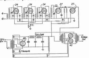
Fig. 26.—Typical t-r-f receiver.
