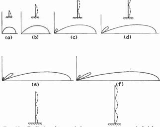
Fig. 23.—Radiation characteristic as antennas increase in height.
