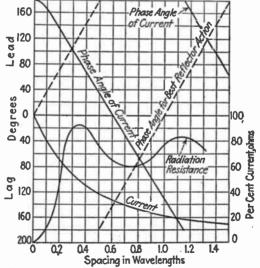
Fig. 12.—Conditions for array of parallel dipoles.
