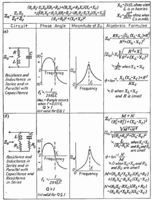
Equivalent impedance of parallel combinations of L, C, and R.
