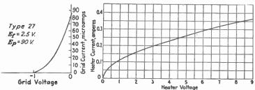
Fig. 10.—Grid-current gridvoltage characteristic.
