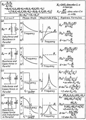
Equivalent impedance of parallel combinations of L, C, and R.
