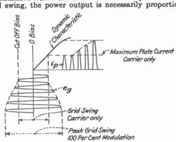
Fig. 55A.—Theoretical curves showing class B r-f amplifier operation.
