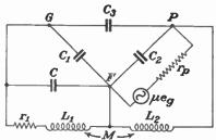
Fig. 5.—Capacities affecting oscillator action.
