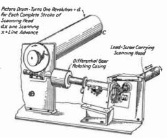
Fig. 3.—Cross-screen analyzing scanner.
