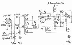
Fig. 23.—Broadcast transmitter power amplifier.
