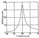
Fig. 3.—Resonance curve of vibration galvanometer.
