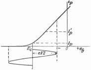
Fig. 25.—Vacuum-tube voltmeter characteristic.
