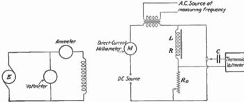
Fig. 10.—Circuit for measurement of inductance.
