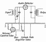
Fig. 17.—Automatic volume-control circuit.
