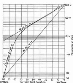
Fig. 12.—Advantage of special taper for volume control.
