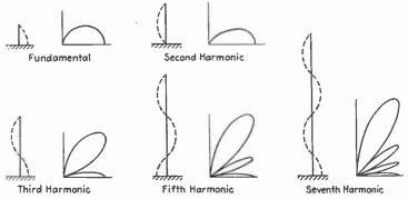
Fig. 16.—Vertical radiator over perfectly conducting ground.
