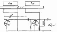
Fig. 24.--Magnetostriction oscillator.
