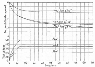
Fig. 5.—Voltage coefficient of carbon resistors.
