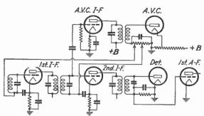
Fig. 21.—Amplified a.v.c. arrangement.
