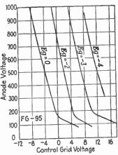
Fig. 20.—Characteristics of shieldgrid Thyratron.
