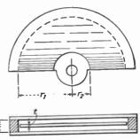
Fig. 13.—Dimensions useful in determining condenser capacity.
