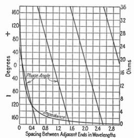
Fig. 11.—Mutual impedance of colinear half-wave dipoles.
