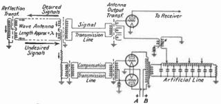
Fig. 8.—Wave antenna and output circuits.
