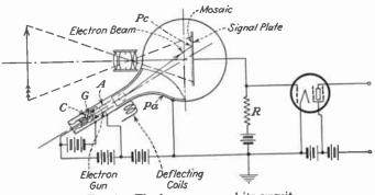
Fig. 2.—The iconoscope and its circuit.
