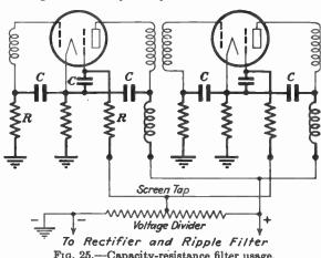
Fig. 25.—Capacity-resistance filter usage.
