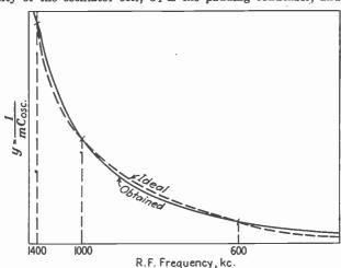
Fig. 15c.—Closeness of tracking secured by formulas.
