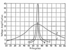
Fig. 5.—Amplification as a function of turn ratio.
