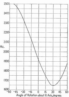
Fig. 15.—Frequency in kilocycles per millimeter thickness versus rotation about the X-axis (see Fig. 14).
