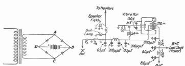
Fig. 29.—Bridge circuit for Rectox rectifier.
