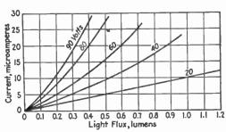
Fig. 18.—Typical emissive phototube characteristics.
