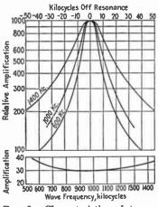
Fig. 5.—Characteristics of transformer in Fig. 4.
