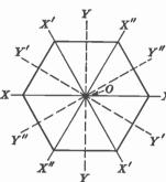
Fig. 12.—Quartz crystal cross section.
