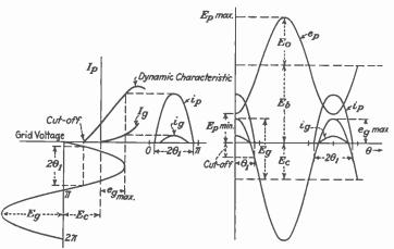
Fig. 28.—Instantaneous values of current and voltage in Class C amplifier.
