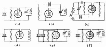
Fig. 18.—Representative oscillator circuits; (a) the most generally used circuit, (b) the Pierce circuit, (c) a high stability circuit (General Radio Company), (d) circuit employed in crystal calibrator—output exceptionally rich in harmonics, (e) Cady circuit adapted (J. R. Harrison) to four-electrode tube, (f) Hull space-charge grid circuit.
