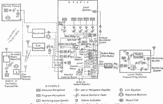
Fig. 1.—Schematic diagram of typical broadcast transmitting system.
