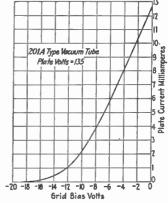
Fig. 3.—Characteristic suitable for detection.
