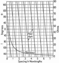
Fig. 9.—Mutual impedance for parallel dipoles.
