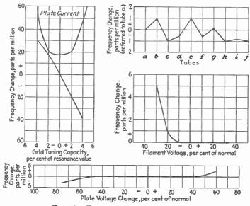
Fig. 19.—Frequency versus circuit variables.
