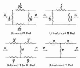
Z=Input Impedance = Output Impedance
