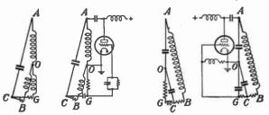
Fig. 47.—Hartley (left) and Colpitts (right) circuits.
