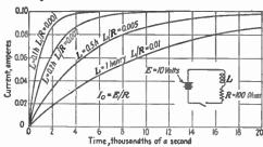
Fig. 1.-Rise of current in inductive circuit.
