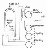
Fig. 15.—Fork control of shunt motor, d-c supply.
