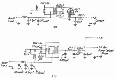
Fig. 40.—Vibrator B-supply systems.
