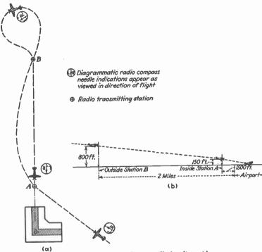
Fig. 27.—Army Air Corps radio landing aid.
