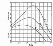
Fig. 17.—High-frequency characteristics of a transformer-coupled amplifier.
