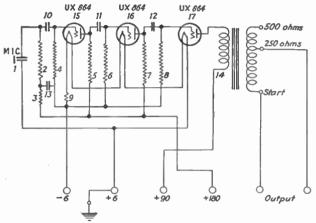
Fig. 26.—Amplifier for condenser microphone.
