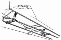
Fig. 55.—Under-car antenna for automobile radio.
