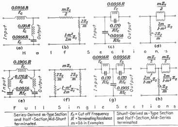
Fig. 37.—Half-section compared with full-section structures.
