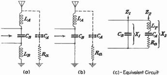
Fig. 70.—Terminations for transmission lines.
