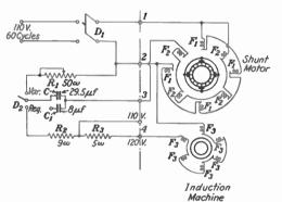
Fig. 12.—A-c projector-drive motor.
