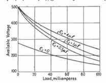
Fig. 10.—Effect of  $C_1$  on voltage available.
