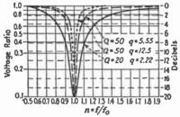
Fig. 28.—Filter cut-off characteristics.
