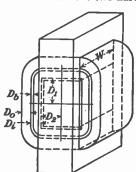
Fig. 14.—Simple winding scheme for a transformer.
