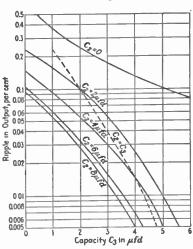
Fig. 12.—Percentage ripple as a function of  $C_2$  and  $C_3$ .
