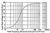
Fig. 22.—Automatic volume-control characteristic.
