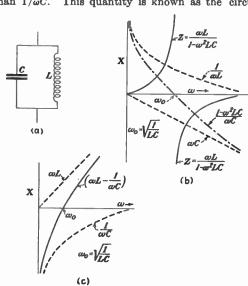
Fig. 4.—Reactance and impedance of parallel circuit.
