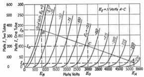
Fig. 52.—Method of determining modulator characteristics.
