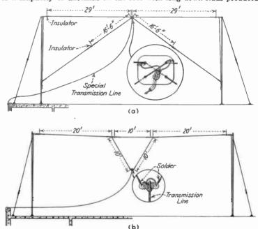
Fig. 54.—Types of all-wave receiving antennas.
