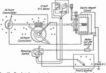
Fig. 10.—Preselected remote tuning arrangement for medium-frequency receiver.
