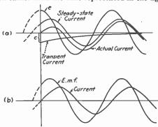
Fig. 8.—Effect on transient current of closing circuit at different times in the cycle.
