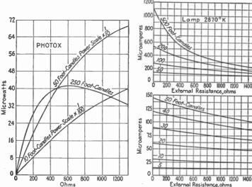
Fig. 15.—Characteristics of Westinghouse photox copper oxide lightsensitive cell.
