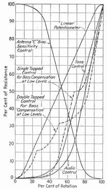
Fig. 11.—Taper curves of variable resistors.
