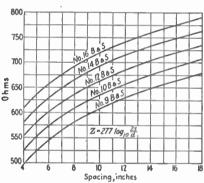
Fig. 33.—Characteristic impedance of open-wire r-f transmission line.
