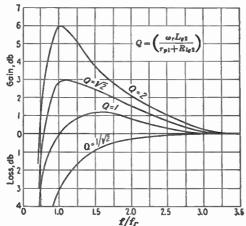
Fig. 12.—Low-frequency characteristic of a double impedance-capacitance coupled amplifier.
