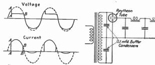
Fig. 26.—Voltage and current waves. Raytheon gaseous rectifier.
