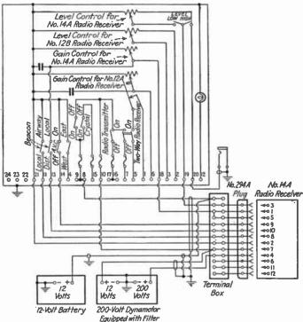
Fig. 13.—Control arrangement for airplane use.
