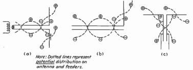
Fig. 35.—Voltage-feed systems (see text).
