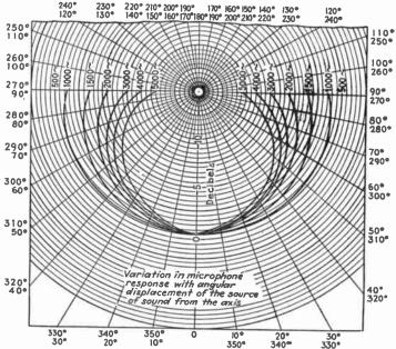
Fig. 30.—Directional characteristic of microphone.
