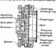
Fig. 22.—Condenser microphone.
