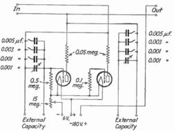
Fig. 31.—Generator of submultiple frequencies.
