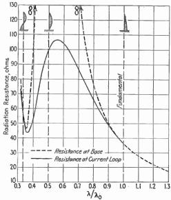
Fig. 8.—Radiation resistance of vertical grounded conductor.
