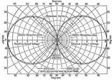
Fig. 9.—Directional characteristics of RCA velocity microphone.
