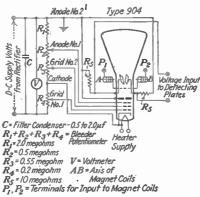
Fig. 7.—Cathode-ray tube control circuit.
