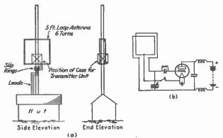
Fig. 19.—Transmitter for rotating beacon.
