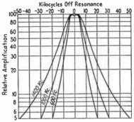
Fig. 7.—Selectivity characteristics of coupled tuned-circuit t-r-f transformer.
