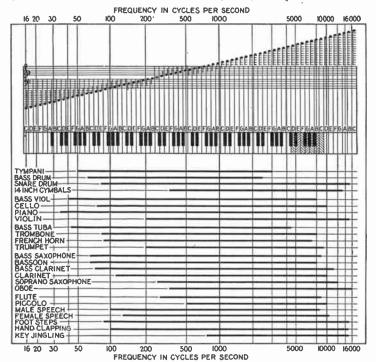
Fig. 3.—Frequency range required for the reproduction of musical instruments, voice, and noise without noticeable distortion.
