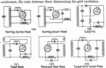
Fig. 7.—Fundamental oscillator circuits.
