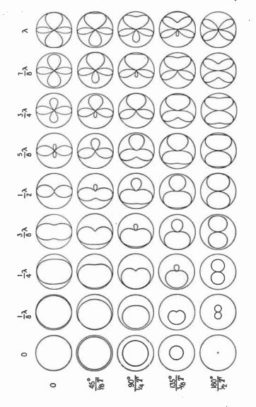
Fig. 18.—Directivity diagrams for radiator separations between 0 and 4 wave lengths and for various phase differences up to  $\frac{1}{2}T$ .
