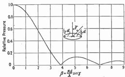
Fig. 10.—Directional radiation characteristics of vibrating disk in infinite
