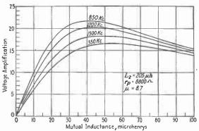
Fig. 9.—Effect of M on resonant amplification.
