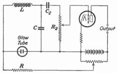
Fig. 34.—Circuit for glow-tube oscillator.
