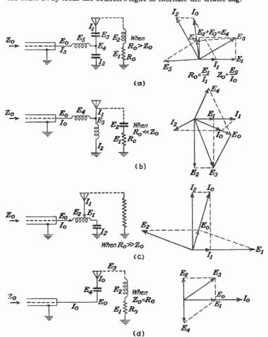
Fig. 31.—Concentric transmission-line terminations.
