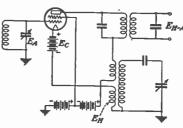
Fig. 21b.—Combined detector-oscillator circuit.
