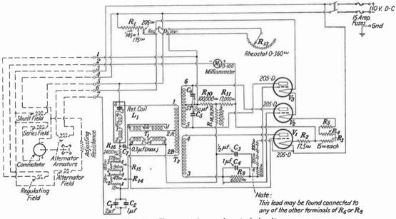
Fig. 11.—Vacuum-tube speed-control circuit.
