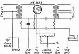
Fig. 13.—Schematic of microphone amplifier. (Western Electric 80A.)
