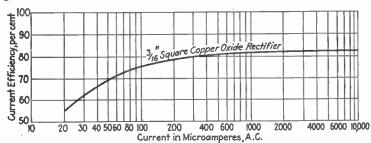
Fig. 10.—Current-efficiency characteristic.
