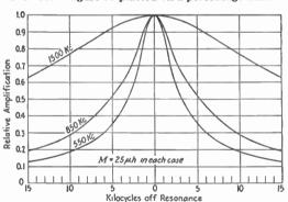
Fig. 12.—Selectivity as a function of frequency.
