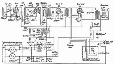
Fig. 37.—Superregenerator receiver for police cars.
