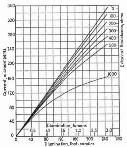
Fig. 17.—Weston Photronic cell characteristics.
