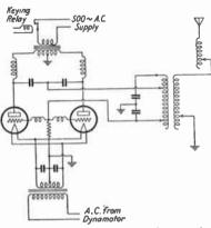
Fig. 6.—Essential circuit of icw marine transmitter with a-c plate supply.
