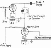
28. Transmitters for shipboard use Fig. 7.—Tube keyer for transmitter.
