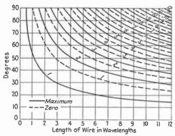
Fig. 15.—Angles at which maxima and minima in wave pattern occur.
