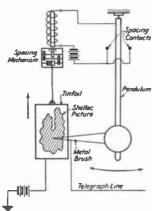
Fig. 2.—Alexander Bain's original picture apparatus (1843).
