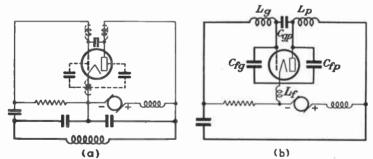
Fig. 38.—Colpitts high-frequency oscillator.
