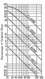
Fig. 9.—Filtering effected by resistance (ohms)-capacity (microfarads) circuit.
