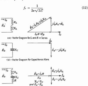
(c) - Vector Diagram for Condenser and Coil in Series
