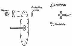
Fig. 1.—"Flying spot" method of scanning.
