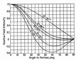
Fig. 22.—Effect of height on field intensity.
