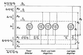
Fig. 2.—Parallel voltage divider.
