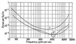
Fig. 2.—Threshold of audibility as given by Sivian and White (Jour. of Acoustical Soc. America, 4, 313, 1933). (1) In terms of pressure on ear drum for single ear; (2) in terms of pressure in free undisturbed sound wave, two ears, observer facing sound source; (3) in terms of pressure in free undisturbed sound wave, two ears, random horizontal incidence.
