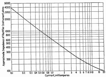
Fig. 11.-Impedance characteristic.
