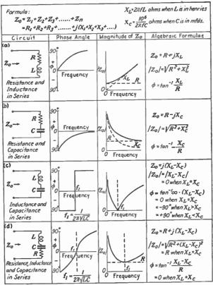
Equivalent impedances of series combinations of L, C, and R.
