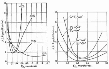
Fig. 16.—Tapped choke. Percentage of total turns (Fig. 15) used in  $L_1$ .
