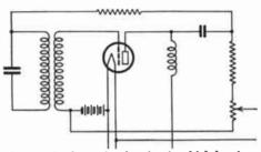
Fig. 27.—Fundamental schematic of a circuit which has been widely used for the generation of audio and carrier frequencies.
