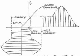
Fig. 25.—Characteristics of class B amplification.
