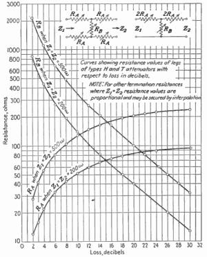
Fig. 40.—Chart for H and T attenuator design.
