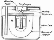
Fig. 18.—Cross section of RCA 50A inductor microphone.
