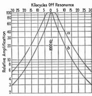
Fig. 6.—Selectivity comparison of single and coupled tuned circuits.
