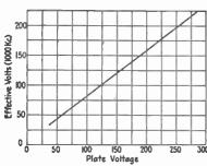
Fig. 27.—Voltage across tuned circuit as function of oscillator plate voltage.
