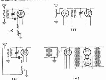
Fig. 10.—Typical uses of variable resistors.
