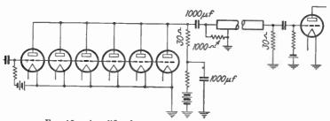
Fig. 10.—Amplifier for use with 1,500-ft. television line.
