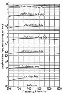
Fig. 29.—Voltage gain in superheterodyne receiver.
