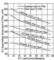
Fig. 23.—Output characteristics of Type 80 tube.
