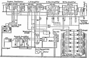
Fig. 50.—Circuit diagram of modern 50-kw transmitter.
