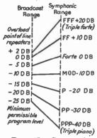
Fig. 45.—Compression of dynamic range in broadcasting system.
