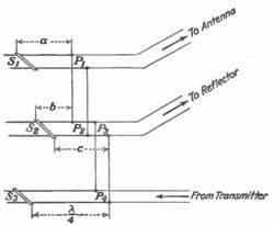
Fig. 48.—Transformer made up of transmission-line section.
