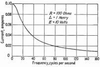
Fig. 7.—Current vs. frequency in inductive circuit.
