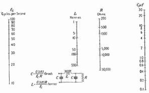
Fig. 6.—Low-pass filter design chart, Pi section.
