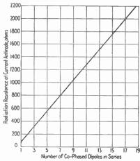
Fig. 7.—Radiation resistance in cophased dipole elements.
