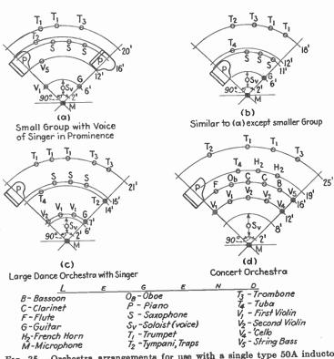
Fig. 35.—Orchestra arrangements for use with a single type 50A inductor microphone.
