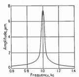
Fig. 23.—Resonance curve of Western Electric telephone.
