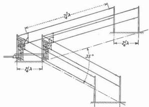
Fig. 40.—RCA model D antenna.
