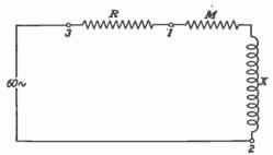
Fig. 12.—Circuit for determining inductance of iron-core coil.
