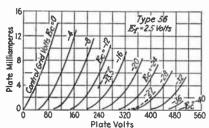
Fig. 9.—Plate characteristics of typical triode tubes.
