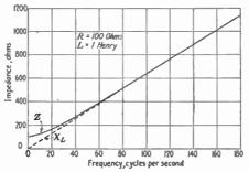
Fig. 6.—Impedance of inductive circuit with frequency.
