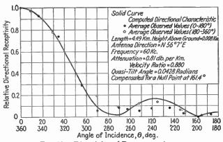
Fig. 50.—Directivity of Beverage antenna.
