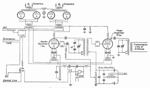
Fig. 5.—Marine coastal transmitter.
