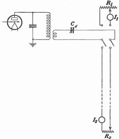
Fig. 69.—Measuring impedance of transmission line.
