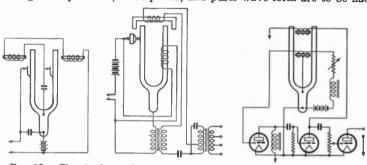
Fig. 25.—Circuits for various types of tuning-fork oscillators (Hummers).
