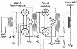
Fig. 54.—Class B push-pull modulator.
