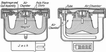
Fig. 11.—Type 618A dynamic microphone. (Western Electric.)
