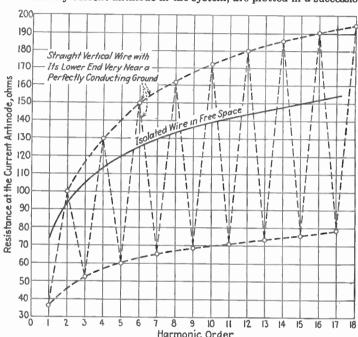
Fig. 6.—Radiation resistances of uniform wires in free space.
