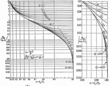
Fig. 6.  $\frac{|Z_0|}{\omega_{rL}}$  vs. n for series circuits.
