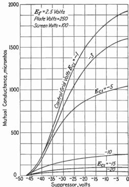
Fig. 31.—Suppressor-grid characteristic, type 58.
