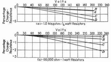
Fig. 4.—Voltage characteristic of various resistors. Curves A are metallised-filament type; others are carbon type.
