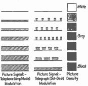
Fig. 9.—Telephonic and telegraphic interpretation of photo densities.
