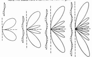
2nd.Harmonic 4th.Harmonic 6th.Harmonic 8th.Harmonic Frg. 14.—Polar diagrams showing radiation from conductor oscillating at several harmonics.
