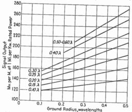
Fig. 24.—Importance of ground system on field strength.
