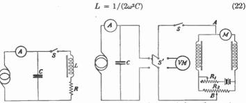
Fig. 13.—Turner constant-impedance method.
