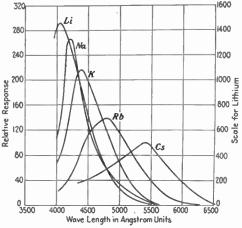
Fig. 1.—Color sensitivity for alkali metals.
