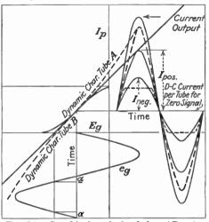
Fig. 34.—Graphical analysis of class AB unit.
