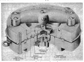
Fig. 27.—Carbon microphone.
