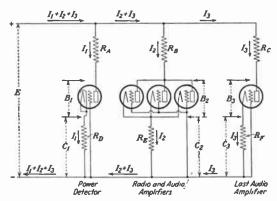
Fig. 3.—Series voltage divider.
