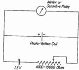
Fig. 11.—Circuit for use with a photovoltaic cell.
