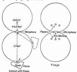
Fig. 36.—Microphone arrangements.
