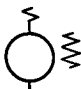
Separately excited D.C. generator or motor with commutating and/or compensating field winding
