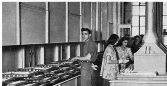
Figure 6-7. Resistors passing through the Enameling furnace where the Vitrohm enamel coating is vitrified.
