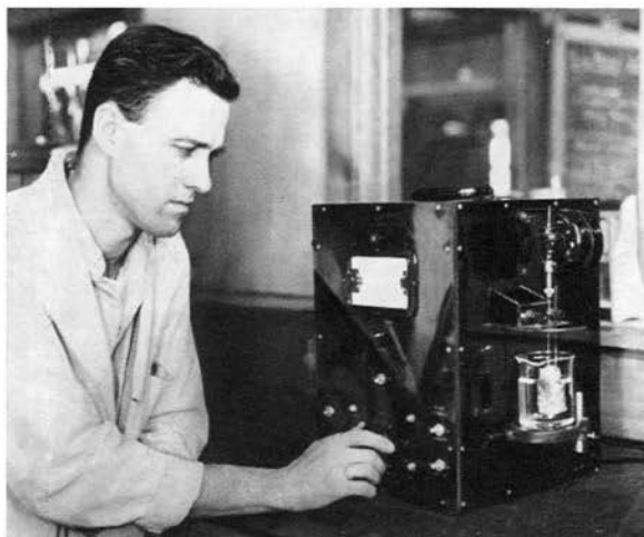
Figure 6-10. Electro-chemical analyzer checks metals and all incoming raw materials for conformity with specifications to insure uniform quality.
