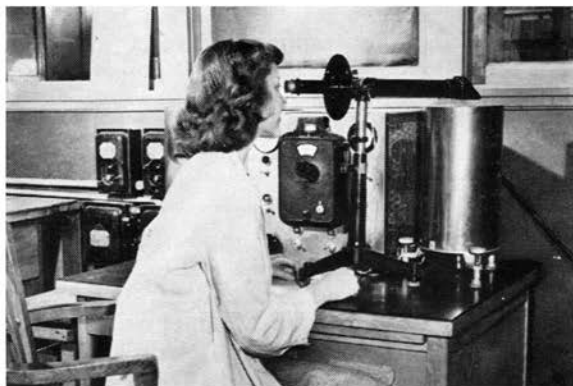
Figure 6-6. Vitreous enamel being measured by interferometer method for coefficient of thermal expansion, melting point and annealing point.*
