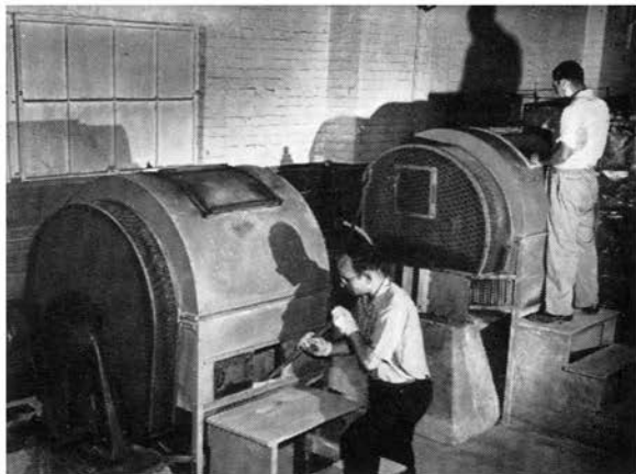
Figure 6-5. These revolving "ball mills" grind the frit to the exact fineness needed to produce perfect Vitrohm (vitreous enamel).
