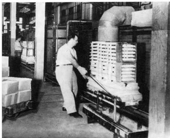
Figure 6-3. Extruded tubes, dried and cut to length, are fired for vitrification in this specially-designed high temperature controlled kiln.
