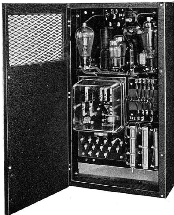
Figure 3-15. Adjustable tubular resistors, lower right, utilizing vertical through-bolt mounting are an essential component of the Electronic Automatic Alternator Voltage Regulator shown.
