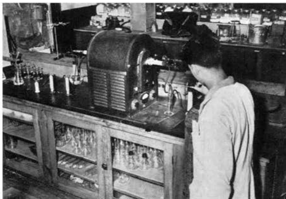
Figure 6-8. A test length of resistance wire is being processed in the combustion furnace to determine carbon and sulphur content and insure accuracy of alloy formula.
