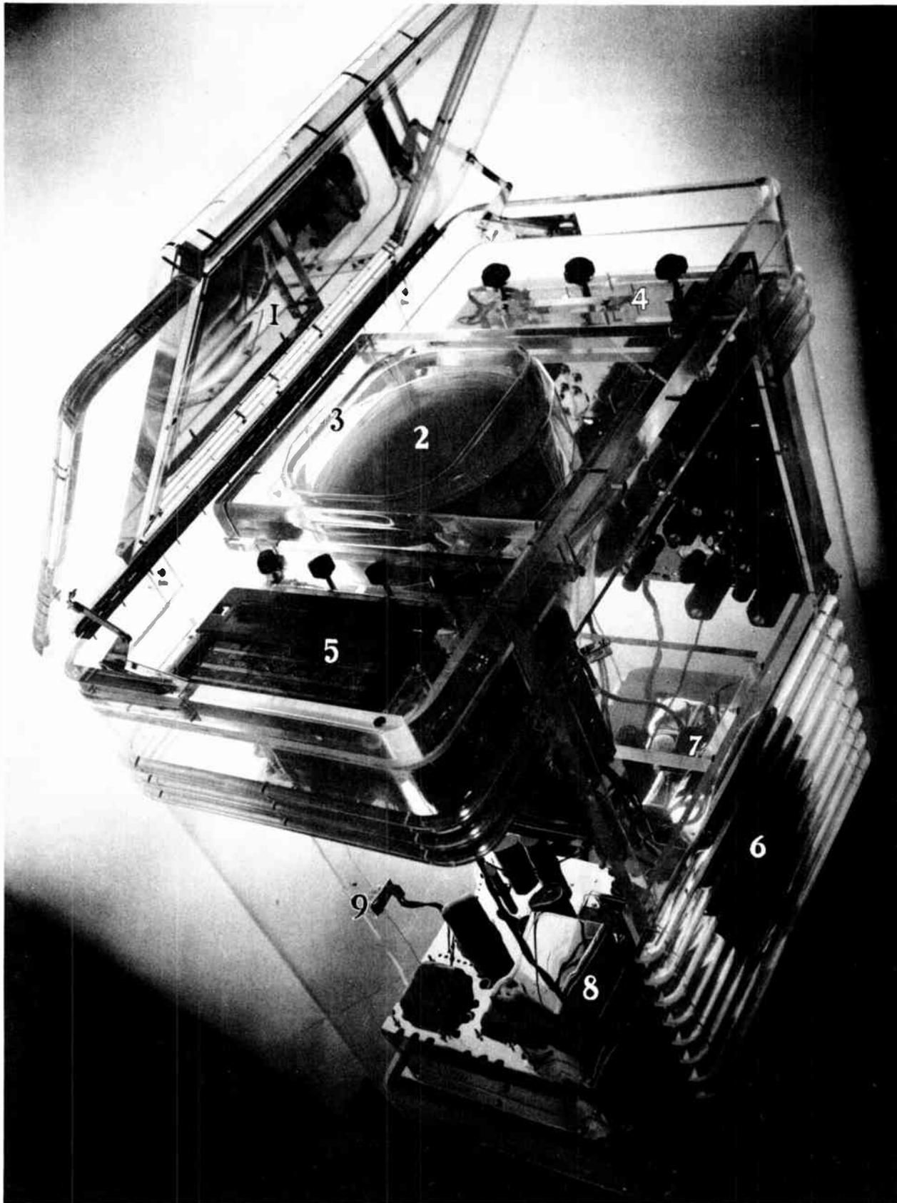
*Inside stuff on a television receiver. (1) Mirror on underside of lid to reflect image; (2) Kinescope picture tube; (3) Frame for picture tube; (4) Television receiving chassis; (5) Radio broadcast receiving chassis; (6) Loudspeaker; (7) and (8) Power supply chassis; (9) Interlocking safety switch to throw off all power when back of cabinet is opened.*
