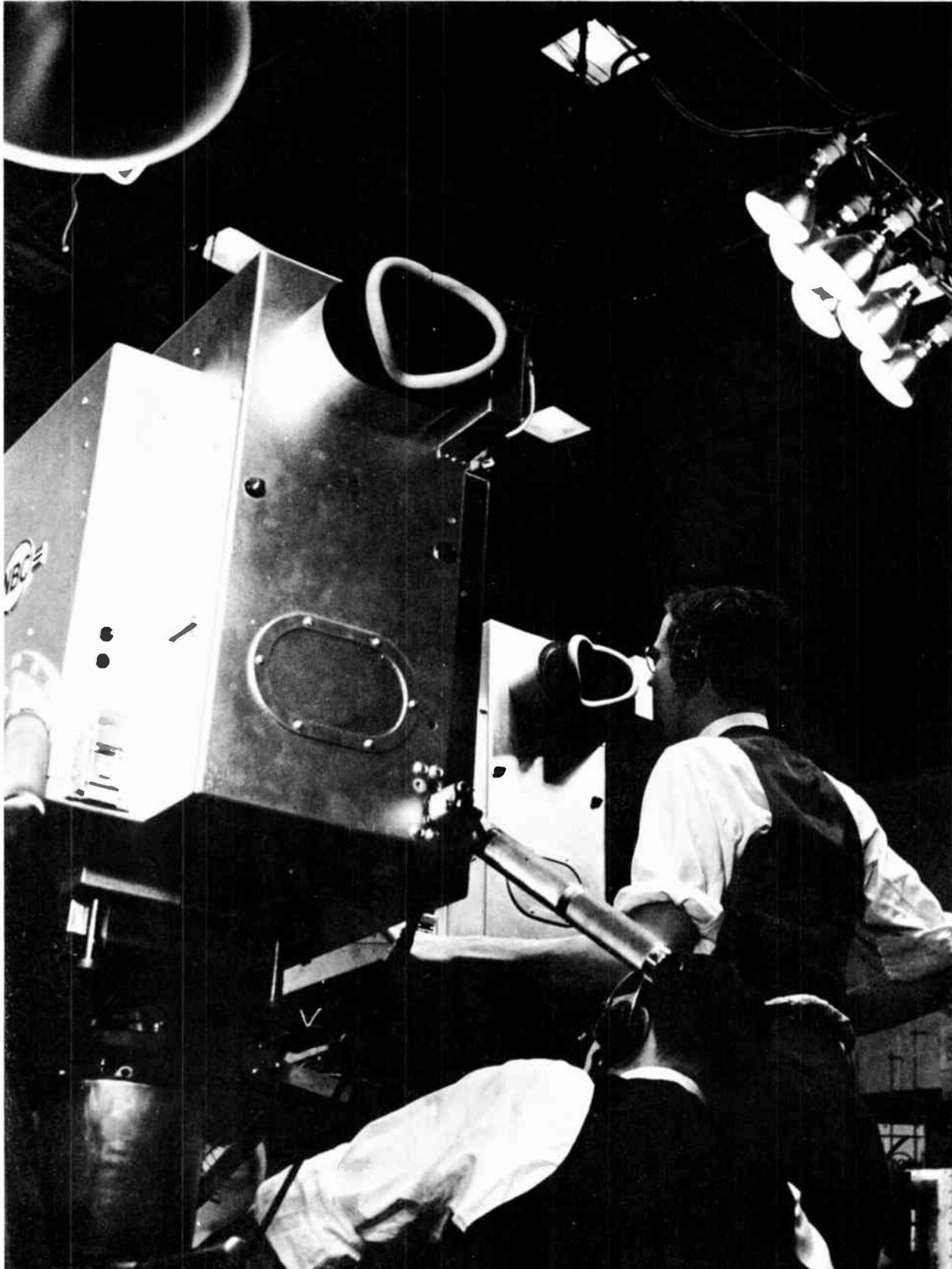
*Behind the television image. Three Iconoscope cameras operate simultaneously in picking up a live talent show. Push buttons in the associated control room make one picture out of the three camera shots.*
