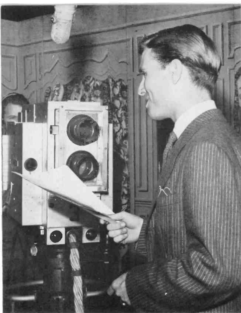
Announcer Ray Forrest in front of early television camera. The upper lens is view finder, the lower is the image-lens. Below lens are two signal cue lights. When green flashes Ray's on the air. When they don't flash, he's off. Overhead is microphone.
