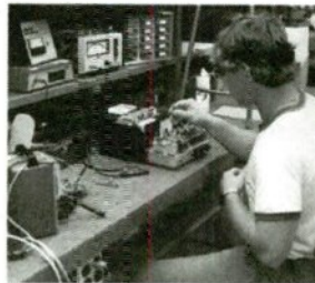
Alignment of circuit modules
