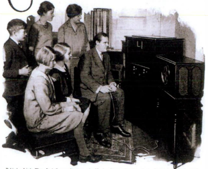
Behind a Little Three-Inch-Square Aperture, the Moving Picture from the Radio Studio Appears. While the Watcher, with a Push Button in His Hand, Keeps the Picture Synchronized
