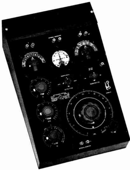
Two popular GR impedance bridges: the modern Type 1650-A and its predecessor, the Type 650-A of 1934.
