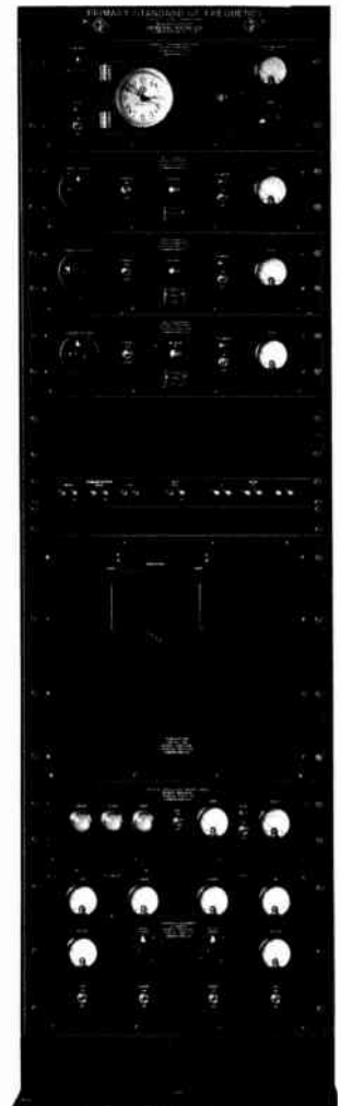
The Type C21H Primary Frequency Standard, introduced in 1928, was the most accurate instrument commercially available for the measurement of frequency and thus soon became the reference standard in laboratories throughout the world.
