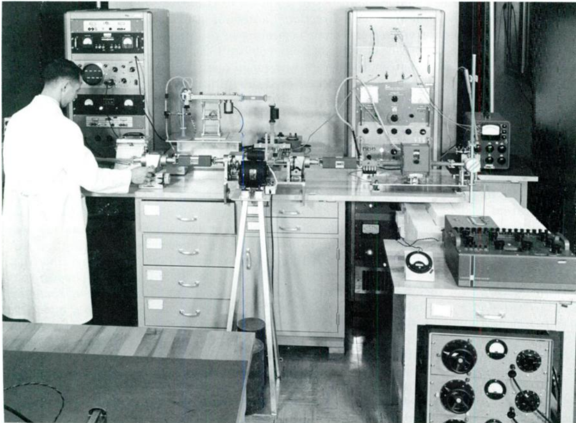
Microwave radiometer in X-band (8.2-10.4 GHz) developed by 1962 to measure the noise temperature of gas-discharge noise sources for use as interlaboratory standards.
