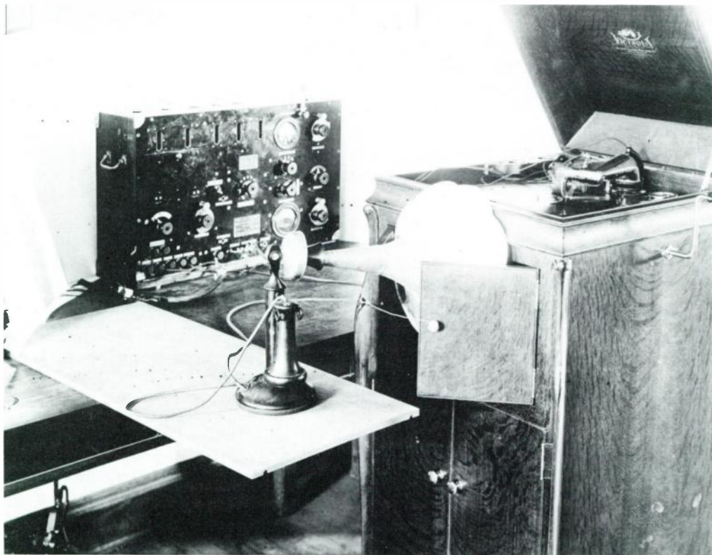
During the spring of 1920 the Radio Section broadcasted music over station WWV in advance of the scheduled commercial broadcasts later in the year. A Victrola phonograph was the source of music, with pickup by a "microphone" using a telephone transmitter fitted with a "morning glory" horn. U.S. Army Signal Corps radio equipment served as the transmitter.
