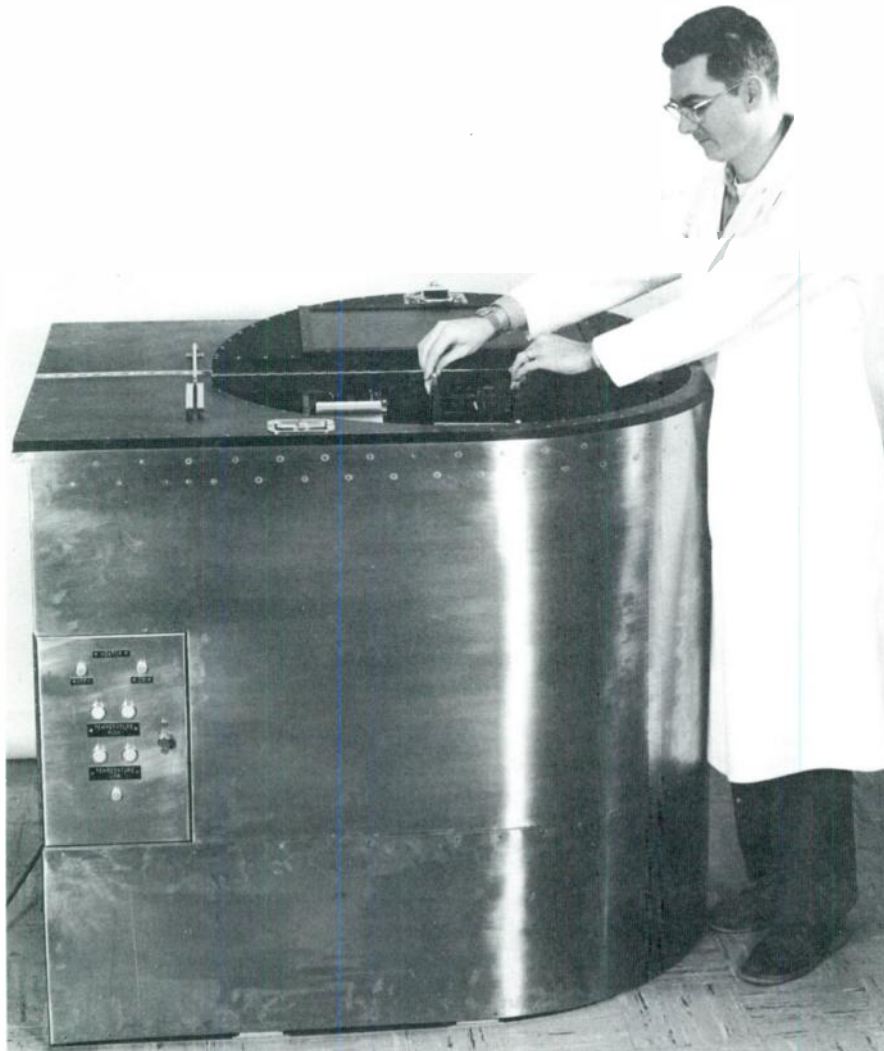
Controlled-temperature oil bath, for saturated standard cells, developed in 1960 by Patrick Lowrie (in photo) of the Electronic Calibration Center. This bath of advanced design combined many novel features for temperature control, ease of handling and circulating the nearly 100 gallons of mineral oil, and easy means of inserting and removing standard cells. Two baths were constructed, one for operation at 28\text{ }^\circ\text{C} , the other at 35\text{ }^\circ\text{C} . Control of oil temperature was within \pm 0.002\text{ }^\circ\text{C} per day. In 1966 the two baths were transferred to the Electricity Division at NBS Gaithersburg.
