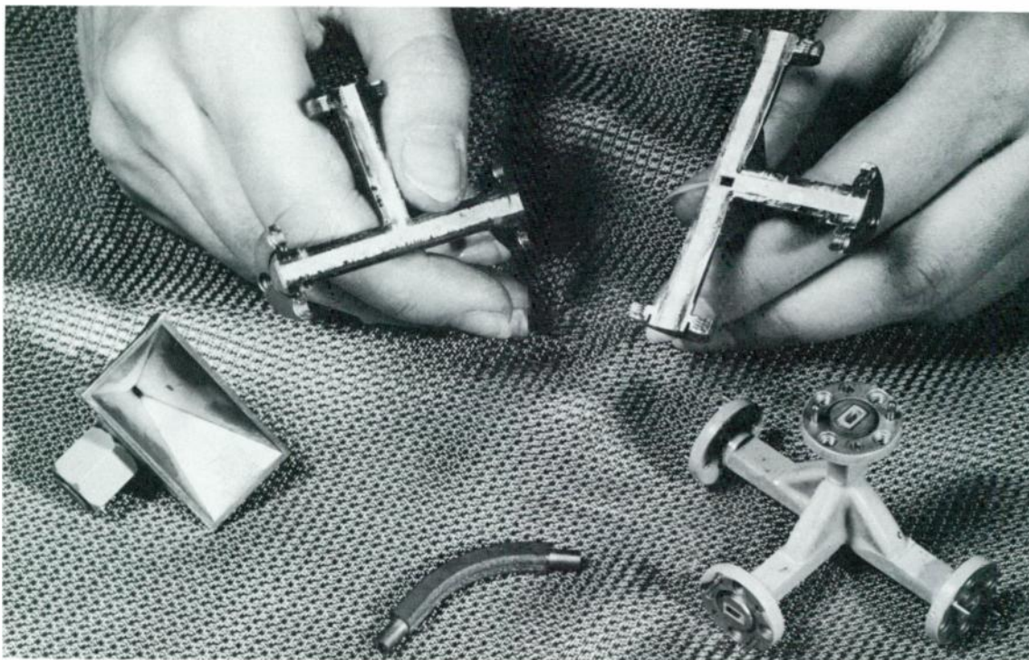
Microwave components in millimeter wavelength sizes electroformed by NBS—connector flanges not electroformed. In foreground cutaway models of hybrid T-junctions in 6-mm wavelength size. Upper left is horn antenna, upper right an E-bend, both in 3-mm wavelength size. Silver was used for electroforming, with added copper layer for increased strength.
