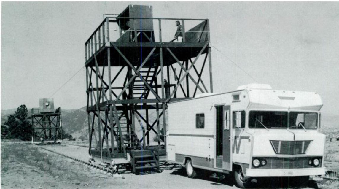
Outdoor 50-meter antenna extrapolation range located at edge of mesa at rear of the Boulder Laboratories site. On-axis antenna gain is measured by using two antennas, each mounted on its own movable tower. Towers can be separated at known distances by moving on accurately aligned rails. Measurements are recorded in the van and a computer analyzes the observations.
