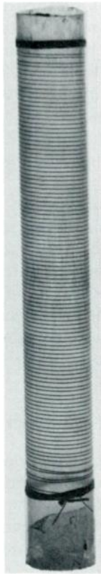
Early form of the electrical hygrometer developed by Dunmore for use on radiosondes to determine relative humidity. Dunmore experimented with this device for more than a decade, bringing about many changes and improvements. In principle, the electric resistance of a film of lithium chloride indicates relative humidity over a wide range. Several patents came from this device and it is used quite extensively today.
