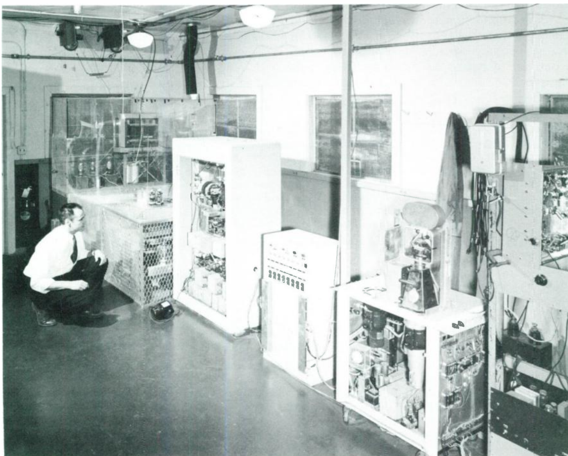
Beginning in 1956, this “one-of-a-kind” ionosonde with a sweep-frequency range of 50 kHz to 2 MHz was used for a number of years for studying the ionosphere at low frequencies. Located at the Sunset field station northwest of Boulder, RF power was radiated efficiently by a very long antenna stretched across Four-mile Canyon and anchored at each end to a mountain top. William S. Hough is shown ready to push a button that started the cycle of operation.
