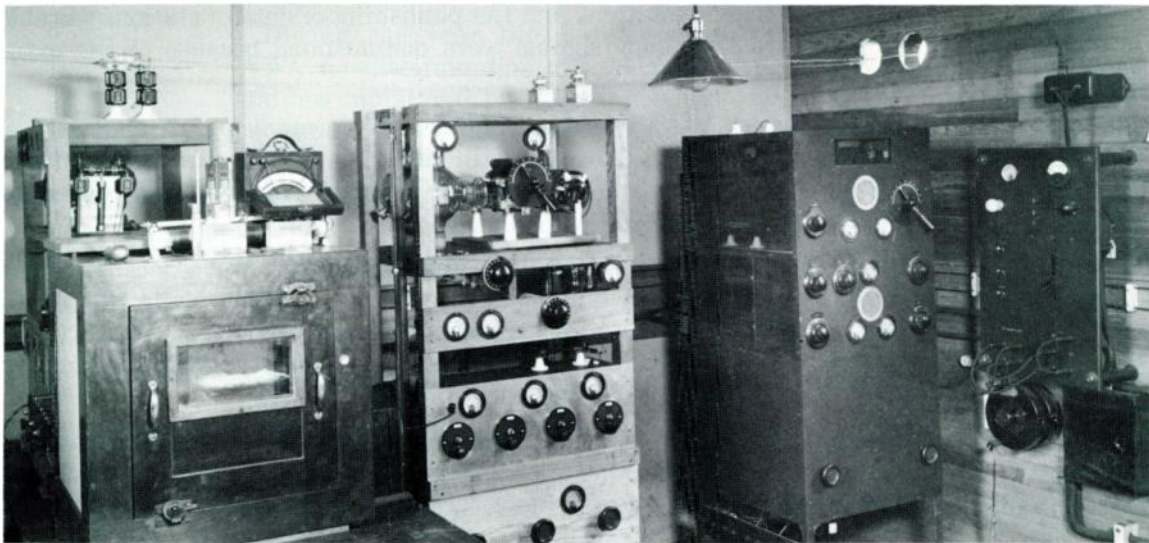
Transmitting equipment of station WWV, College Park, Md. Left front, temperature-controlled cabinet housing 200-kHz control piezo oscillator. Left rear, 150-watt, 5000-kHz transmitter Center, 1-kW 5000-kHz transmitter Right, 1/2-kW multifrequency transmitter Far right, switchboard
