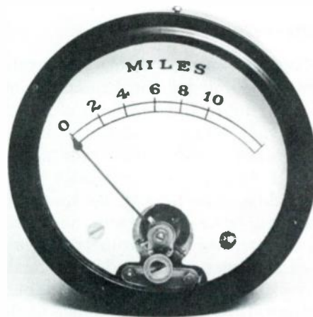
Distance indicator to show approximate distance of plane from runway (actually, distance from the airfield marker beacon transmitter).
