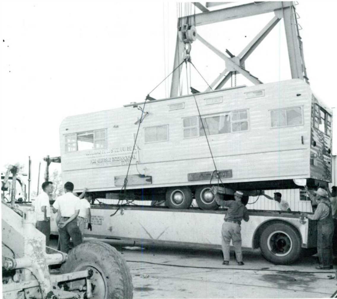
One of four radio receiving mobile laboratories being loaded in August 1955 at the Boulder Laboratories for shipment to South America as a facility in an IGY program to study ionospheric forward scatter across the geomagnetic equator. After test runs in several locations, the trailers were barged down the Mississippi River to New Orleans, then by freighter to South America. Standing, left, by the trailer are Kenneth L. Bowles (left) and Robert S. Cohen, who were in charge of the project. The destination of this trailer was Guayaquil, Ecuador.
