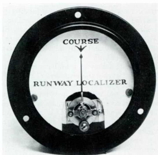
Early pointer-type runway localizer beacon course indicator. A later development of the vibrating-reed indicator, differing only in visual display to pilot.
