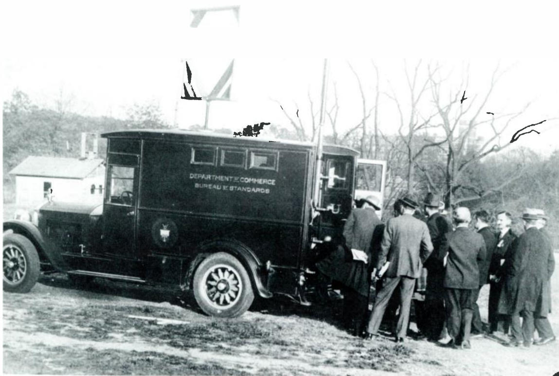
Delegates to International Radio Conference, Washington, D.C. in fall of 1927, inspecting the mobile radio laboratory at the Bureau of Standards. The laboratory truck was used in various parts of the country to make field measurements of fading and intensity of radio signals.
