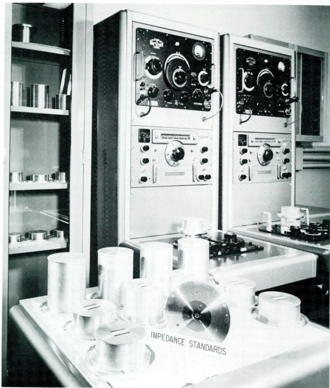
This photograph of 1958 shows 2 of 18 consoles that were being developed in an ambitious project in the Electronic Calibration Center for the calibration of impedance bridges in the frequency range of 30 kHz to 300 MHz. In foreground is assortment of impedance standards of resistance, inductance, and capacitance, shielded in "top hat" enclosures. A specially designed connector made contact with the standard bridge. Passage of time and experience led to a simpler method of calibrating bridges.
