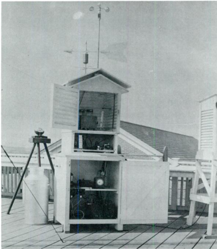
Automatic weather station installed in 1940 at Naval Air Station, Anacostia, District of Columbia. Designed by Diamond and Hinman, the experimental station transmitted radio information on barometric pressure, air temperature, relative humidity, wind speed, wind direction, rainfall, and visibility of the atmosphere.
