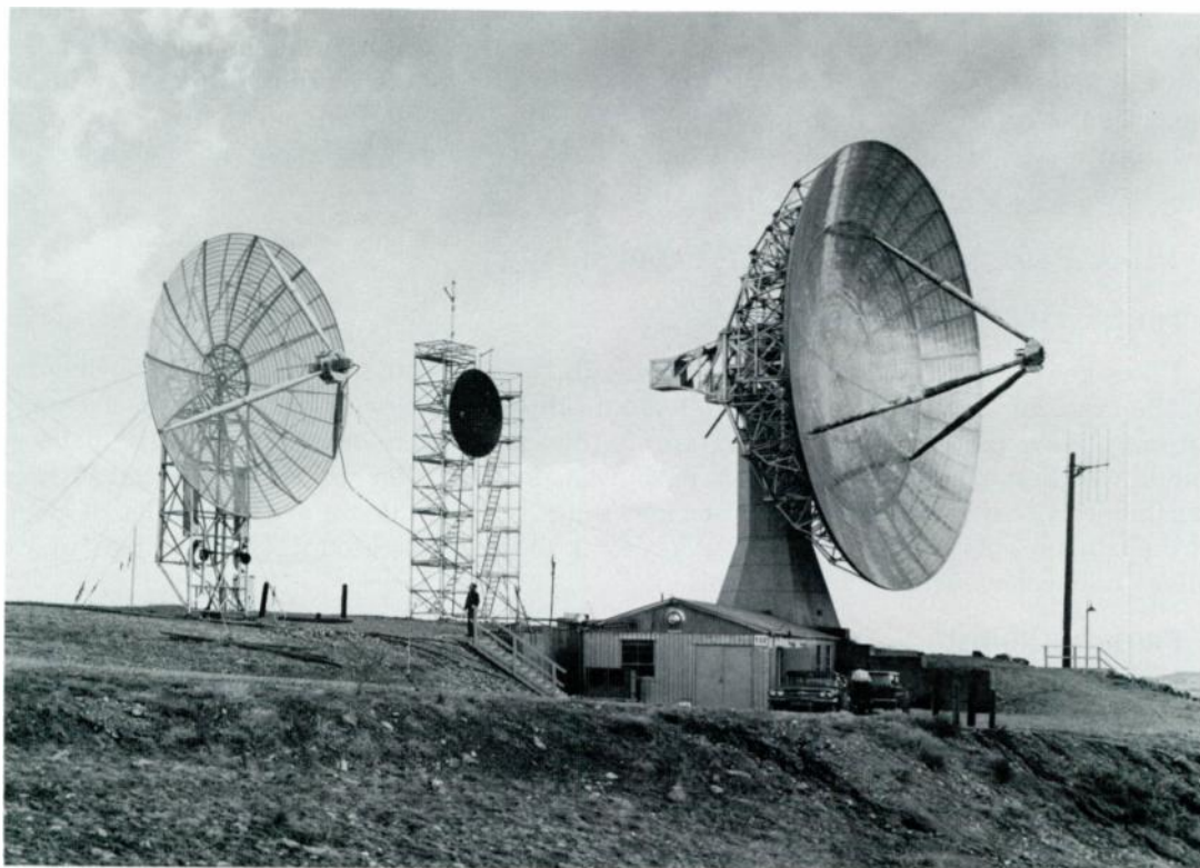
Antenna array at the CRPL Table Mountain field site north of Boulder, including a pair of 60-foot-diameter parabolic antennas. The antennas shown here were located at one corner of the almost level surface of a mesa (approximately 1 mile \times 2 miles) (Table Mountain) which formed the field site.
