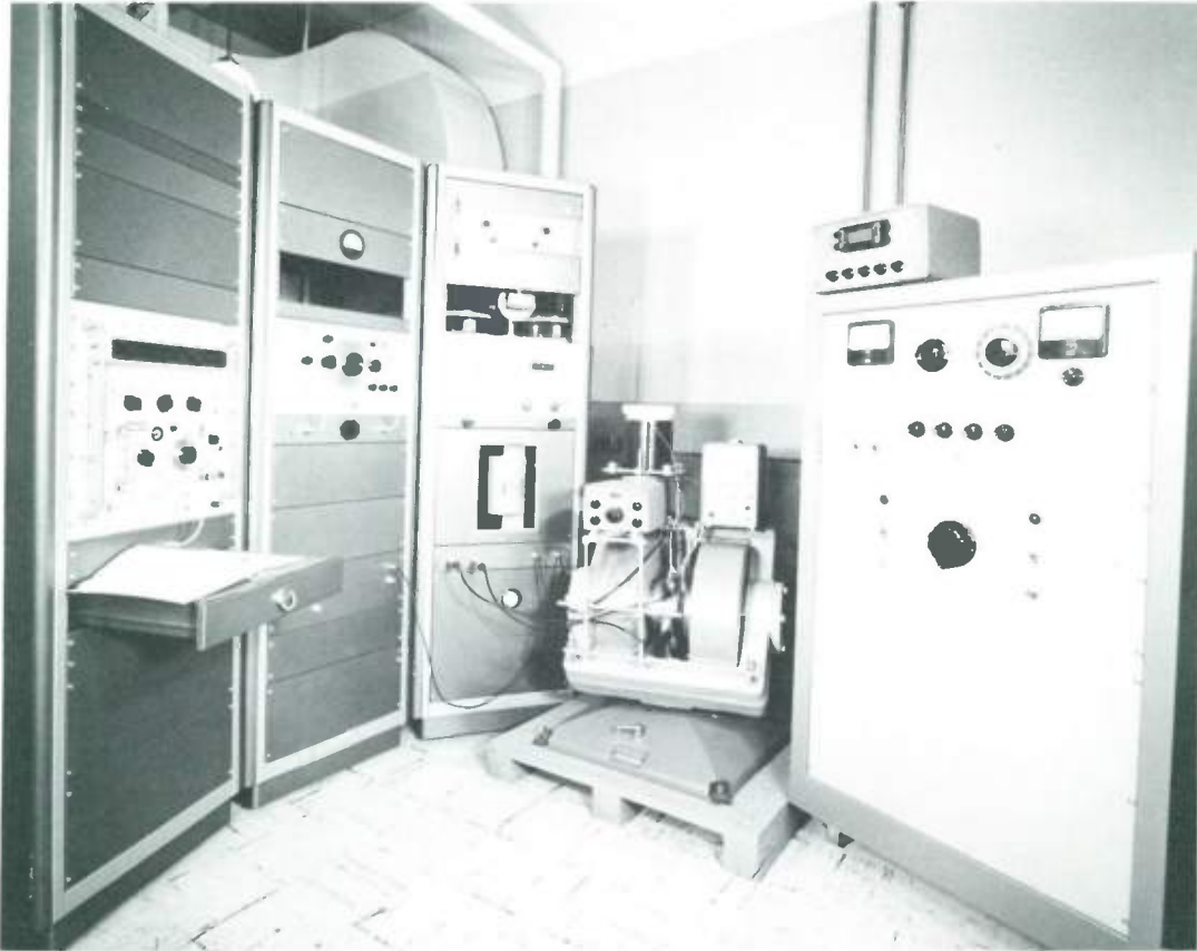
Equipment used in early 1960's for measurement of tensor permeability properties of ferrites at 3100 MHz by the Radio and Microwave Materials Section. The ferrite material was placed in cavity between pole pieces of strong electromagnet (center). Signal generators, detectors, and other electronic equipment are at left. Ferrites have found many uses in RF equipment.
