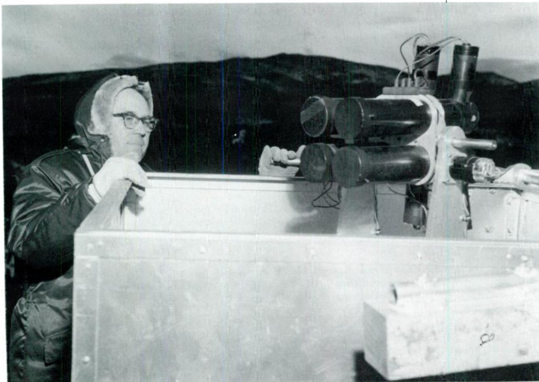
Franklin E. Roach of the Radio Propagation Physics Division views his airglow photometer on a cold day in 1957. Since 1955, observations of the invisible glow in the night sky from large areas of the ionosphere have been recorded on Fritz Peak, several miles south of Rollinsville (west of Boulder) and near the Peak-to-Peak Highway.
