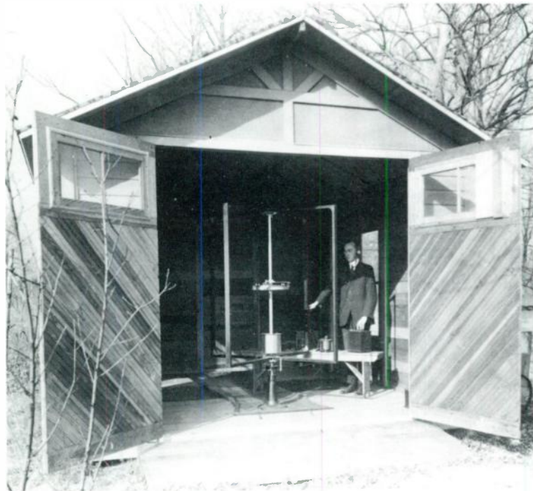
Direction finder at Kensington, Md. field station in 1919, being operated by L. E. Whittemore. A cooperative program (engaged in by L. E. Voorhees) with the Navy revealed large errors in directional bearings caused by the ionosphere. The received signals were from transmissions of long wavelengths (e.g., 13,600 meters, or 22 kHz).
