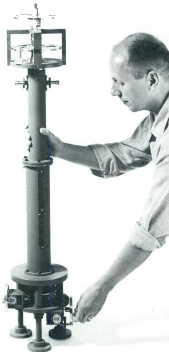
In 1962 Alvin Rasmussen, Radio and Microwave Materials Section, examines a re-entrant cavity (250-950 MHz) used for measuring complex permittivity of dielectric samples. Two wheels at top change and measure separation of capacitor plates between which sample is inserted. Mechanism at bottom tunes cavity to desired frequency. Measurement reveals characteristics and suitability of dielectrics for RF equipment.
