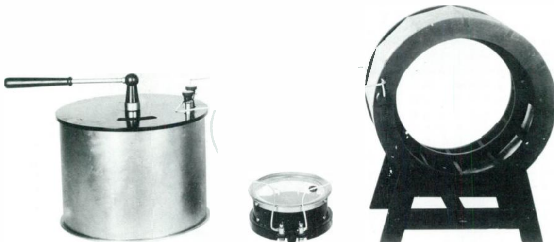
Very early wavemeter developed by Radio Section. This photograph was published in NBS Circular 74, "Radio Instruments and Measurements" (issued March 23, 1918), with the title "Standard wave meter circuit." Wavelengths over the range of 100 to 13,000 meters were calculated from low frequency calibrations of several capacitors and inductors, taking into account the high frequency effects of leads, distributed capacity of inductors, and losses in capacitors. Resonance was indicated by current flow in loosely-coupled, single-turn loop and thermal ammeter.
