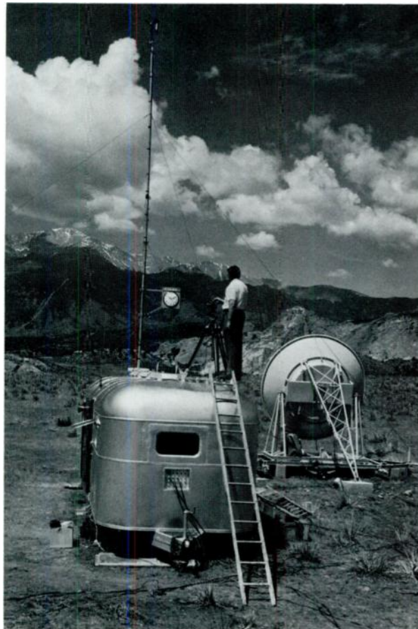
Portable radio receiving antenna (right) and meteorological and photographic equipment (in and atop the van), as used in line-of-sight experiments between Pikes Peak and Garden of the Gods, Colorado Springs, Colo. The equipment was part of a study of the effects of atmospheric turbulence on the stability of the electrical length of a radio path.
