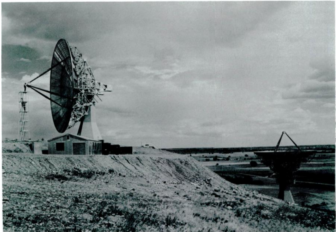
Two 60-foot-diameter parabolic antennas at the NBS Table Mountain field site, north of Boulder. Differences in azimuth and elevation allowed measurement of phase differences (and differences of electrical length) in the arrival of radio waves. The antennas could be moved 90° in elevation between the vertical position (left) and the horizontal (right), and could be rotated 360° in azimuth.
