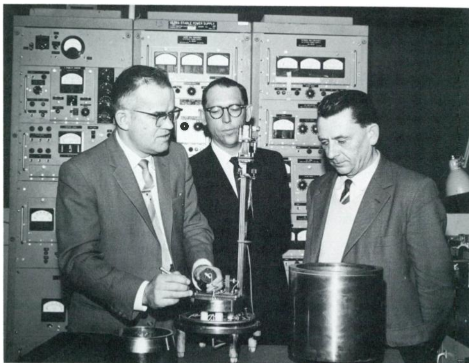
Glenn Engen (left) explains the features of advanced model of microwave microcalorimeter to Dr. Schaffeld (right) of the Physikalisch Technische Bundesanstalt (counterpart of NBS, Western Germany). At rear, George Schafer, chief of the Radio Standards Engineering Division. Engen improved upon the design of Macpherson and Kerns to obtain much greater accuracy of microwave power measurement. Klystron power supply at rear was one of three specially designed by manufacturer for NBS use. Photographed February 1963.
