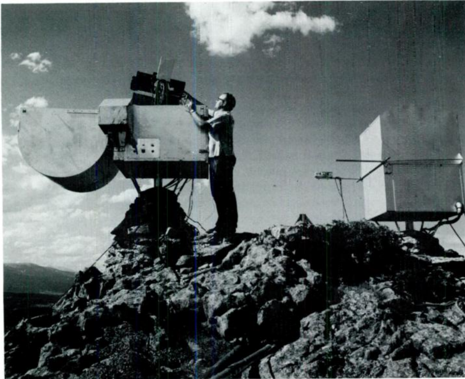
Lawrence R. Megill adjusting controls of the automatic airglow photometer mounted on top of Fritz Peak. The metal housing protects the photometer and remains open only for nighttime recordings of airglow. A closeup view of a long stretch of the Continental Divide can be had from Fritz Peak (elevation 9010 ft). On the date this photo was taken, October 2, 1957, the aspens would be in full autumnal foliage, mottling the nearby landscapes with a golden glow.
