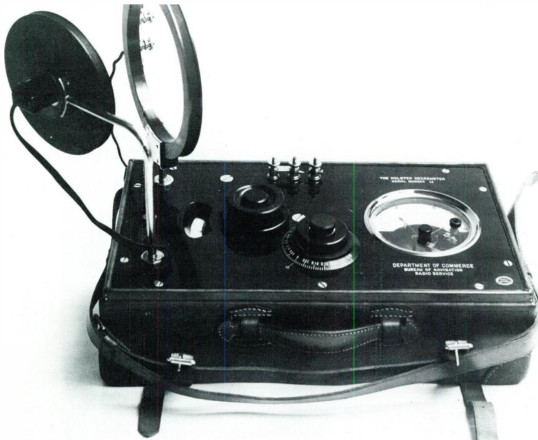
An early form (1912) of a series of direct-reading decremeters designed by Kolster. Among the users of these instruments were the radio inspectors of the Bureau of Navigation, Department of Commerce. The instrument provided a test that determined the degree of interference caused by damped oscillations of spark transmitters.
