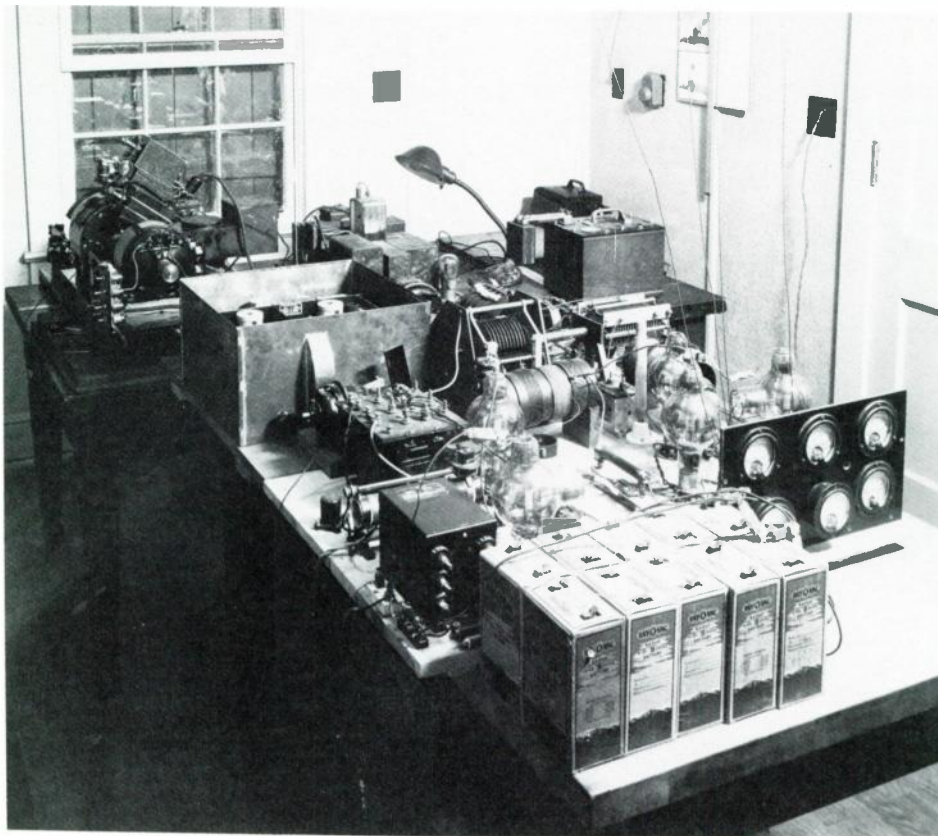
Radio transmitter (front) and receiver with recorder (rear) for automatic recording of virtual heights of ionosphere. This first automatic multifrequency recorder (or ionosonde), with a frequency range of 2500 to 4400 kHz, was developed by Gilliland in 1932 and installed in Building No. 3 at the Beltsville, Md. field station, and later moved to the Meadows, Md. field station.
