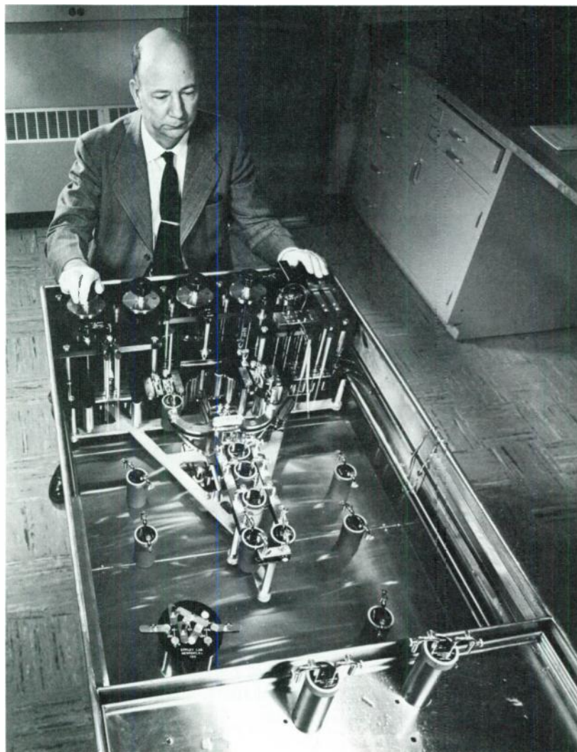
Photograph (1958) of Frank Weaver, head of Low Frequency Unit, Electronic Calibration Center, operating precision bridge used to calibrate standard resistors with uncertainty of less than one part per million. The bridge was a development in 1918 by Dr. Frank Wenner of the Electricity Division, and a small number have been manufactured through the years. Originally called the NBS Precision Bridge, it became better known as the Wenner Bridge. All parts of bridge, except control knobs, are submerged in oil at constant temperature of 25 °C.
