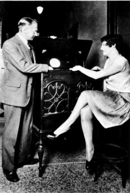
*Dr. Vladimir K. Zworykin demonstrates an early cabinet TV receiver, based on the cathode ray system that he invented and that laid the groundwork for all-electronic television.*
