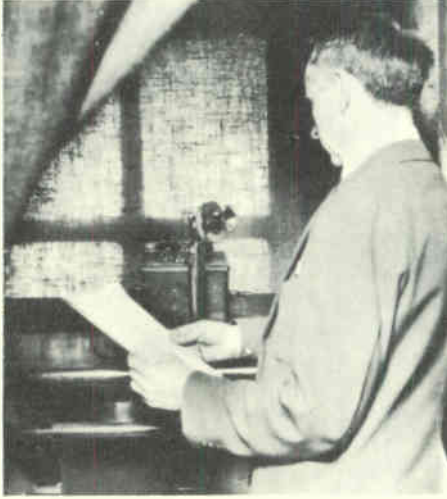
In 1920 an ordinary telephone served as microphone for the first USDA broadcasts of market news over government-owned stations.
