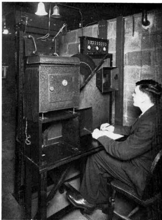
An early television 'studio'. A Nipkow scanning disc can be seen just below, and to the left of, the panel with three meters on it.
