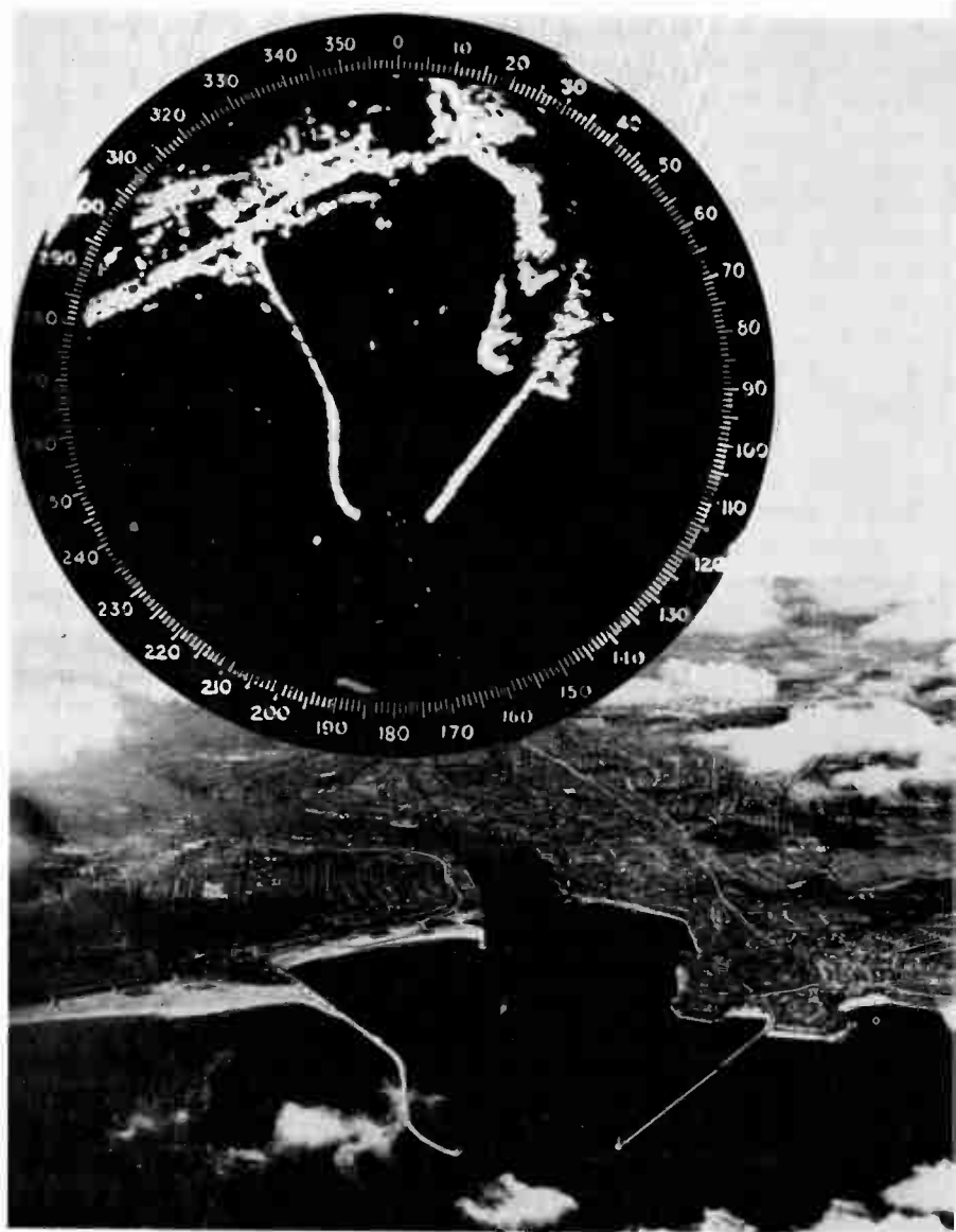
A harbour entrance and its image on a radar screen.
