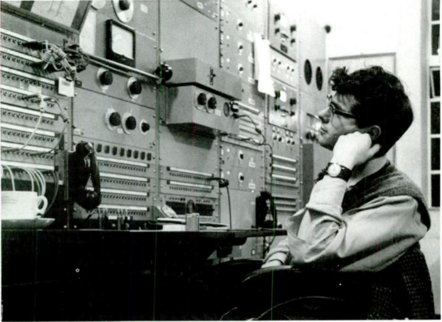
Figure 14.4 The control position at the Woofferton VOA relay station in the 1960s. Note the old-fashioned jackfields and the old-type drop-flap telephone indicators
