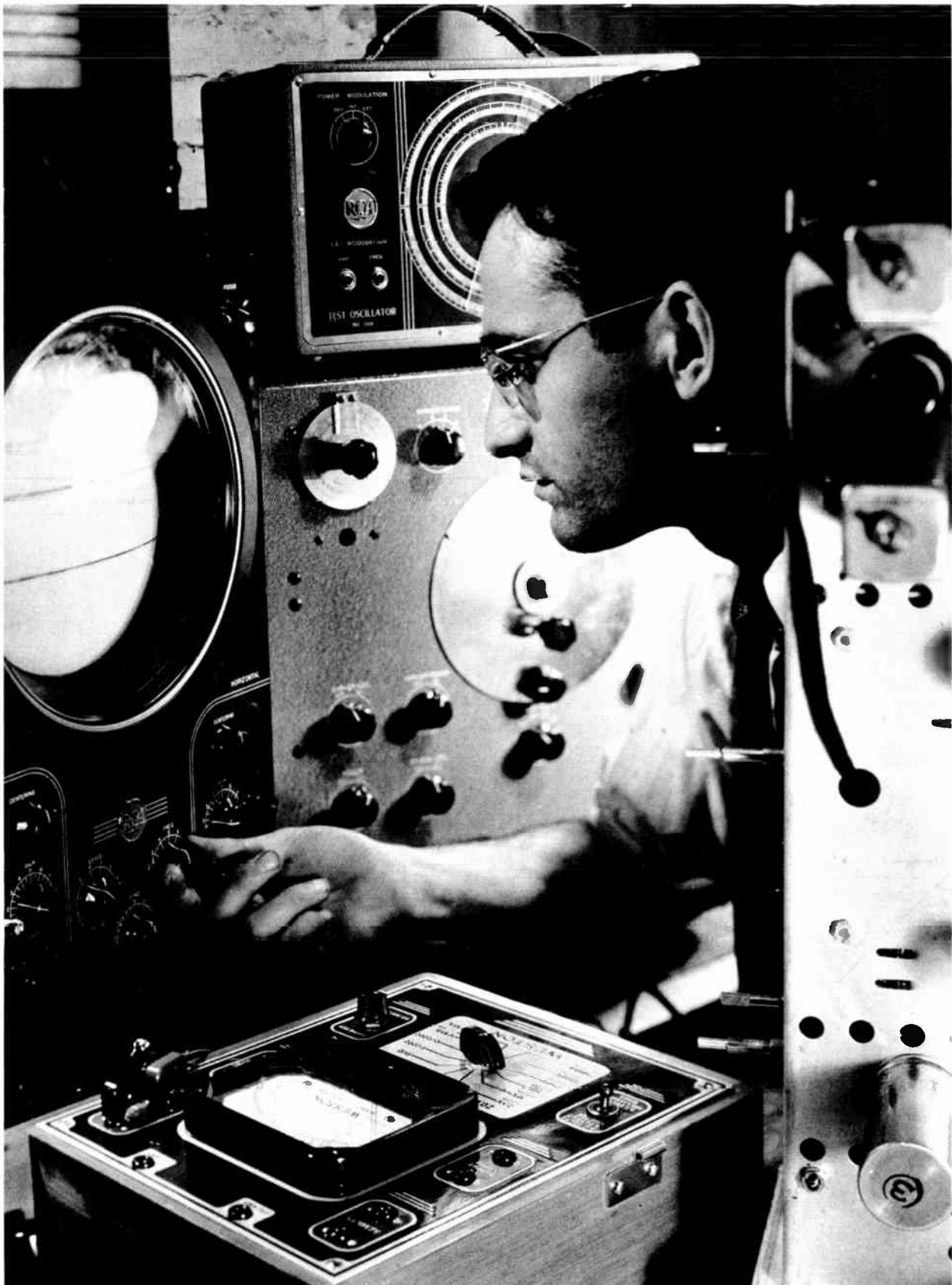
Testing television. Checking on receiver's efficiency by means of test oscillator and large cathode ray oscillograph.
