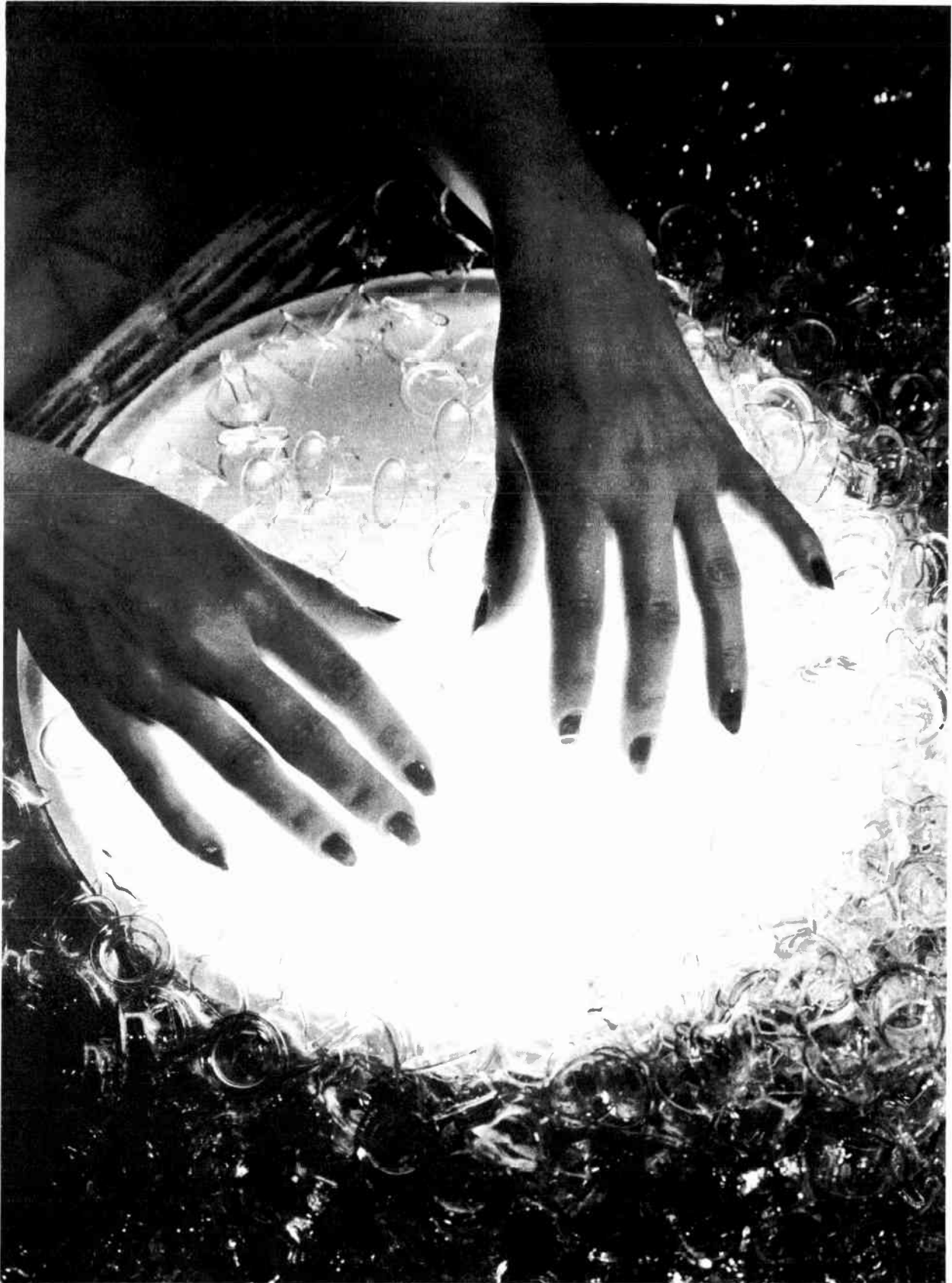
Not bubbles—but glass. The girl behind those perfect hands is testing radio tubes for imperfections in the glass.
