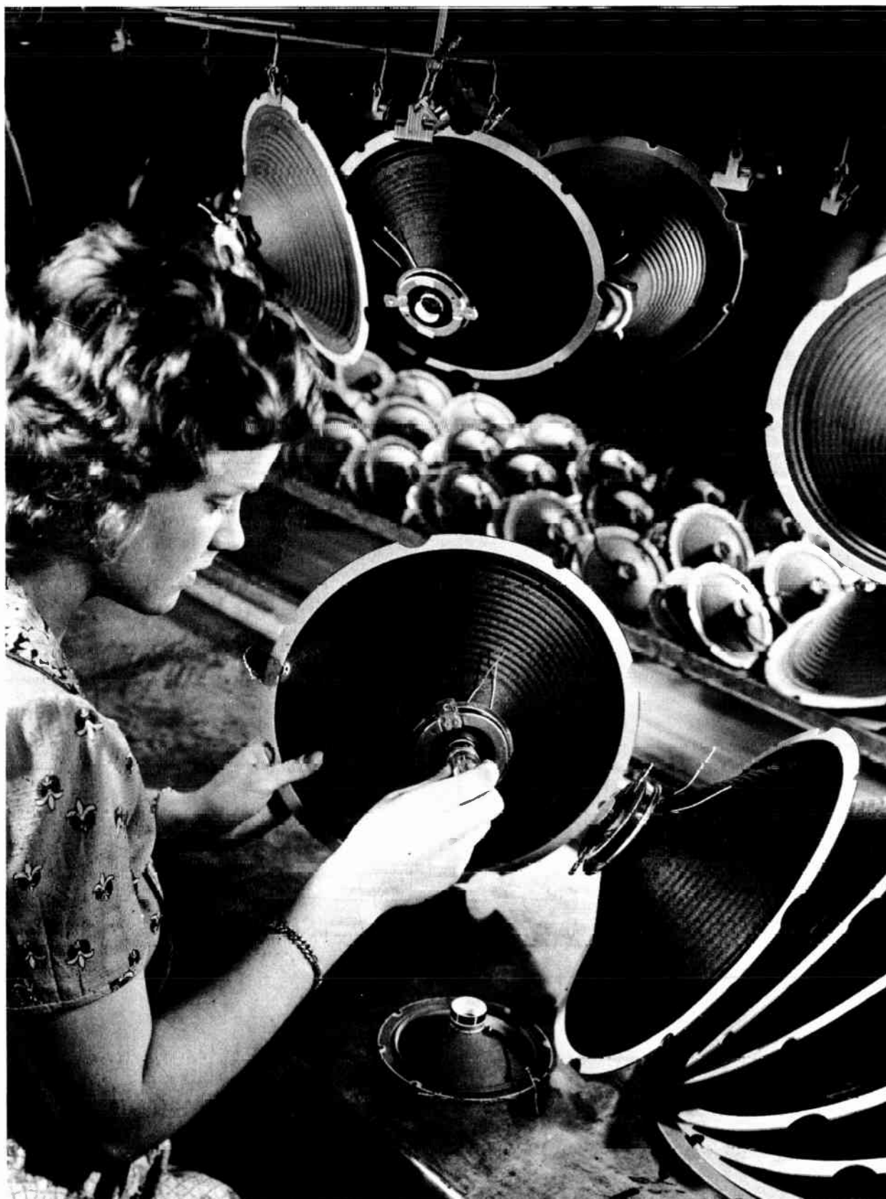
Loud speaker cone manufacture. Checking voice coil to make sure that it is within necessary close tolerances as to size and roundness.
