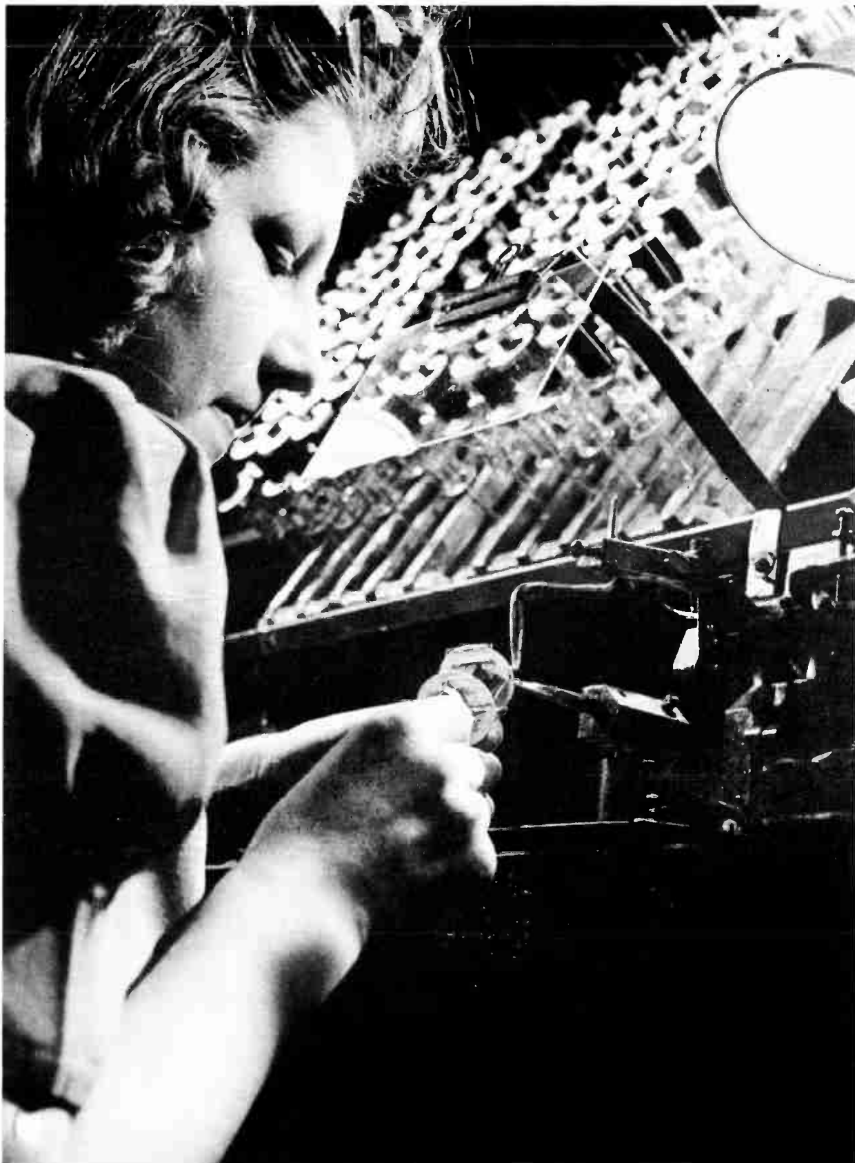
Assembling the mounts of beam power transmitting tubes. Parts are assembled on a jig which aligns and spaces them while they are spot-welded together.
