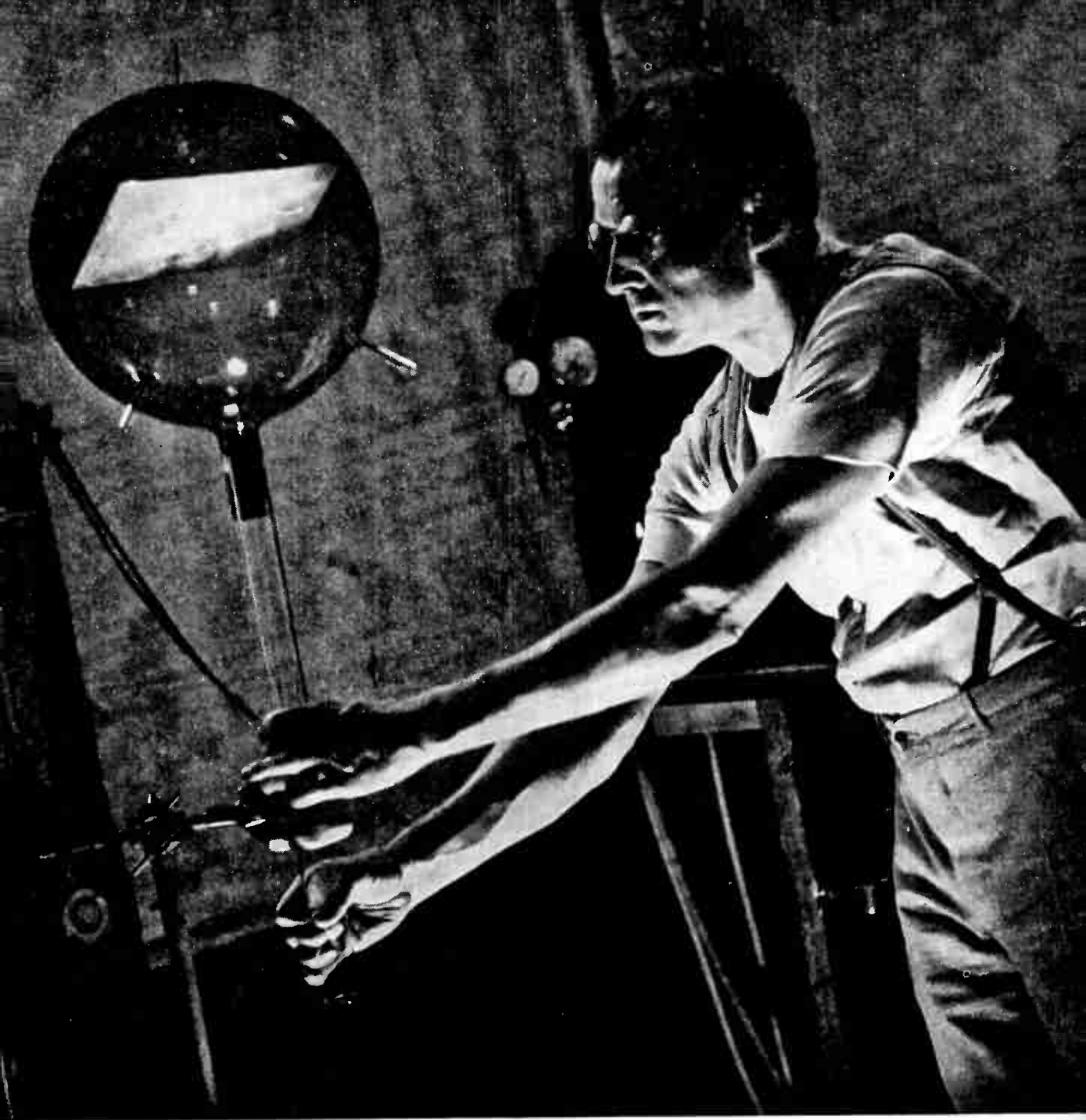
Above, an "iconoscope" tube in an early stage. This tube is the "eye" of the television camera
