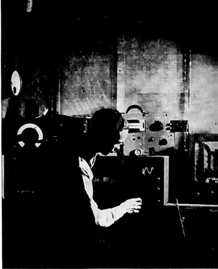
Engineers check up the tonal qualities of a radio receiver and make sound visual on this oscilloscope for close study
