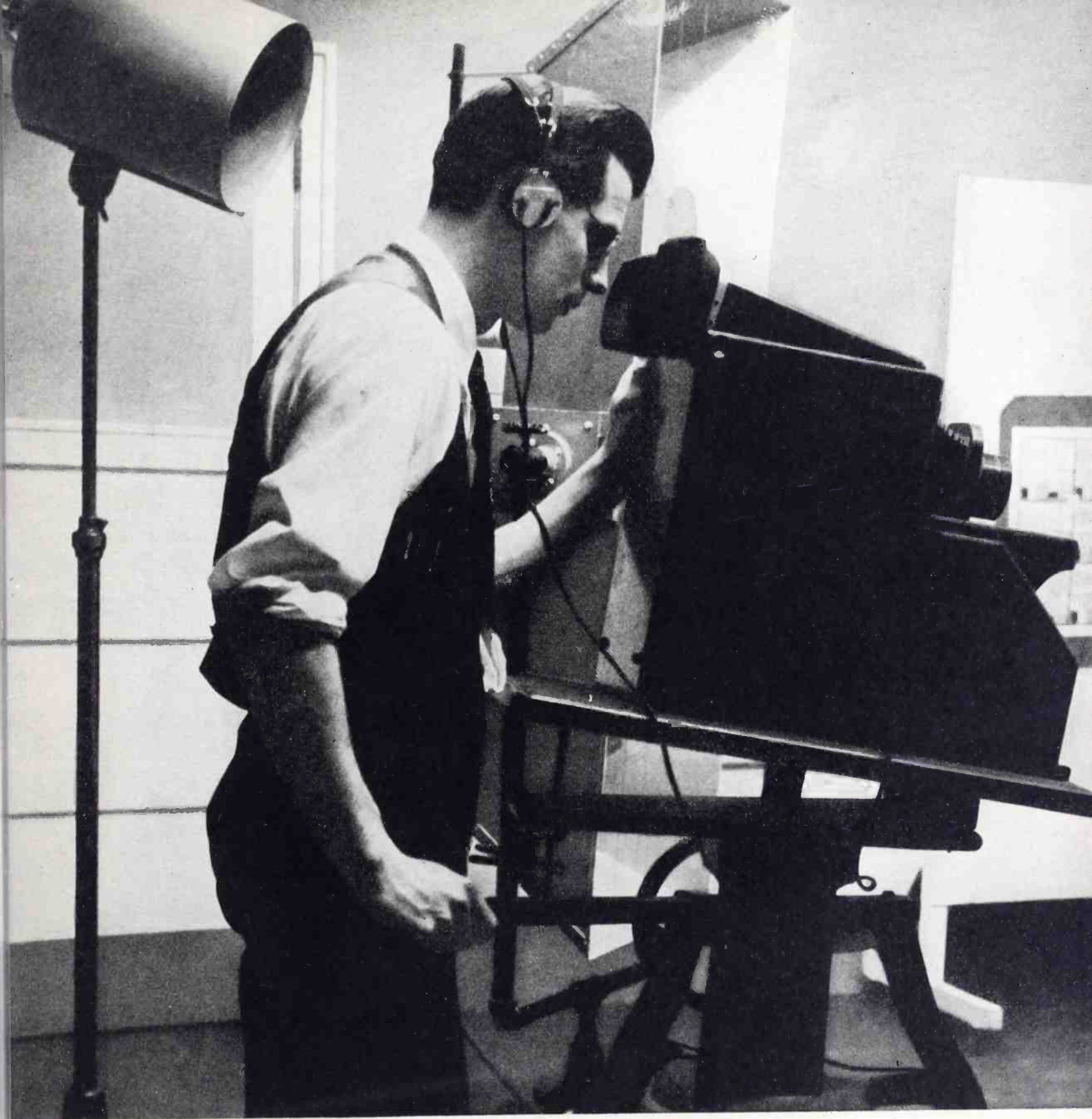
Laboratory model of the television camera. The iconoscope tube is contained in the compartment
