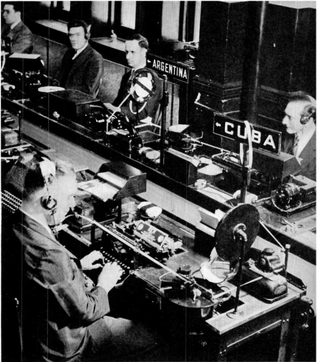
The operator in the foreground is transcribing the wavy line on a receiving tape into the words of a message
