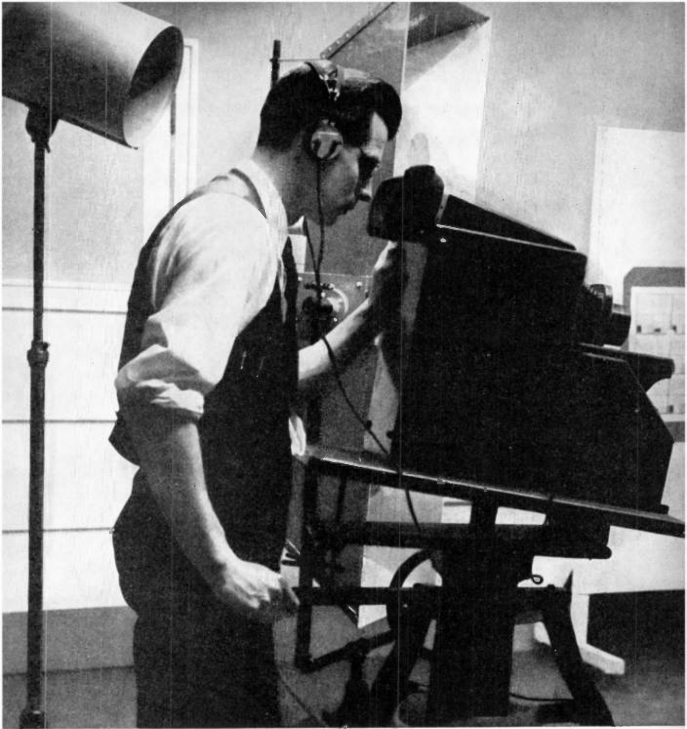
Laboratory model of the television camera. The iconoscope tube is contained in the compartment
