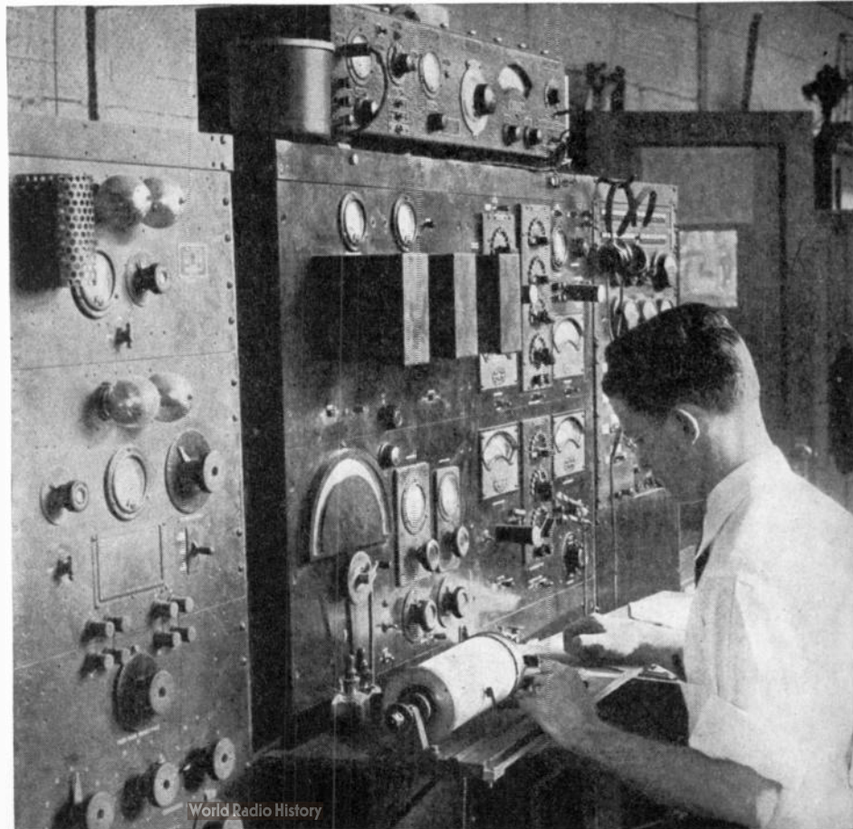
Measuring acoustic characteristics of radio receivers
