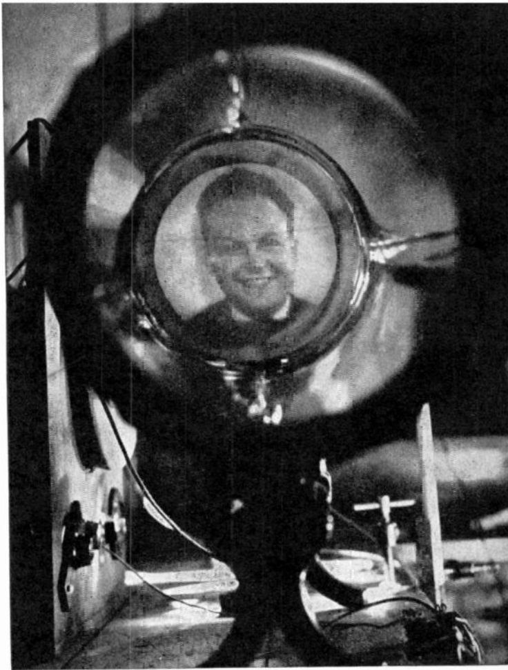
The television image tube is here shown reproducing a picture invisible to the eye
