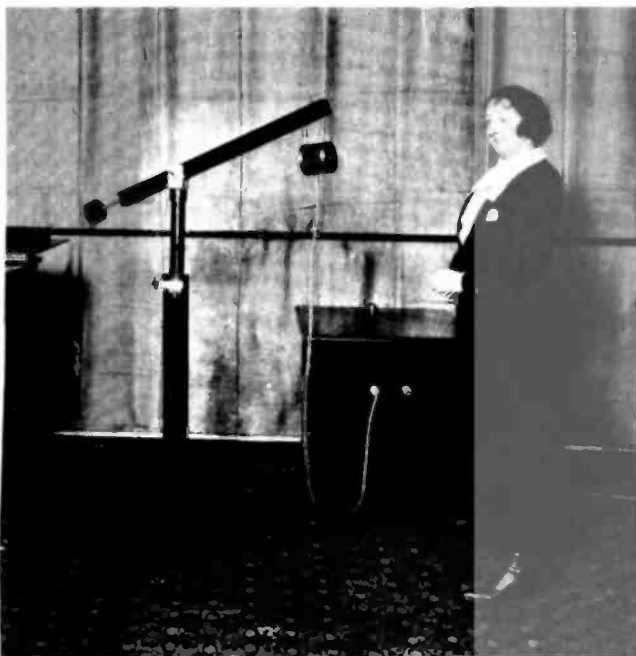
This 1921 picture shows an early microphone with a boom arrangement that permitted it to be raised or lowered according to the performer's height.
