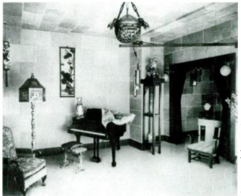
KMED's Sparta Building studios featured elegant Chinese decor. The technical plant was similarly grand. Note the traveling boom-mounted condenser microphone, which could easily be adjusted to pick up performance groups of different size. A condenser microphone was state-of-the-art and not frequently found in smaller-market stations in 1931, the approximate date of this photo.
