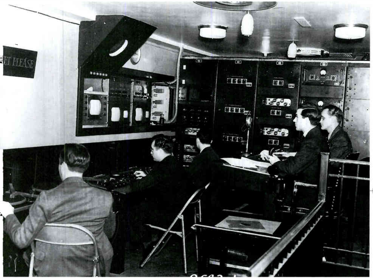
T he control room at NBC's 4H. The director and technical director could not see the studio floor, only the the preview monitor. Keys to the studio were fiercely guarded, and technicians were sworn to secrecy. (COURTESY GLOBE PHOTOS)
