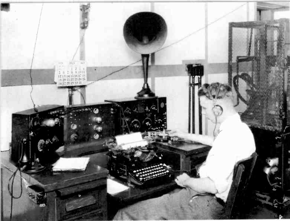
Shortwave and longwave receiving sets at the Westinghouse Telegraph transmitter control at WBZ in Springfield, Massachusetts.
