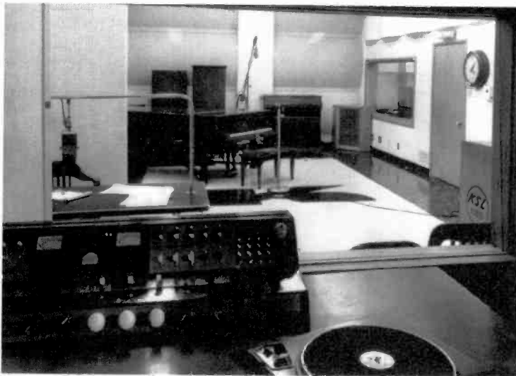
This KSL, Salt Lake City, studio was typical for local 1940s radio stations, which included a control console, turntable for transcripts of shows to be played, a studio piano and organ.
