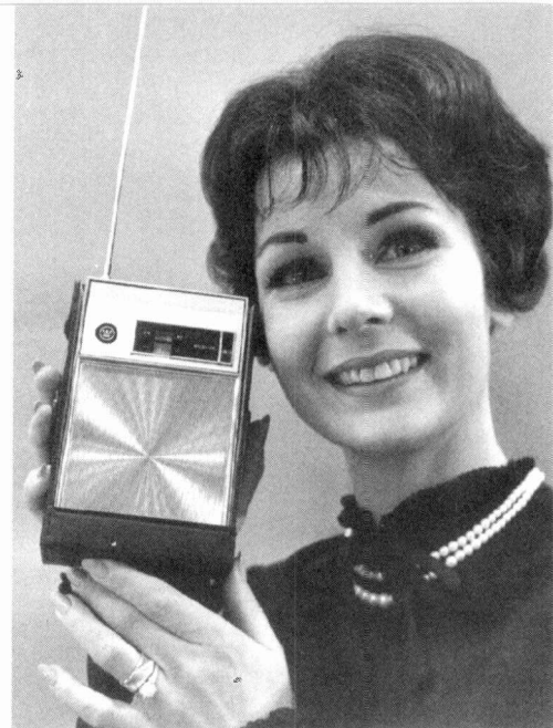
Wow! Nine transistors! This portable AM/FM radio was placed on the market in January 1963. It was said this Westinghouse radio would play 100 hours on four penlight batteries.
