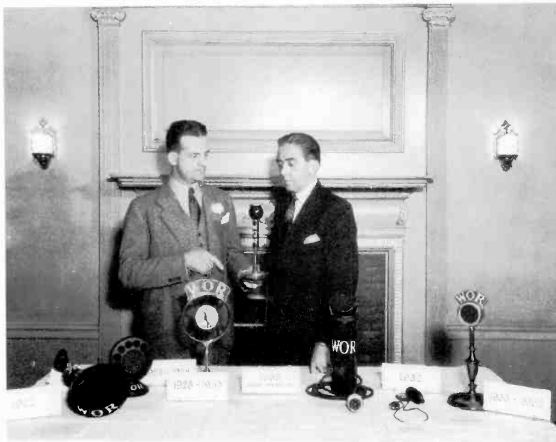
J.R. Popele, WOR's chief engineer, showing Alfred J. McCosker, then-president of WOR, the new dynamic mic, the latest in microphones in 1935. Displayed is an evolution of WOR microphones: (l-r) Telephone transmitter with megaphone (1922), Double Carbon Button (1923-1928), Improved Double Carbon and mounting (1928-1933), Condenser Mic with amp (1928-1933), Lapel mic (1932) and the dynamic (1933-1935).
